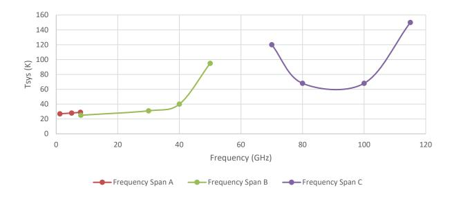
Figure 3 – T<sub>SYS</sub> over frequency in precision environment.
