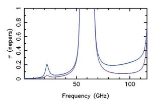
Figure 4 - Atmospheric temperature and opacity for wet (blue) and dry (purple) conditions. [RDII]
