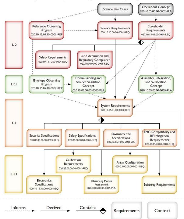
Figure I – Requirements flow-down to the ngVLA System Requirements.
