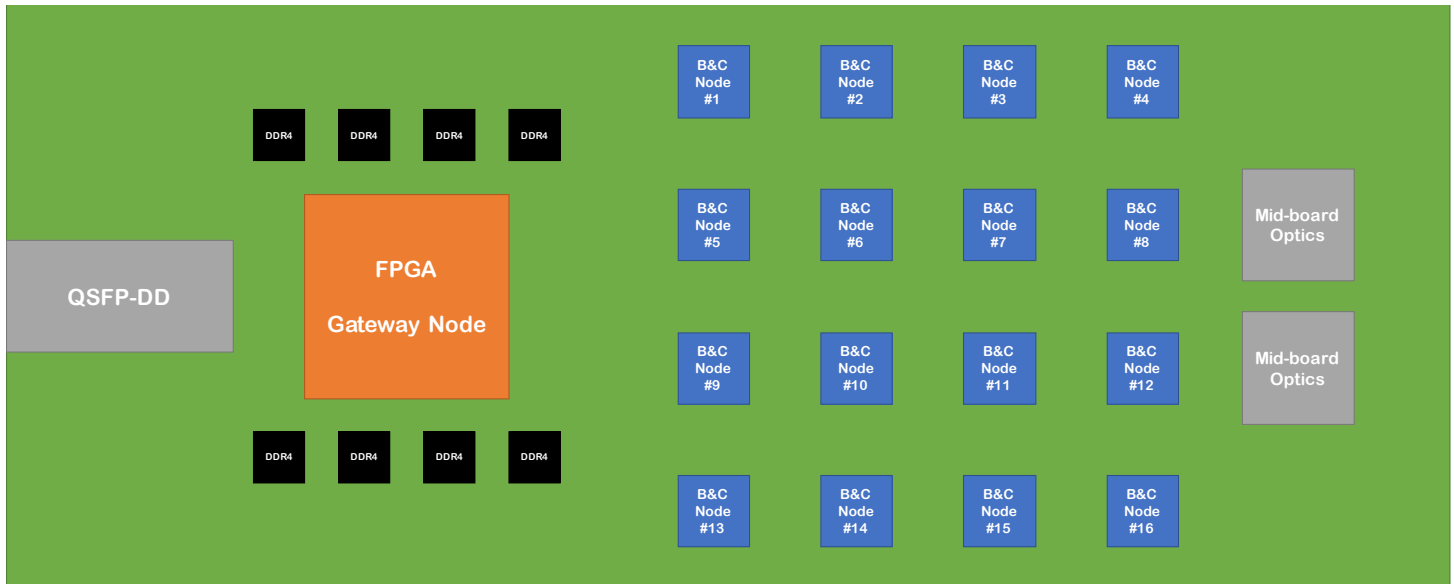
Figure 24: Preliminary B&C board layout featuring 16 nodes per board and other main processing and data communications components. Two boards would fit into a 19-inch enclosure constituting a B&C LRU.
