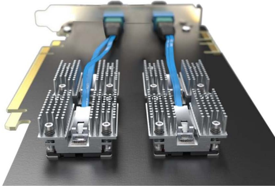
Figure 14: An On-Board Transceiver system is used to interconnect each SBP unit’s FPGA to one another through a passive optical mesh. Taken from fibersystems.com . Credit: Amphenol FSI.
