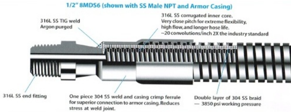
Figure 1 - Armored flex-line cross section view.
