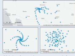
Main interferometric array composed of a compact core (bottom right; short baseline array antennas are shown in green), a five arm spiral spanning the Plains of San Agustin (bottom left) and a nearly 3-armed spiral that extends into TX, northern Mexico and AZ (top).
