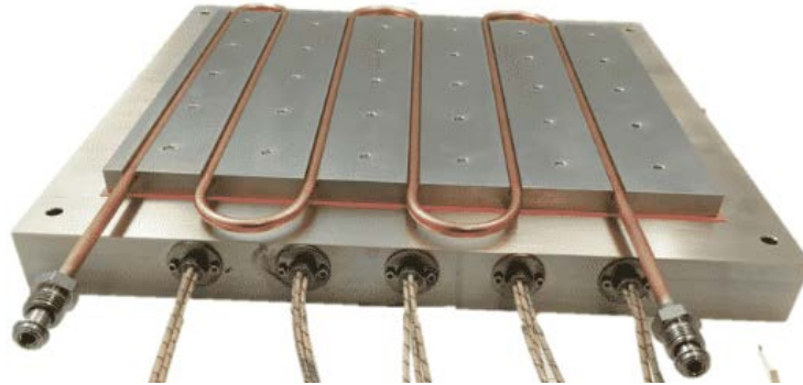
Figure 7. Example of a liquid cold plate on sample electronics
