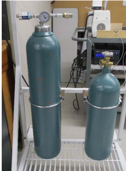
Figure 17: Picture of the buffer tank on the left and the helium charge cylinder on the right.
