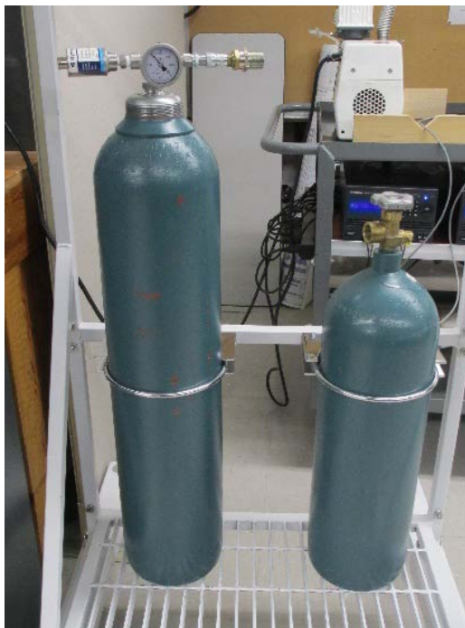
Figure 18: Picture of the buffer tank on the left and the helium charge cylinder on the right.
