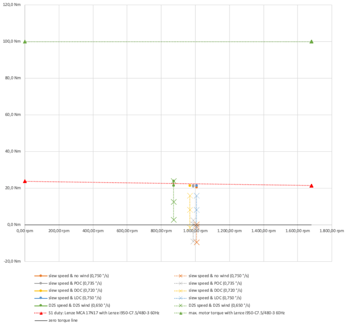
Figure 64 Elevation torque-over-speed diagram and operating points of drive system by Lenze, the gearbox ratio is changed to 1200:1
