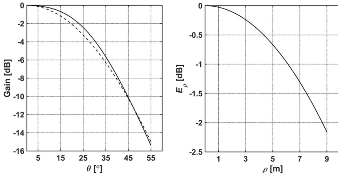
Figure 5 – The associated feed pattern and aperture field distribution of the ngVLA mapping function.
