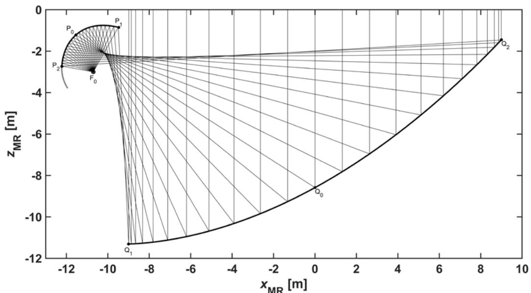
Figure 2 – ngVLA 18-meter reflector system with an optical ray trace overlay.
