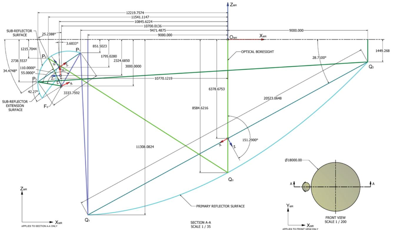
Figure I – 18-meter antenna optical system critical dimensions.
