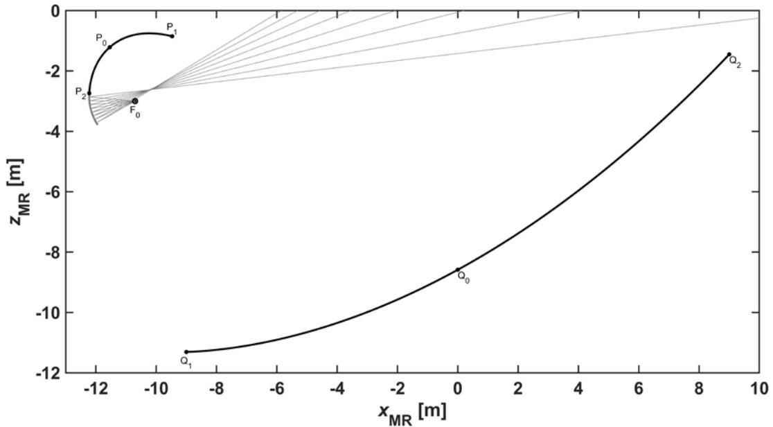
Figure 3 – ngVLA 18-meter reflector system with the ray trace overlay of rays from the secondary extension.
