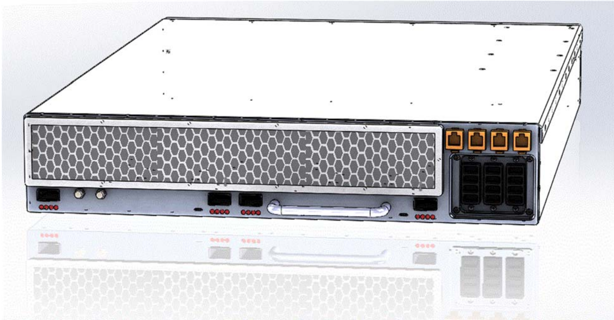
Figure 5-17 Rendering of the 2U air-cooled 19" rack-mount TALON LRU for SKA Mid.CBF. The 1U DCLC LRU would be ½ the height. Note that this LRU has no front-rail mounting ears because of fiber routing space limitations; instead, it is mounted on custom slide rails in a 19" rack, and quick-lock secured to the rack at the back
