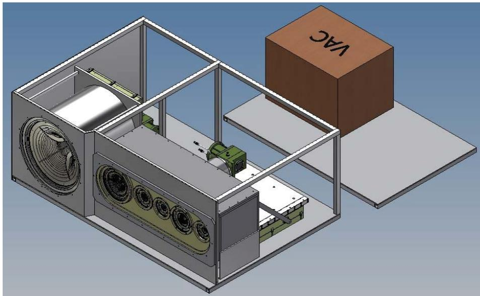
**Figure 14 - Front End subsystem enclosure, opened to show cryostats and IRD assembly.**
