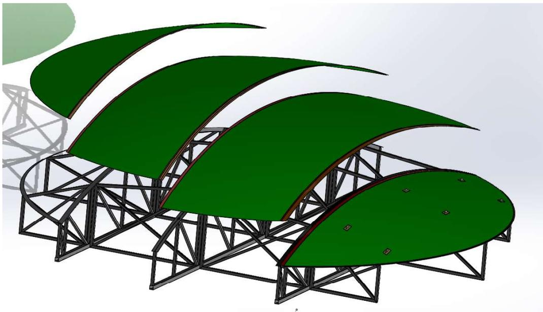
**Figure 25 Four primary surface parts being added to the assembly jig**
