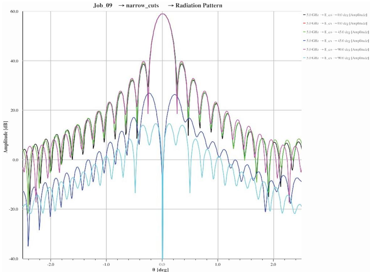
Figure 15 - Plot of close-in beam pattern for ngVLA\_6 using the corrugated feed horn.
