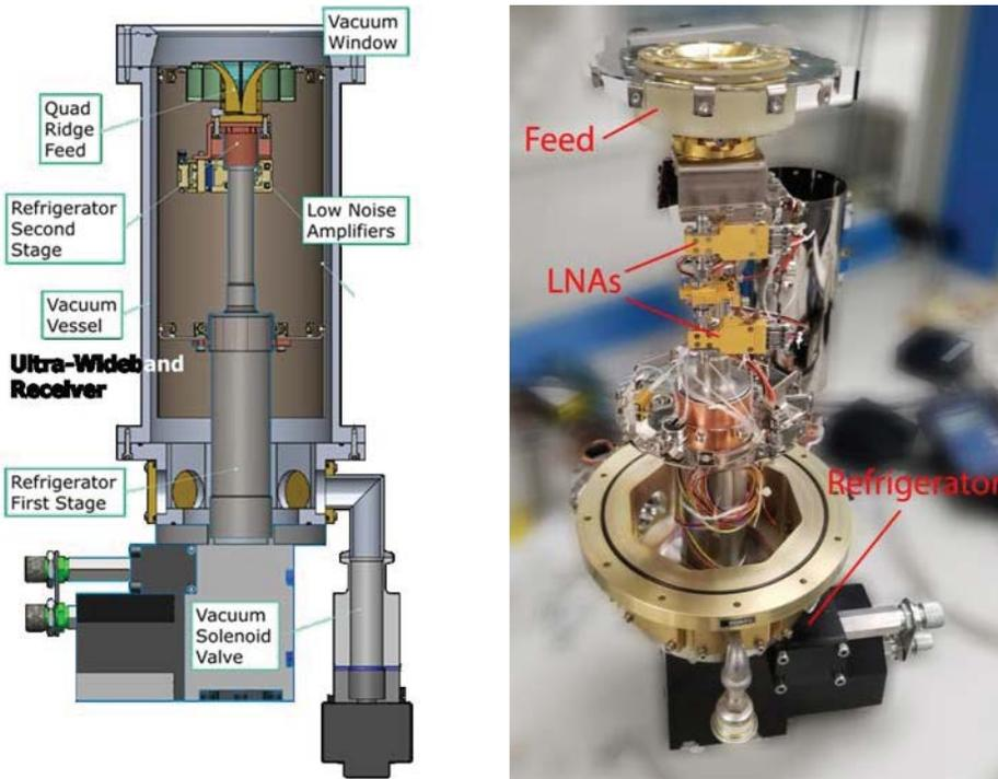
Figure 20 - JPL ultra-wideband receiver cryostat, side rendering and inside view.
