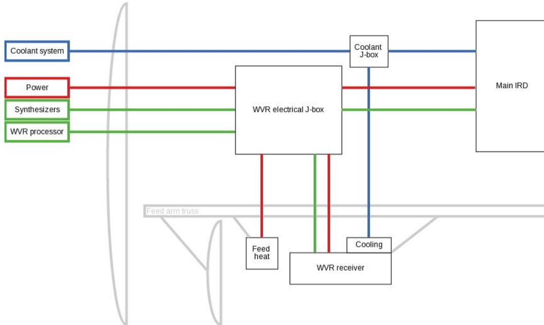
Figure 3 - WVR subsystem overview and interfaces.
