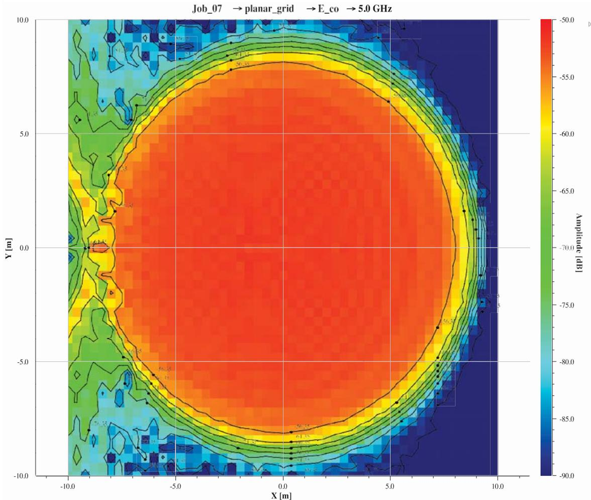
Figure 4 - Copolar aperture illumination on the plane at  $z = 0$ .
