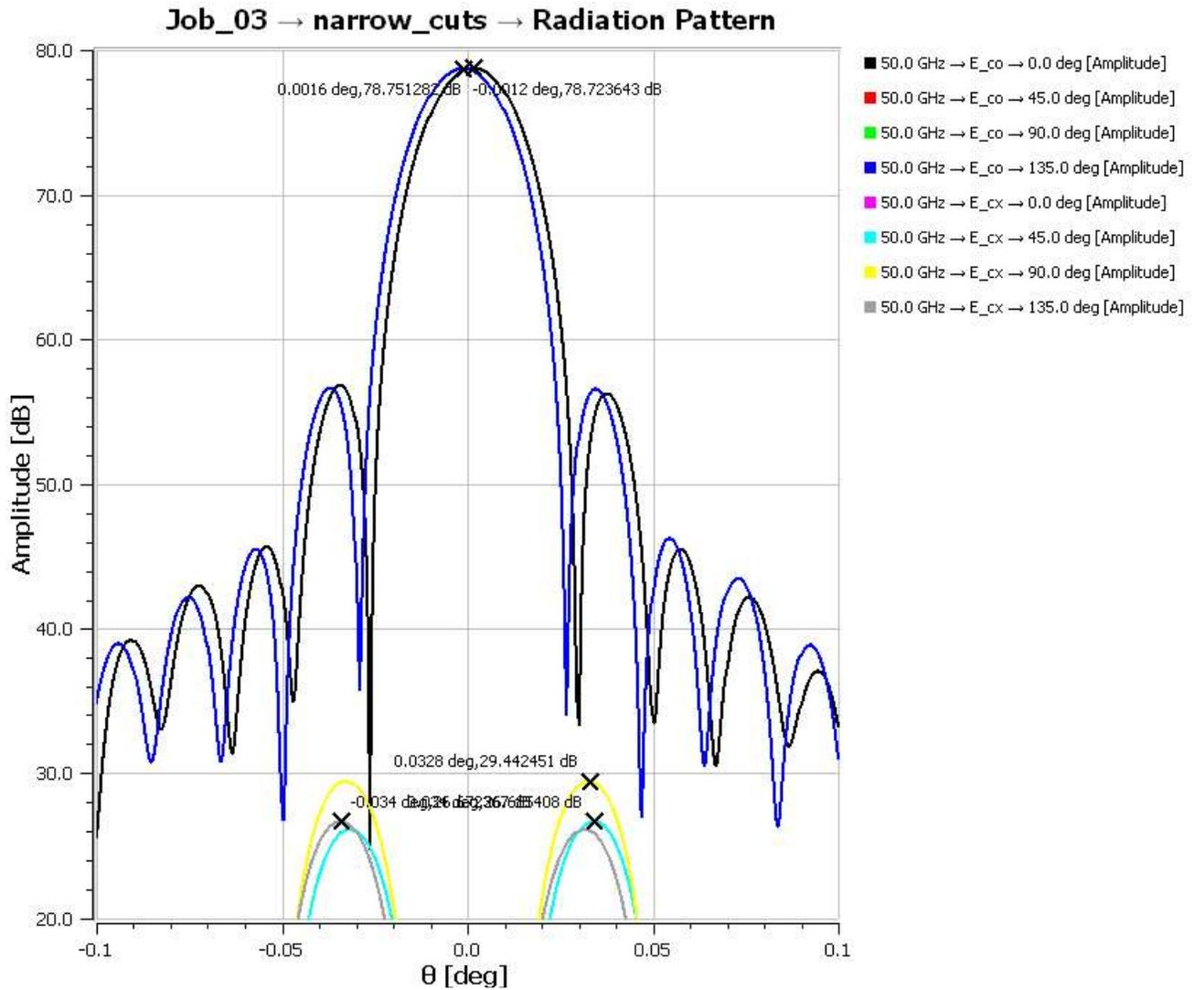
**Figure 60 Beam Pattern, Thermal Gradient, 50 GHz**
