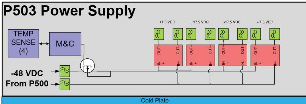
Figure 5 - P503 block diagram.
