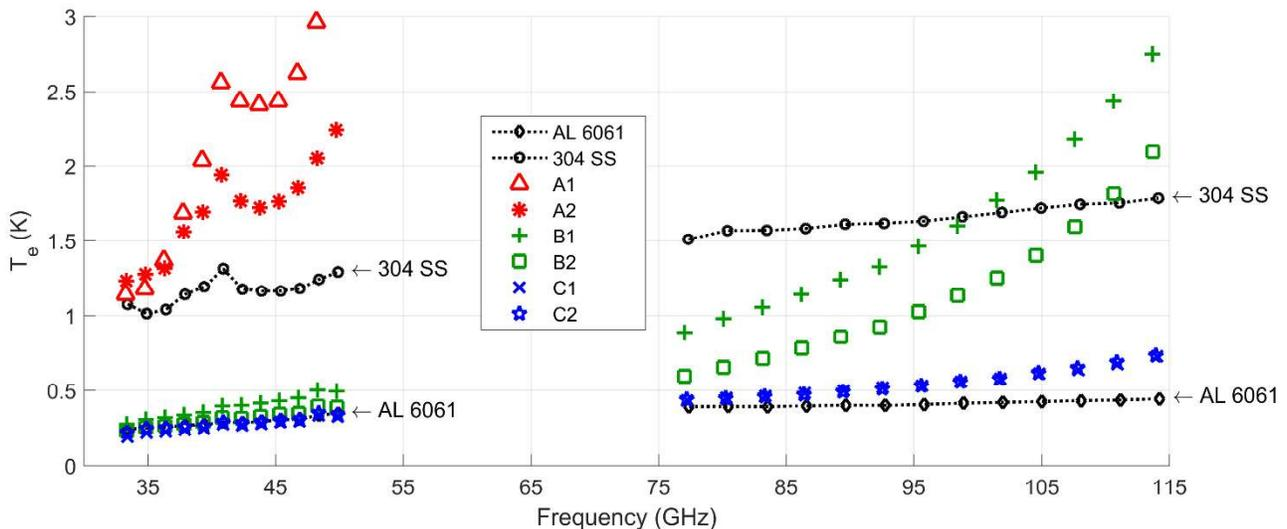
Figure 37 Reflector Surface Noise Measurement Results
