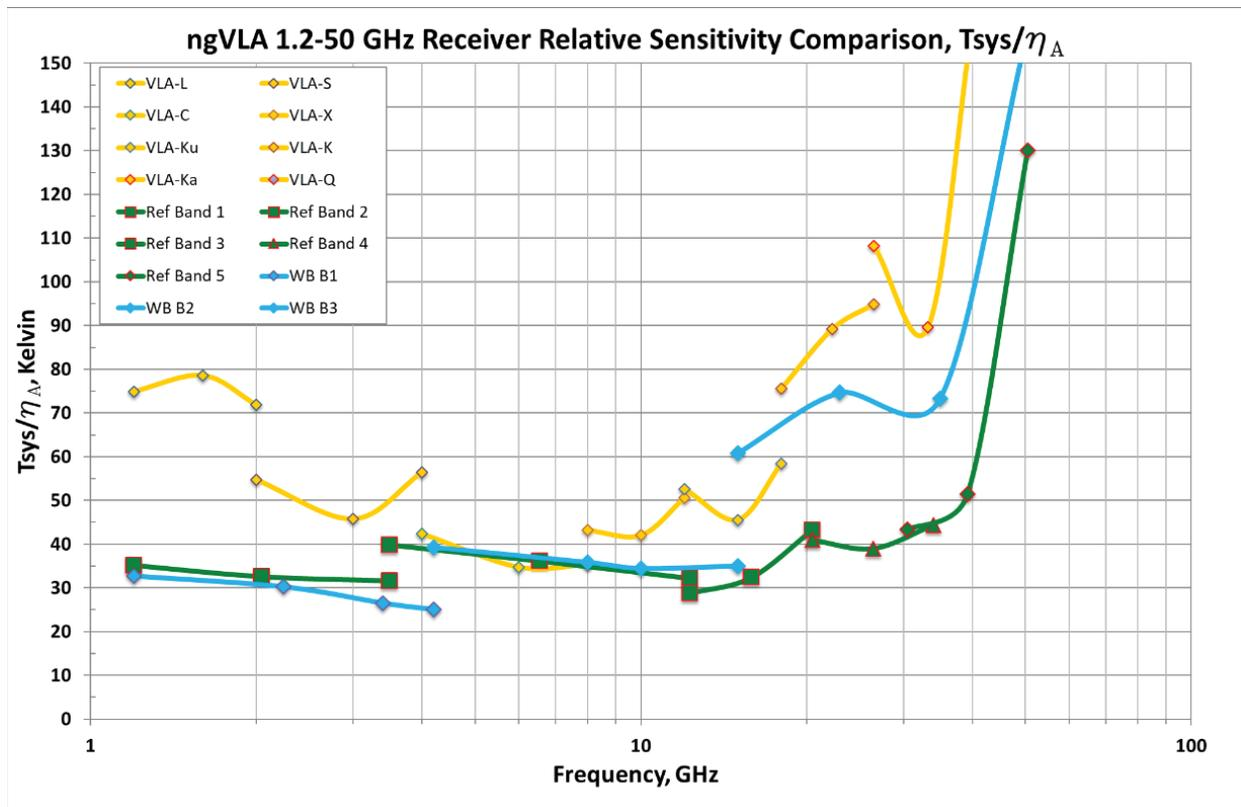
Figure 7 - Relative sensitivity of ngVLA reference Bands 1–5, versus a single VLA antenna.
