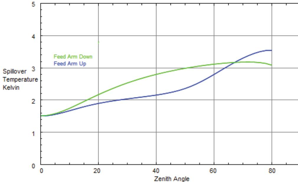
Figure 11 - ngVLA Design#6, spillover curve at 5 GHz with ideal feed and SKA noise model.
