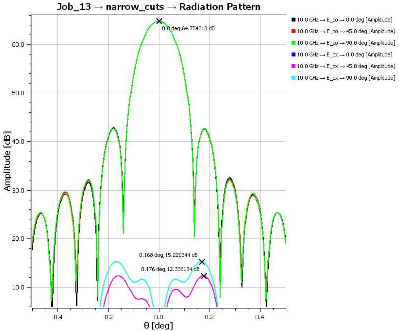
**Figure 45 90° Elevation Angle Gravity Load Case Beam Pattern 10 GHz**
