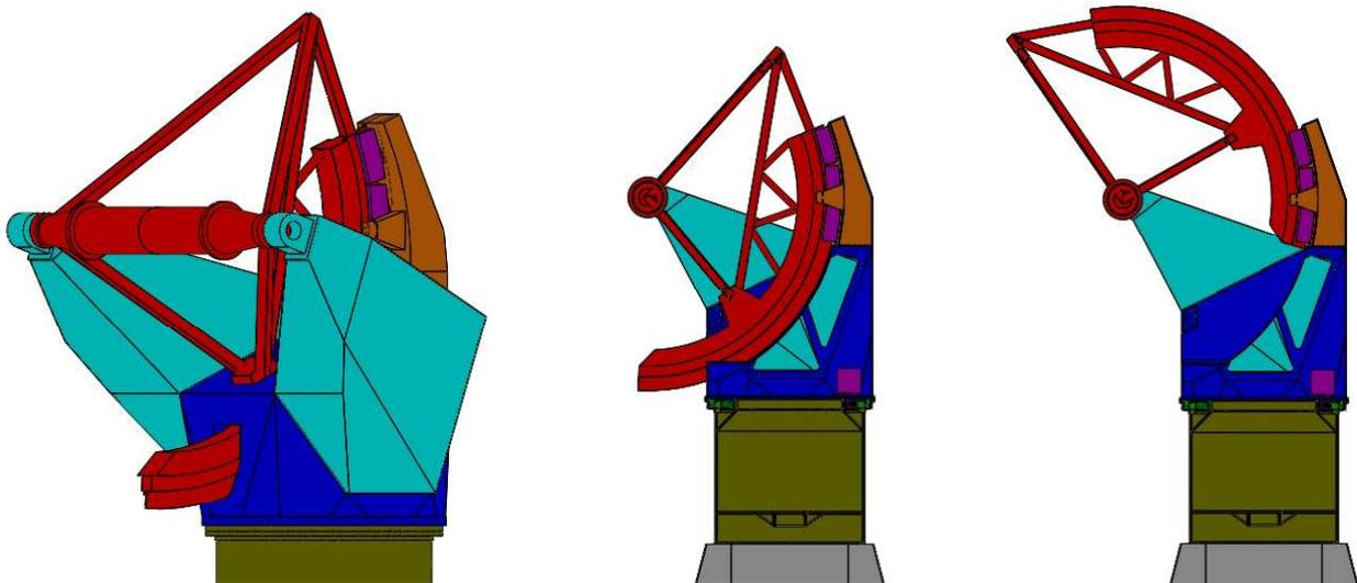
Figure 30 Yoke and Elevation Drive Structure
