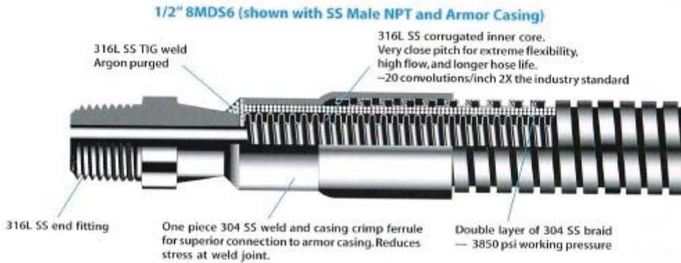
Figure 1 - Armored flex-line cross section view.
