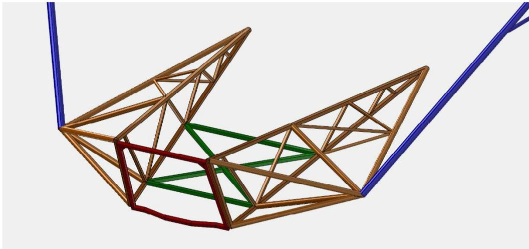
**Figure 17 Secondary and Feed Support Structure.**
