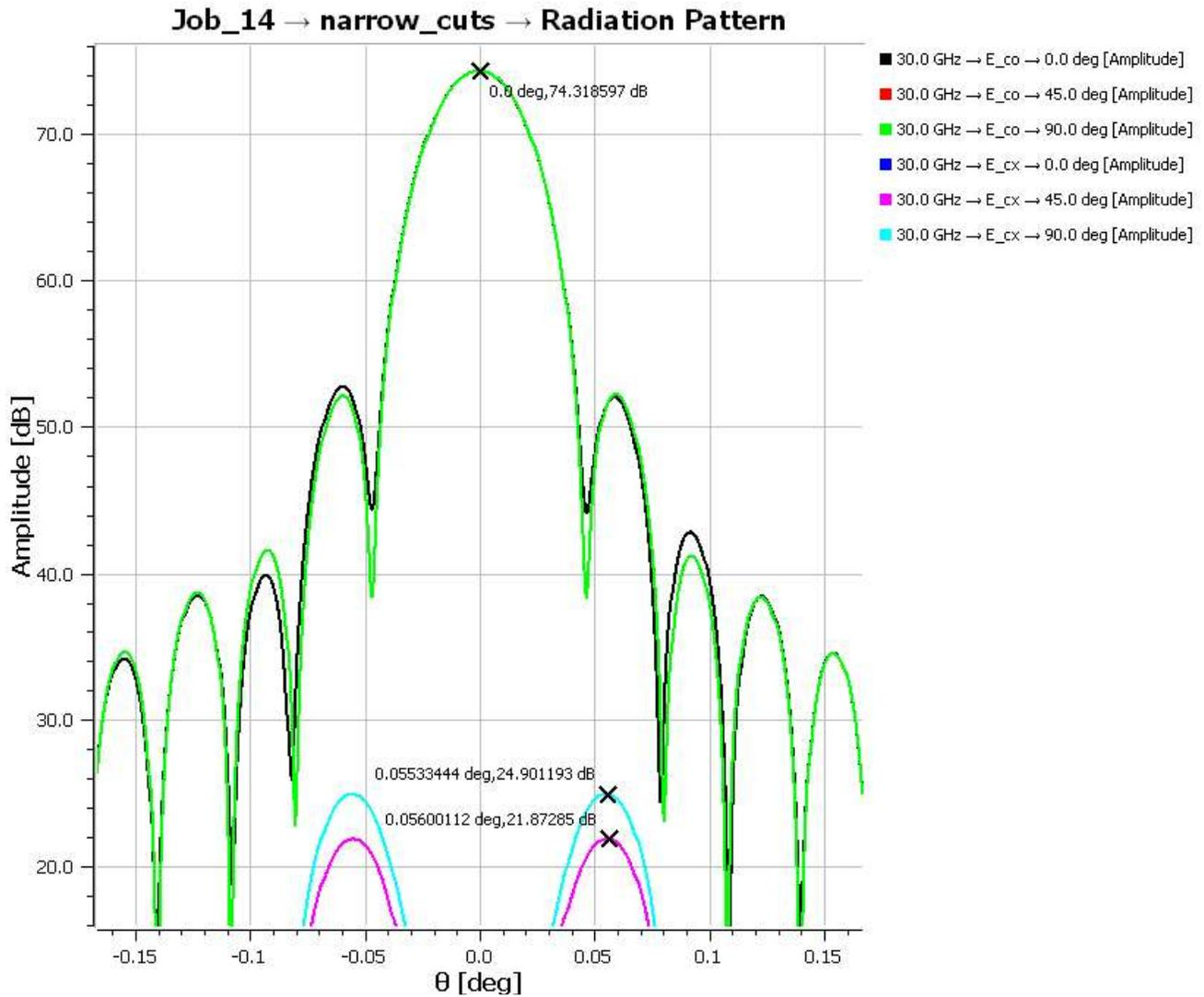
Figure 46 90° Elevation Angle Gravity Load Case Beam Pattern 30 GHz
