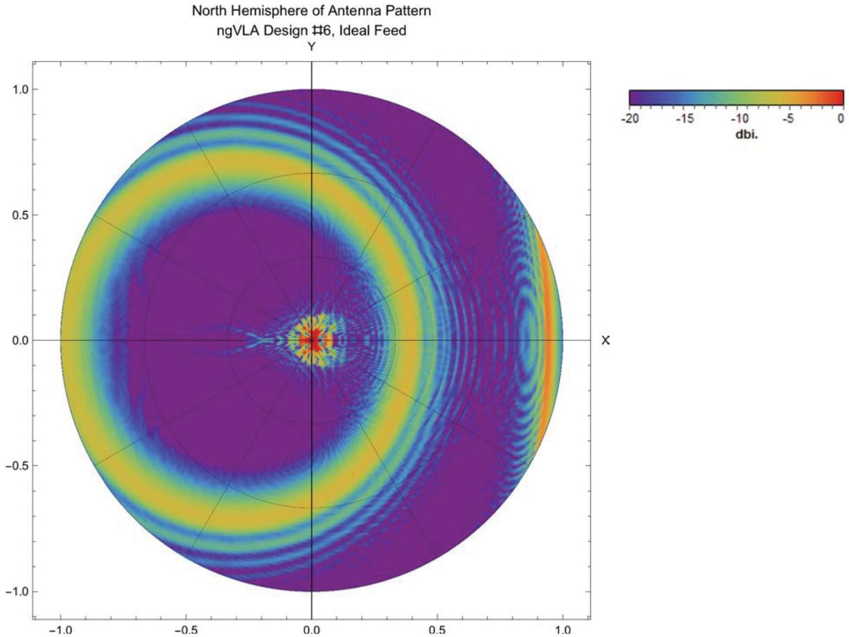
**Figure 6 - Unit disk projection of the far-field response, north hemisphere.**
