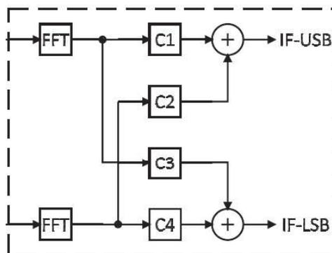
Figure 6 - Side-band separation processor.
