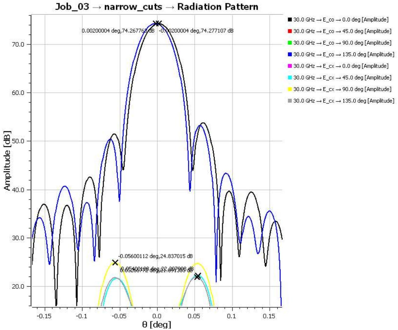
Figure 56 Beam Pattern, Thermal Bath 30 GHZ
