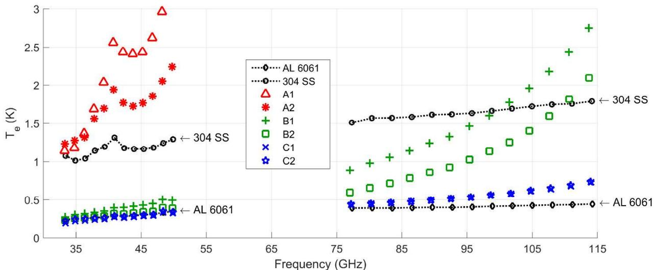
Figure 12 Reflector Surface Noise Measurement Results
