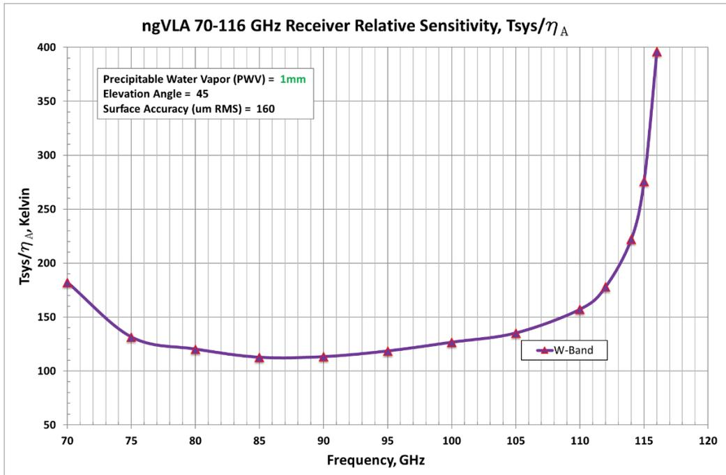
Figure 8 - Relative sensitivity of ngVLA reference Band 6.
