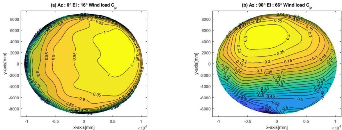
**Figure 48 Wind load cases: (a) & (c) are pressure coefficient contour plots at Az: 0° El: 16° and Az: 90° El: 66°.**
