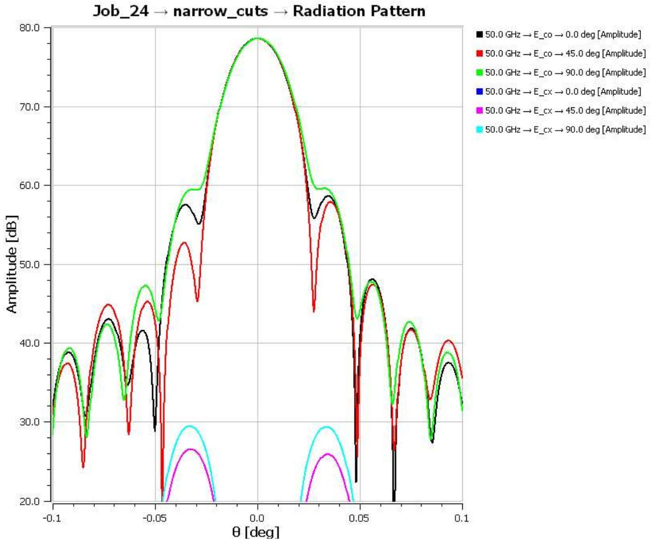
**Figure 44 15° Elevation Angle Gravity Loading Case Beam Pattern 50 GHz**
