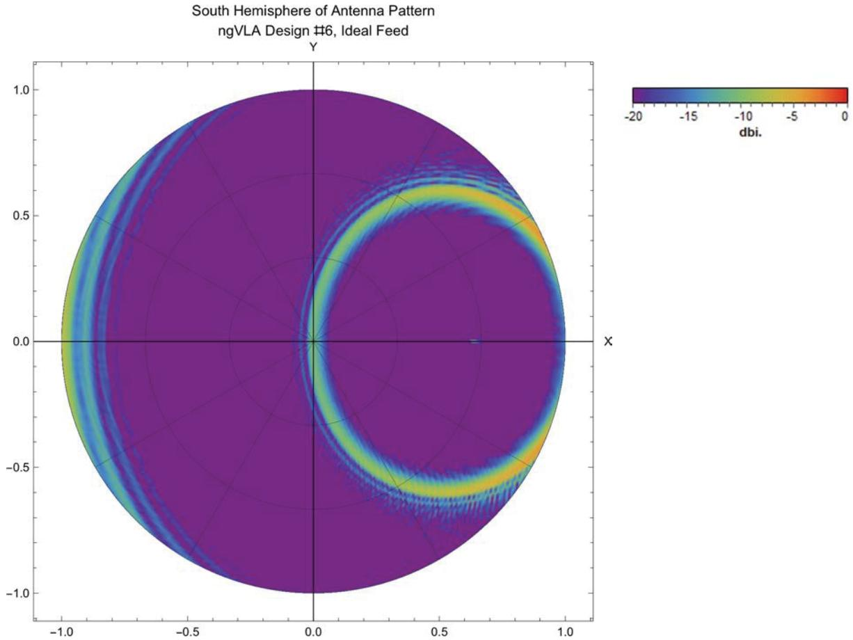
Figure 7 - Unit disk projection of far-field response, south hemisphere.
