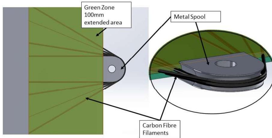
**Figure 2 Primary surface edge adjuster tab concept**
