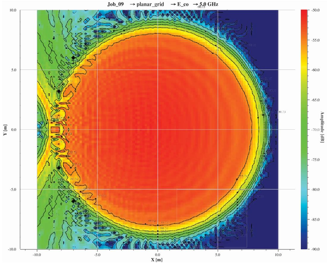
Figure 14 - Illumination pattern of ngVLA\_6 in  $z = 0$  aperture plane using the corrugated feed horn.
