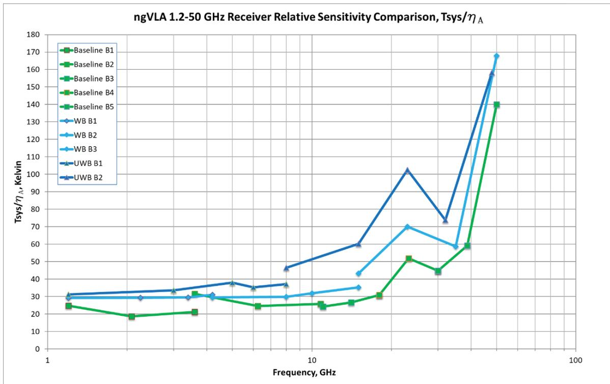
Figure I - Relative sensitivity of baseline, wideband, and UWB receiver configurations.
