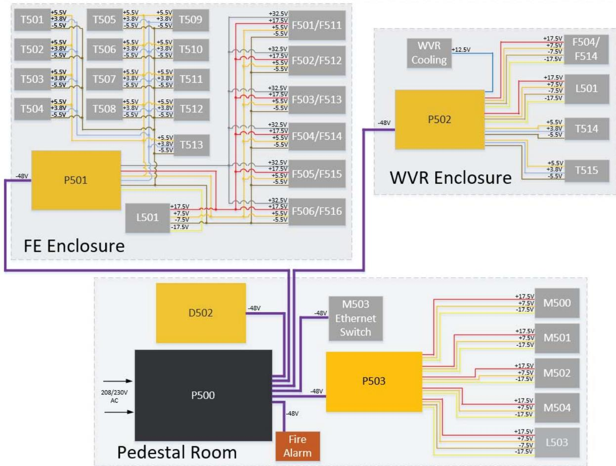
Figure 1 - Block diagram of DC Power Supply system.
