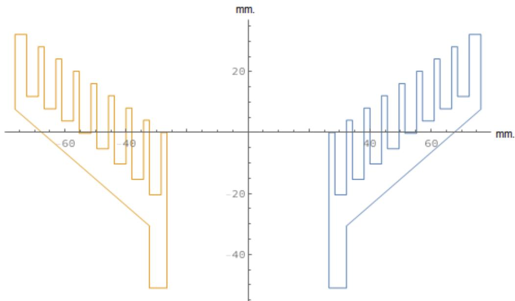
Figure 12 - Cross-section of corrugated feed horn used for analyzing the ngVLA\_6 optics performance.
