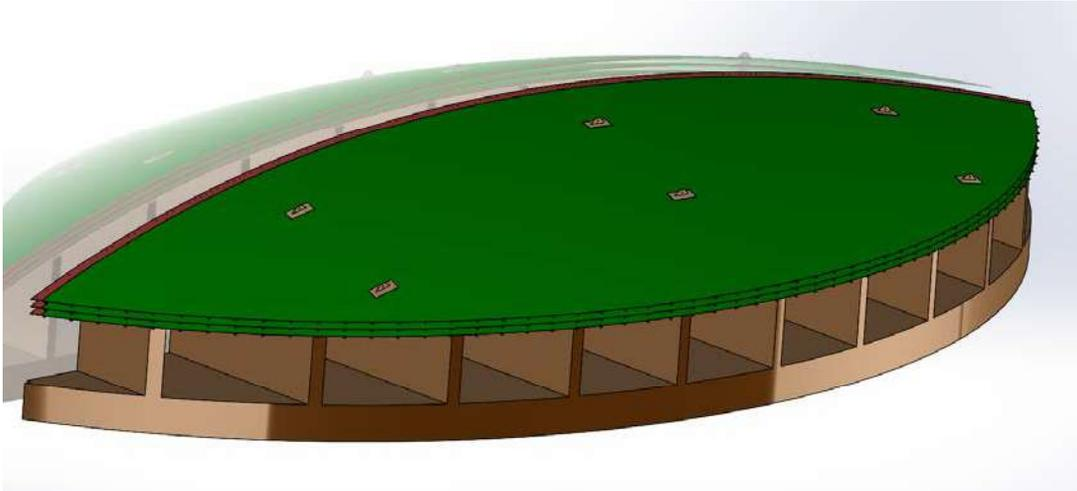
**Figure 24 Nesting multiple instances of primary surface pieces for transport to remote sites**
