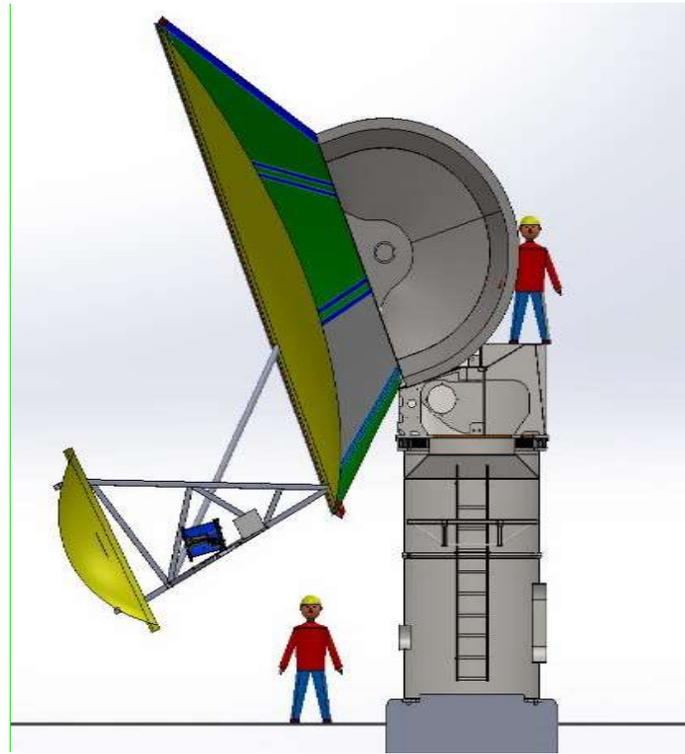
**Figure 6 Cross Section of Antenna at Low ( $12^\circ$ ) Elevation Angle**
