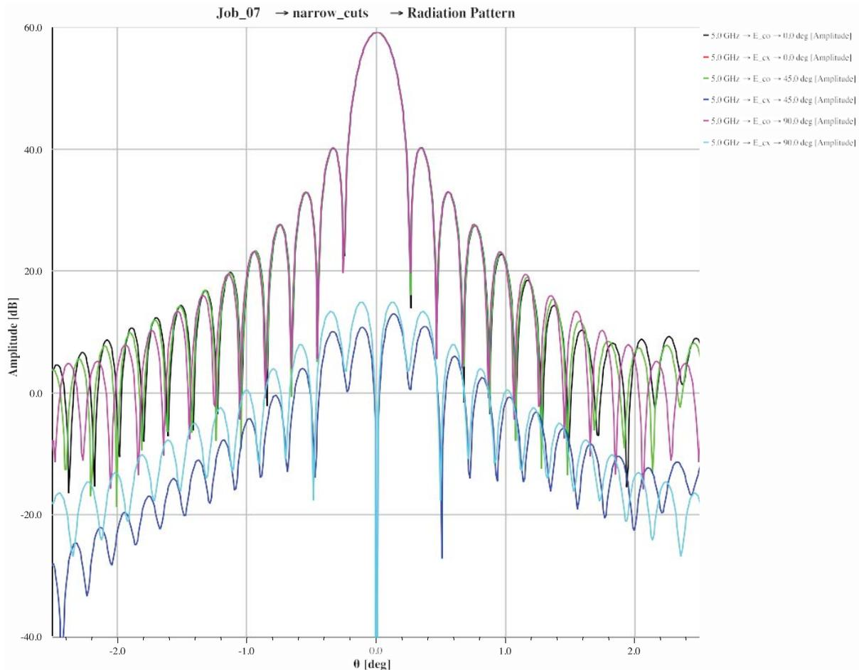
Figure 5 - Close-in far-field pattern using azimuth cuts at 0°, 45°, and 90°.
