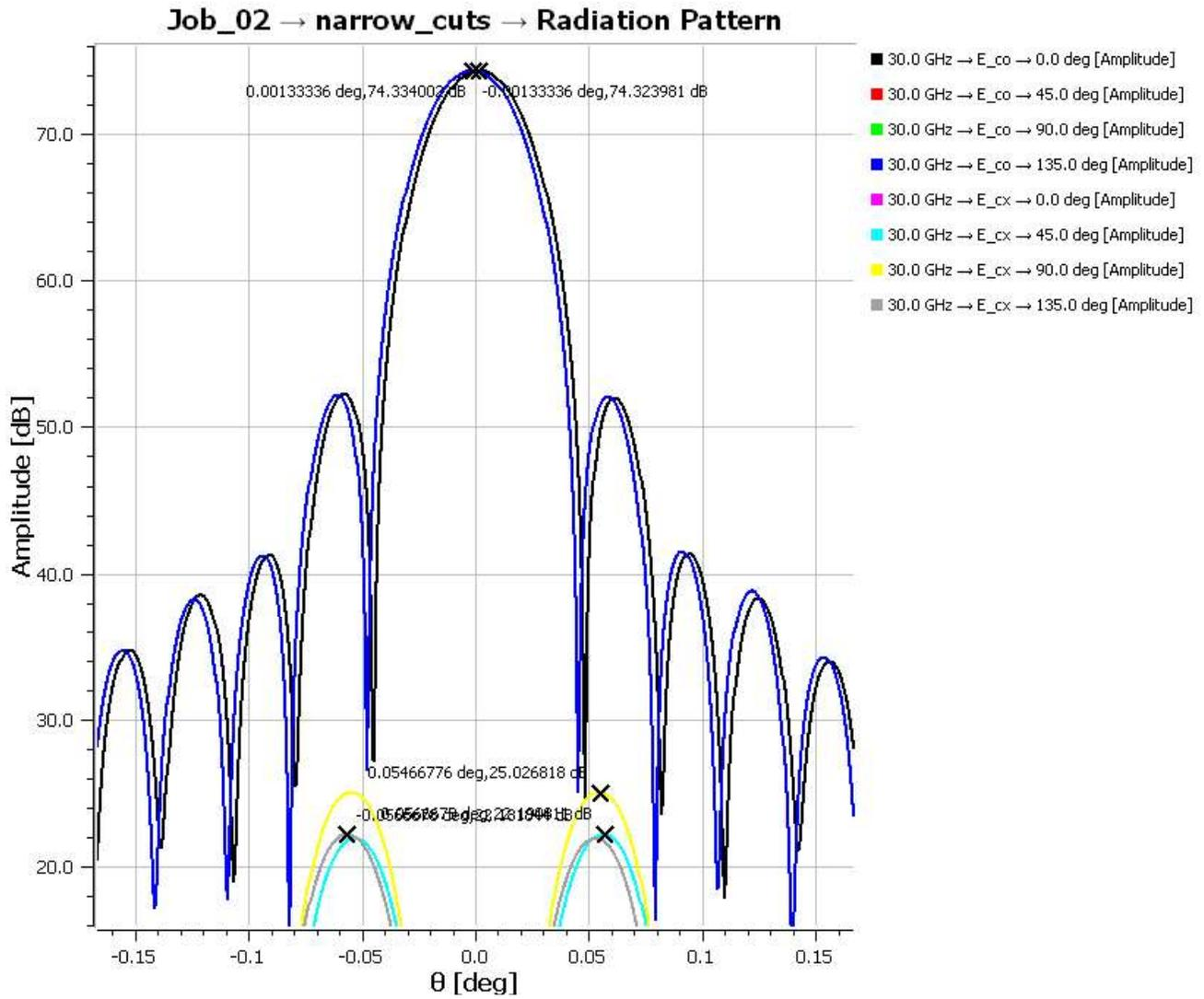
Figure 59 Beam Pattern, Thermal Gradient, 30 GHz
