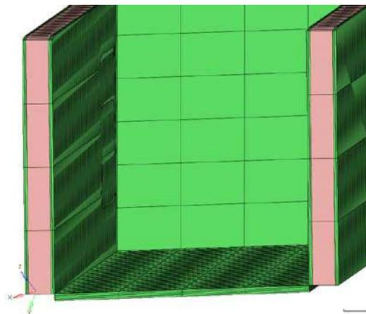
**Figure 17 oBUS rib Laminate schedule (green layer: carbon qiso, pink layer: foam core)**
