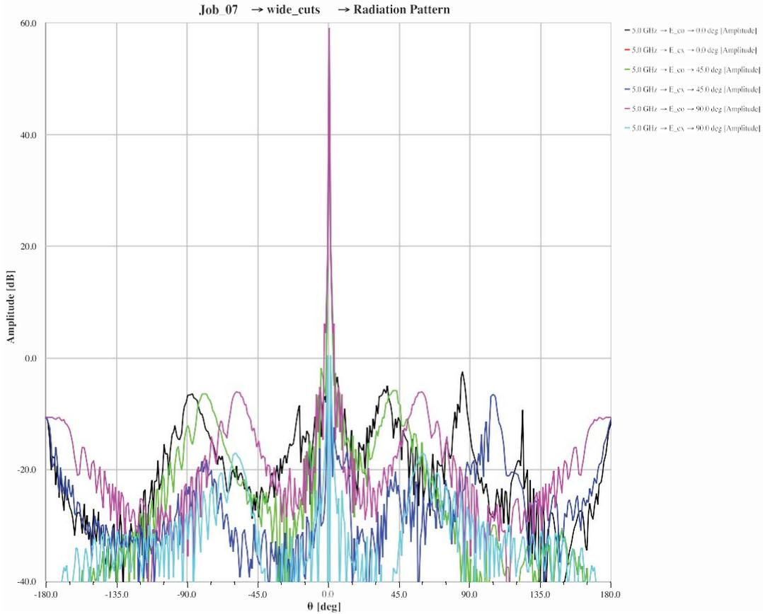
Figure 8 - Plot of far-field pattern over the entire range of elevation angles and azimuth cuts of  $0^\circ$ ,  $45^\circ$ , and  $90^\circ$ .
