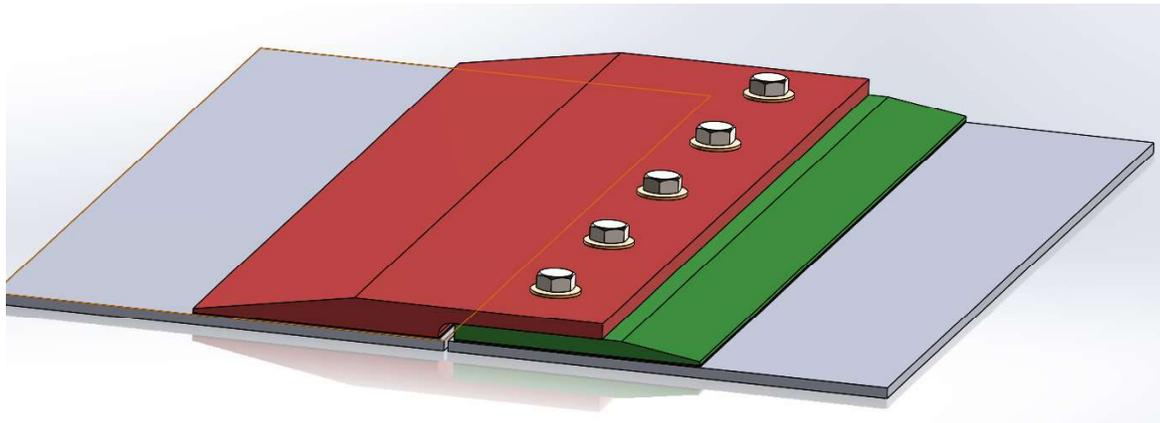
**Figure 19 Proposed multi-piece primary surface connection detail**
