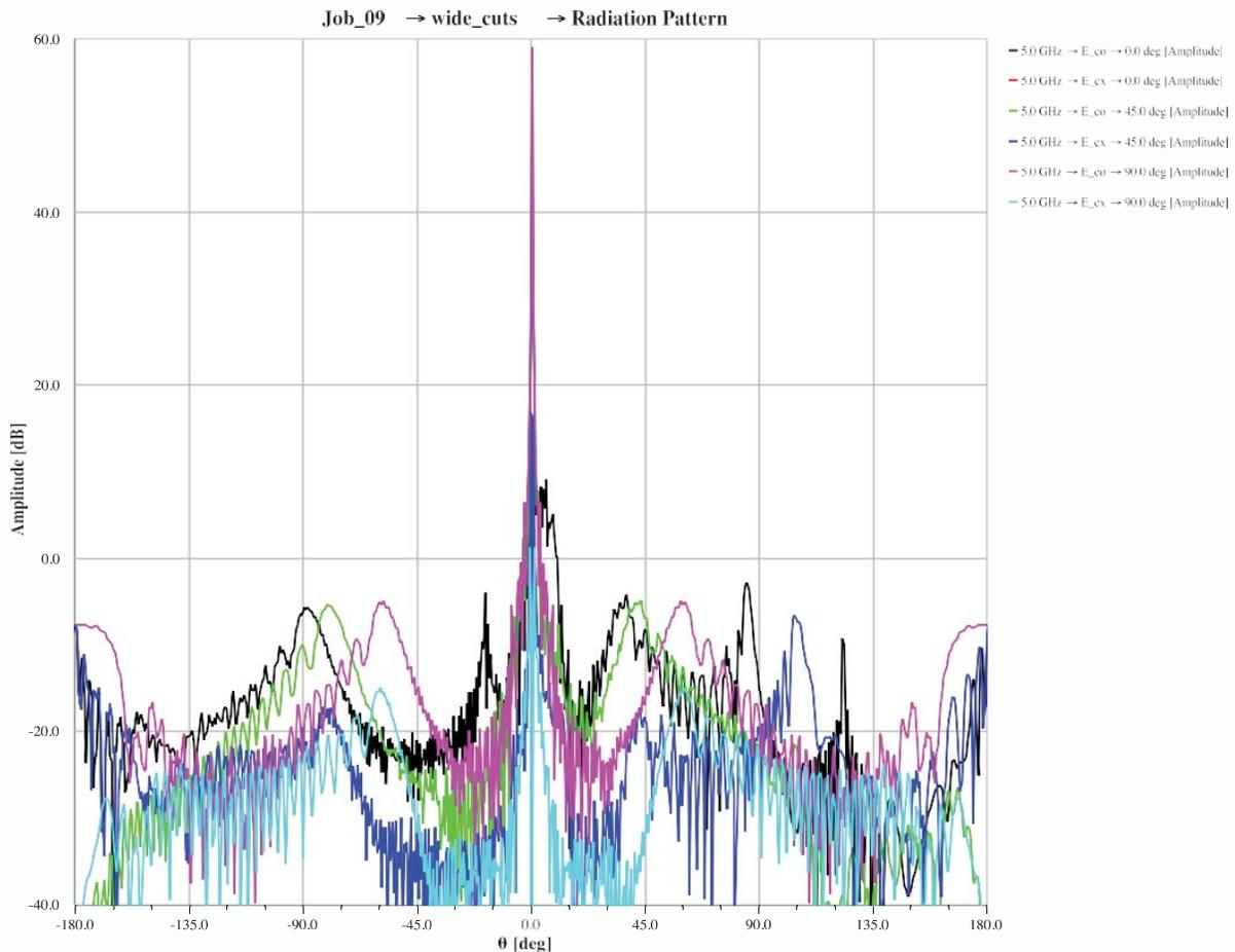
Figure 18 - Plot of wide-angle far-field illumination pattern using corrugated feed horn.
