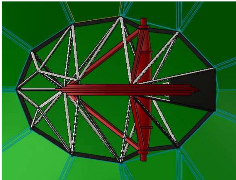
Figure 13 iBUS with its 11 Discrete Connection Points to the oBUS
