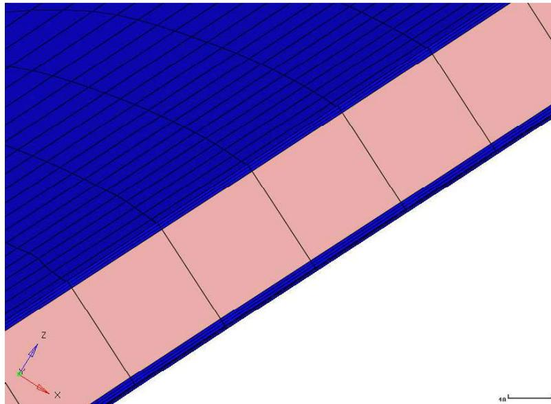
**Figure 16 oBUS Laminate schedule (blue layer: carbon qiso, pink layer: foam core)**
