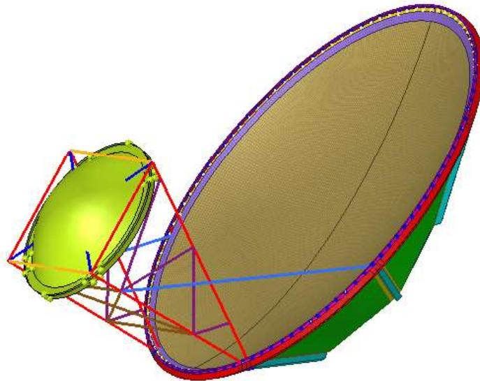
**Figure 13 6m Reflector Assembly**
