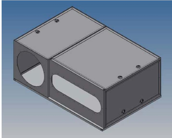
Figure 2 - Front End receiver enclosure.
