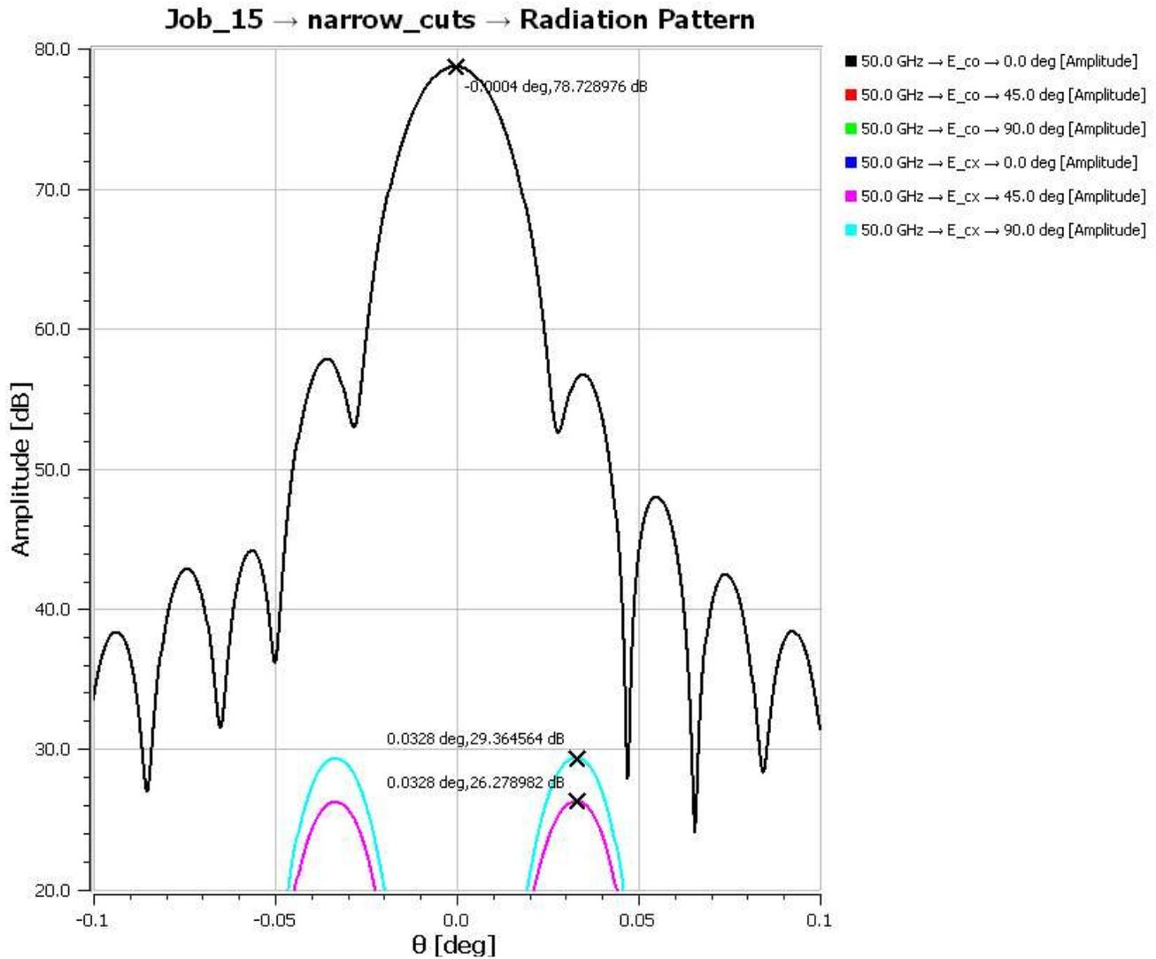
**Figure 47 90° Elevation Angle Gravity Load Case Beam Pattern 50 GHz**
