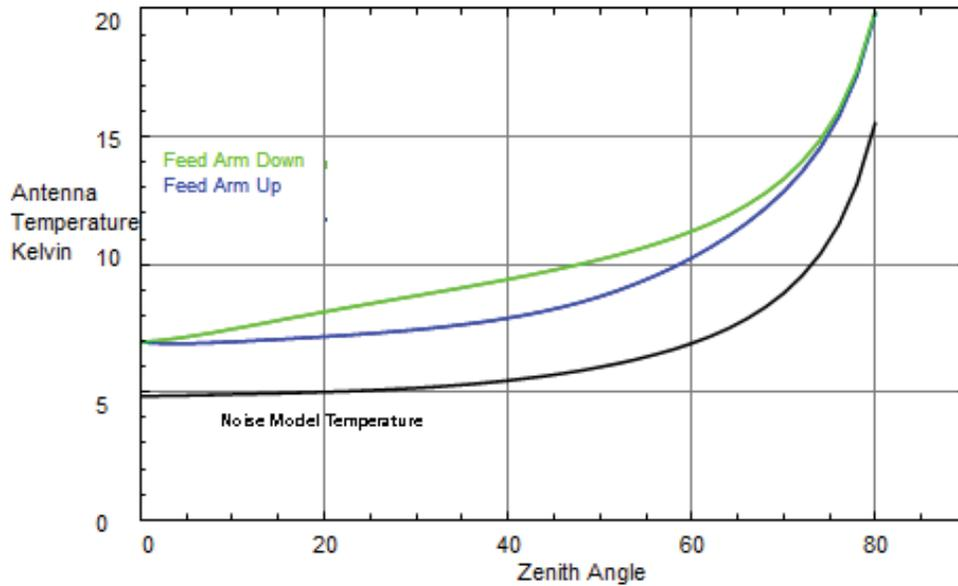
Figure 19 - ngVLA\_6 tipping curve at 5 GHz with corrugated feed horn and SKA noise model.
