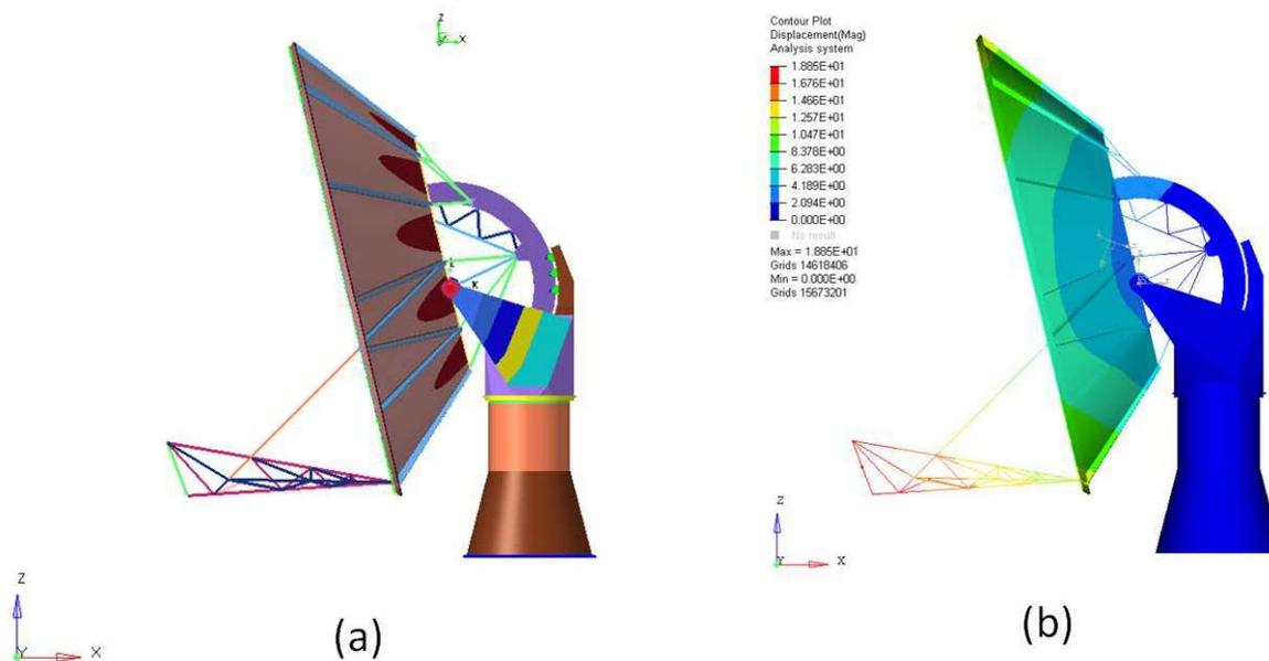
Figure 38 (a) Integrated FE model (15° elevation angle), (b) example FEA results
