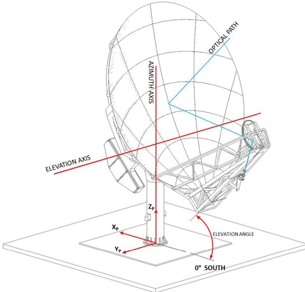
**Figure 2 - Cartoon of the antenna pad coordinate system and major axes. Separate Cartesian reference frames define each mirror surface, the focus, and the pad respectively. Antenna design is diagrammatic only.**
