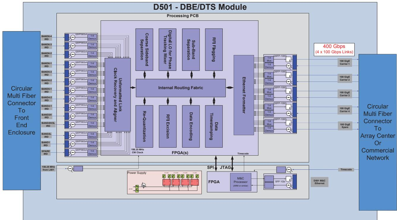
Figure 9 - Block diagram of antenna DBE/DTS subsystem.
