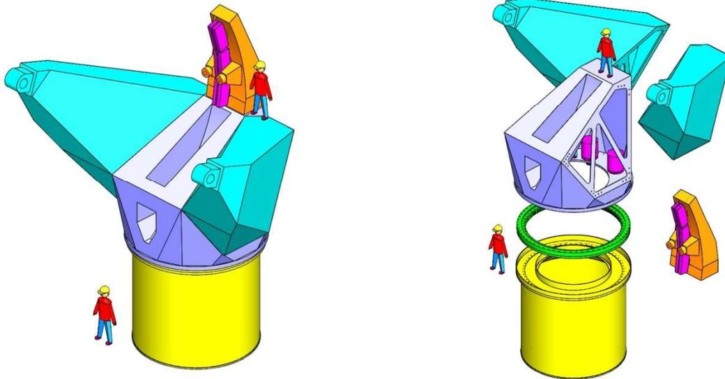
Figure 29 Azimuth Rotating Structure
