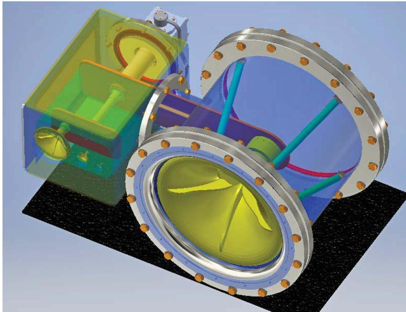
Figure 16 - 3D rendering of Caltech 4-band, single-cryostat Front End concept.
