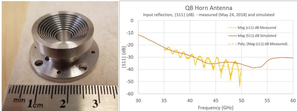
**Figure 5 - Prototype Q-band axially corrugated feed horn.**
