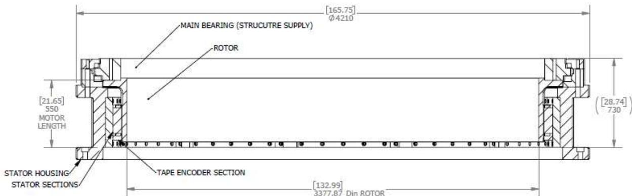
**Figure 35 Direct Drive Azimuth Motor X-section**
