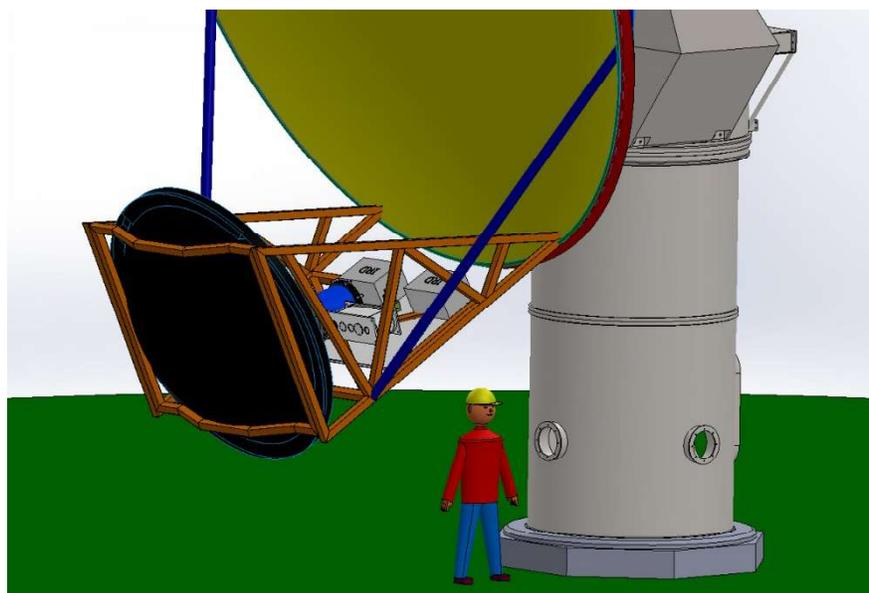
**Figure 8 6m Secondary Support Structure.**
