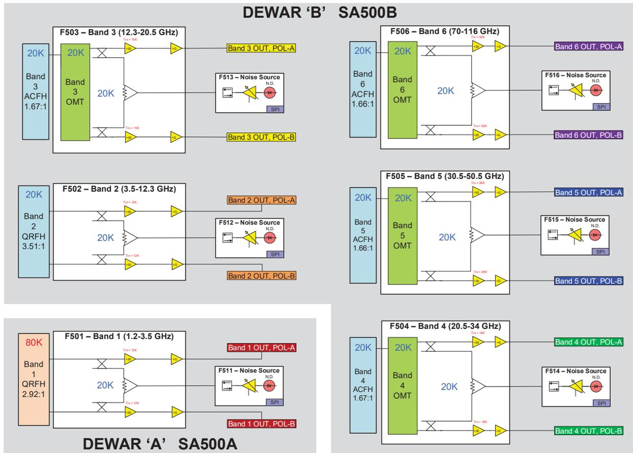
Figure 10 - Block diagram of Front End subsystem.
