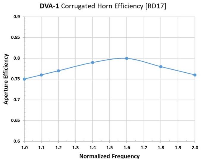
Figure 3 - DVA-1 corrugated feed horn, 3D rendering and aperture efficiency.
