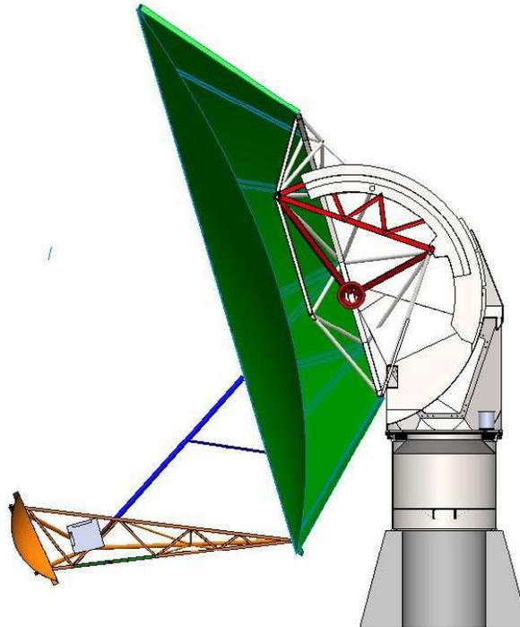
Figure 12 Cross Section of Antenna at Low ( $12^\circ$ ) Elevation Angle
