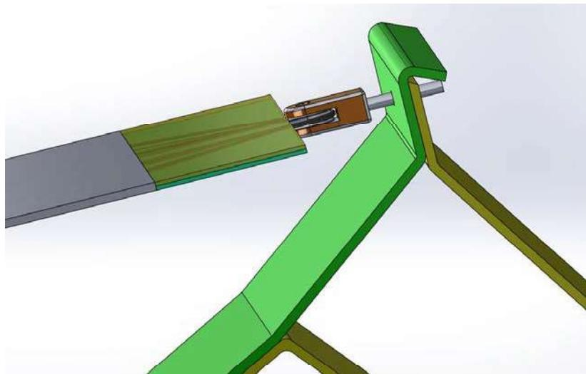
**Figure 3 Primary surface edge adjuster with oBUS**
