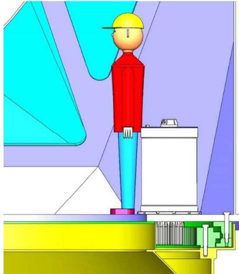
Figure 36 Direct Pinion/Gear Drive
