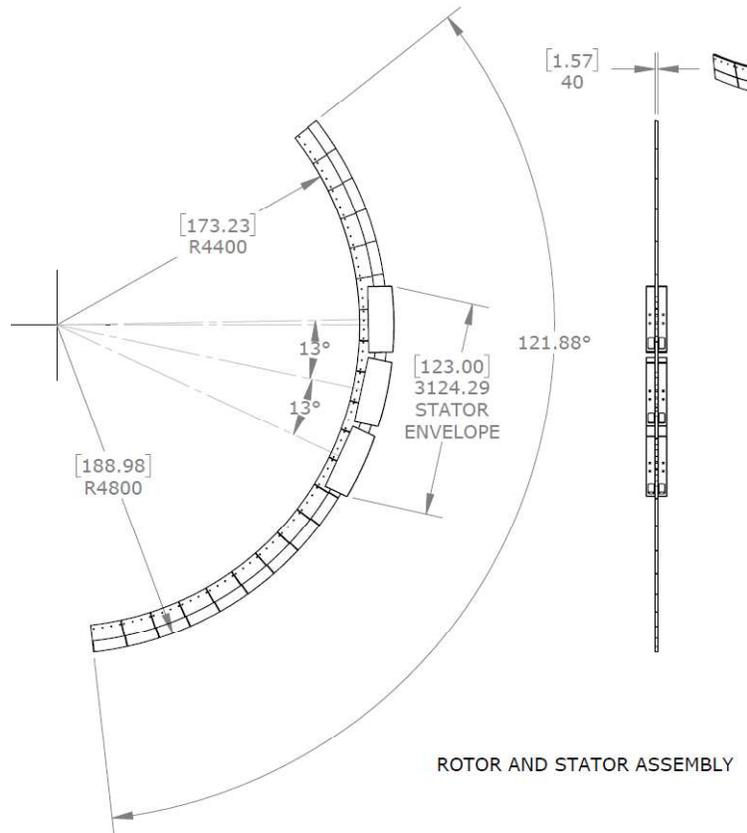
**Figure 28 Elevation Drive Configuration**
