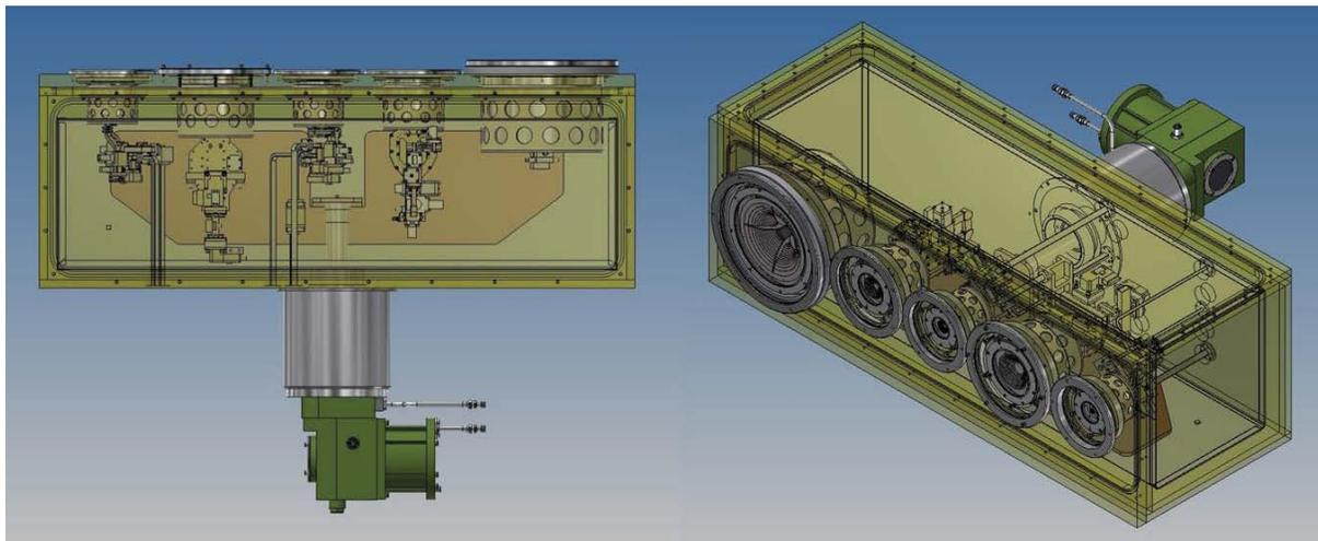
Figure 12 - ngVLA reference receiver Bands 2-6 (cryostat B).
