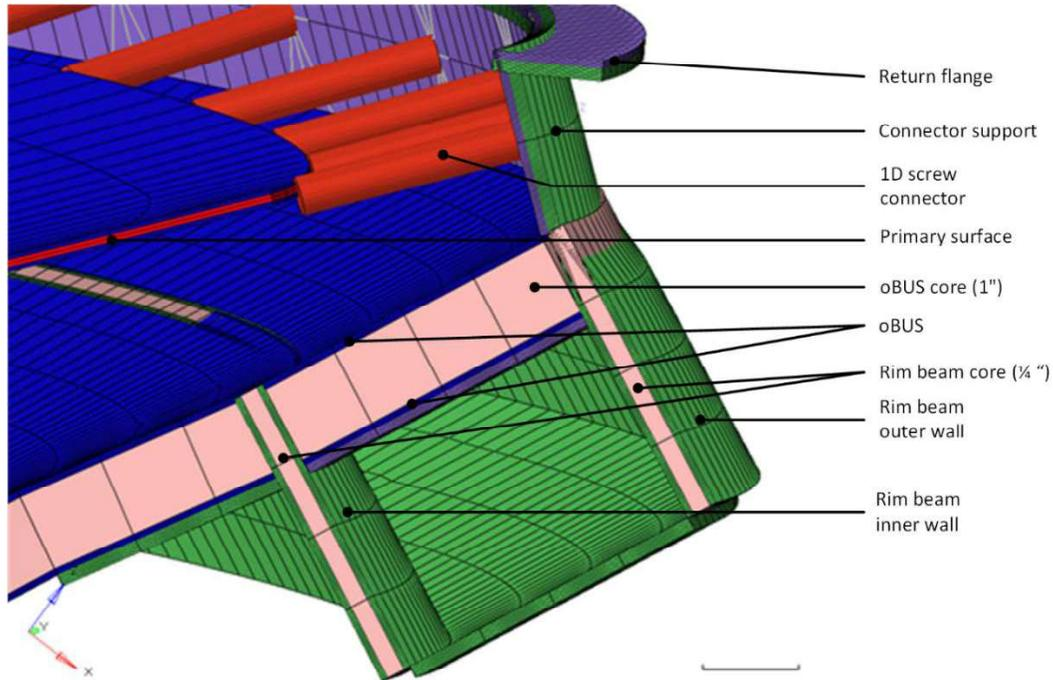
**Figure 18 Cone back-primary laminate schedule and foam core (blue layer: carbon QISO, magenta layer: carbon uni, grey layer: foam core).**
