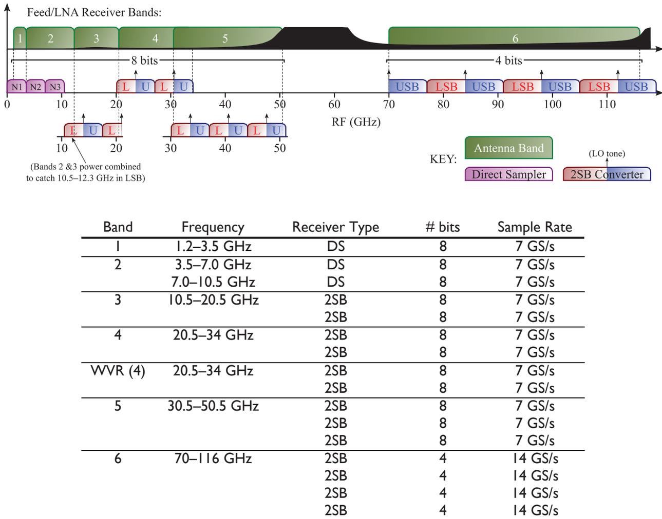
Figure 2 - Integrated Receiver/Downconverters and Digitizers frequency plan.
