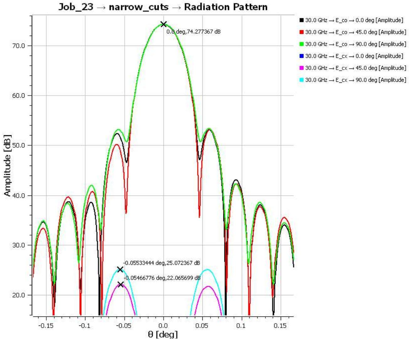
Figure 43 15° Elevation Angle Gravity Loading Case Beam Pattern 30 GHz
