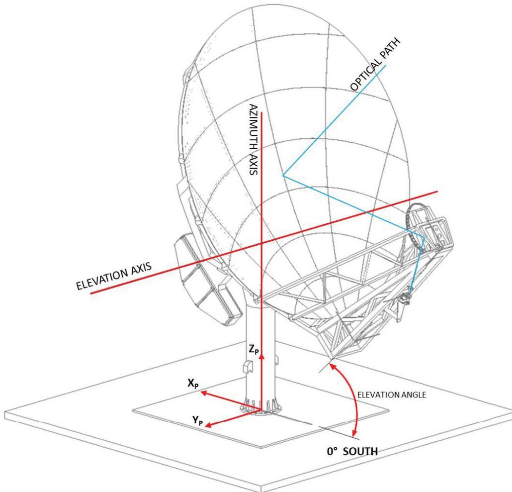
**Figure 2 - Diagram of the antenna pad coordinate system and major axes. Separate Cartesian reference frames define each mirror surface, the focus, and the pad respectively. Antenna design is diagrammatic only.**
