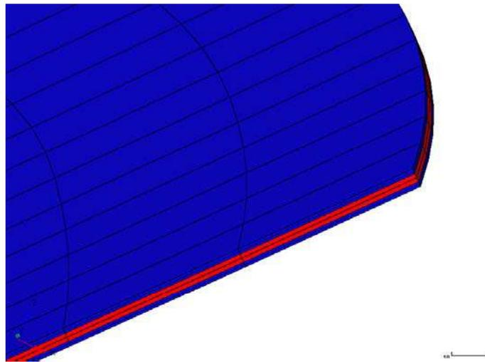
Figure 15 Primary surface Laminate schedule (blue layer: carbon qiso, red layer: triaxial carbon).
