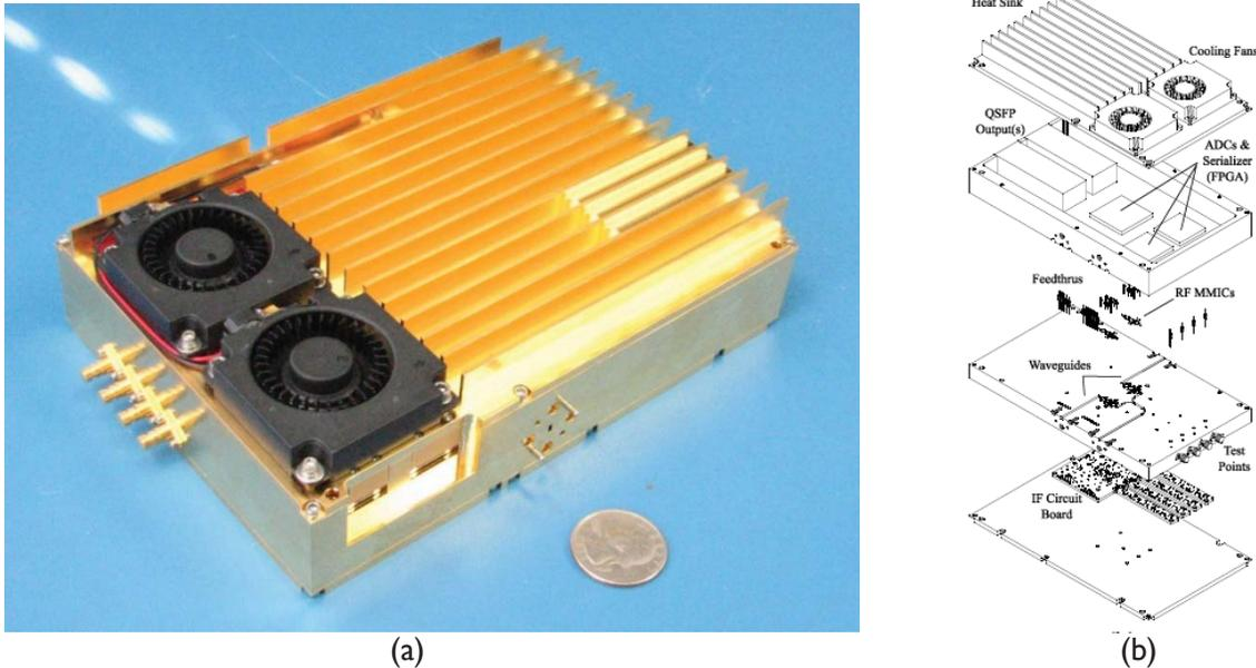
**Figure 7 - Prototype W-band IRD 2SB receiver module. (a) Photo. (b) Exploded view of internal construction. Note that this is only a prototype. The cooling fans are needed here since the power-saving Serial ADC ASIC was not yet available. The reference design version will be smaller, consume less power, and be cooled without fans by attachment to a temperature-controlled plate.**
