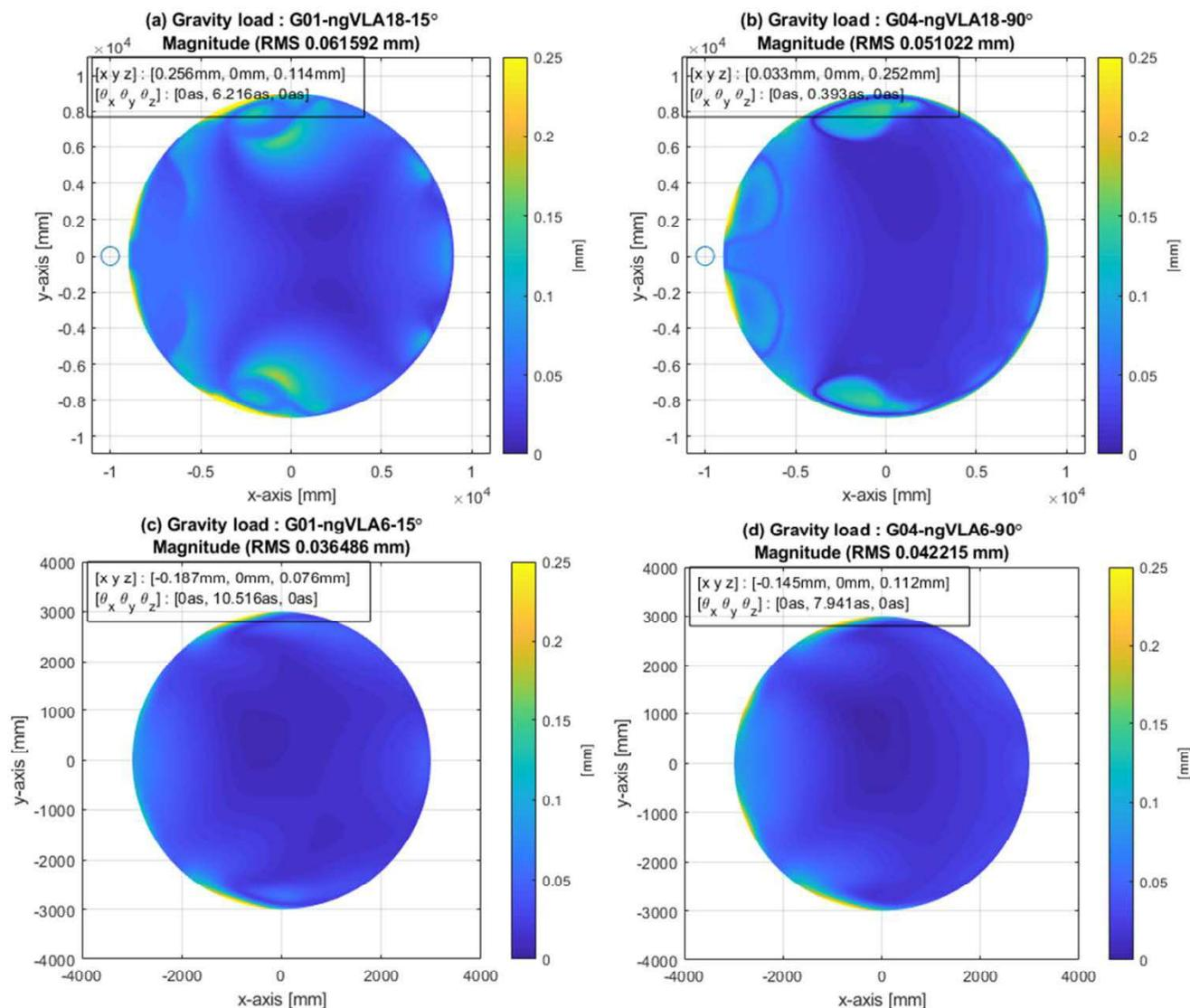
**Figure 21 Surface RMS error under Gravity load cases for ngVLA 18m (a) 15° and (b) 90° elevation angles and ngVLA 6m (c) 15° and (d) 90° elevation angles.**
