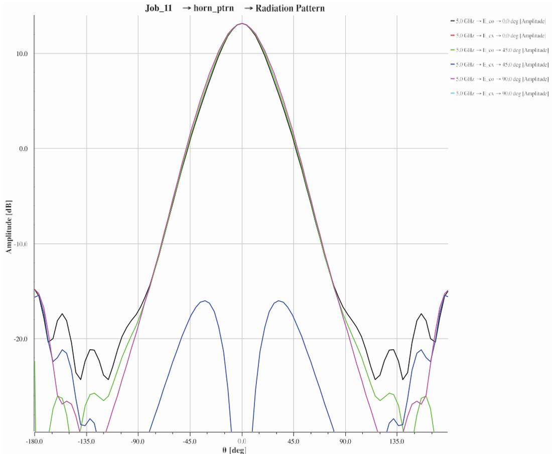
Figure 13 - ngVLA\_6 feed pattern plot, using the corrugated horn feed shown in Figure 12.
