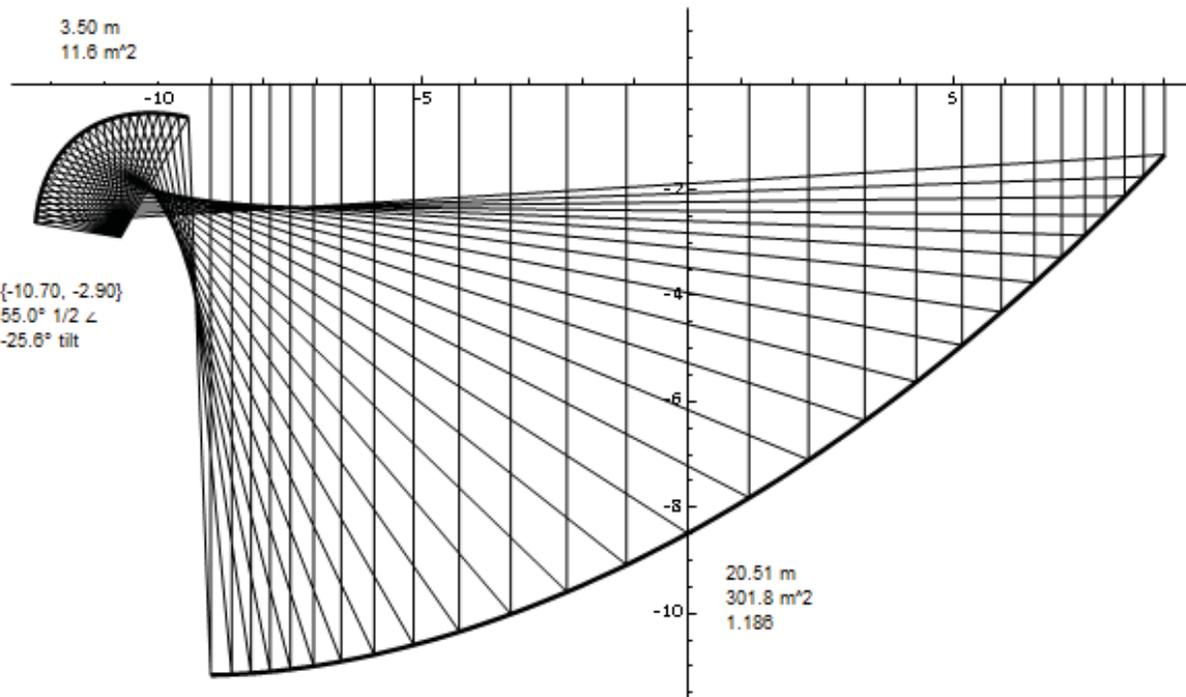
Figure 3 - ngVLA\_6 Optics: Cross-section in the symmetry plane.
