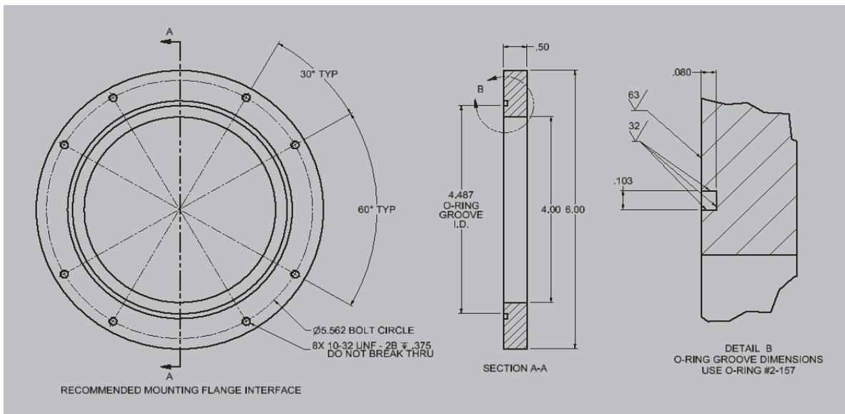
Figure 13 - Cryocooler displacer mechanical interface.
