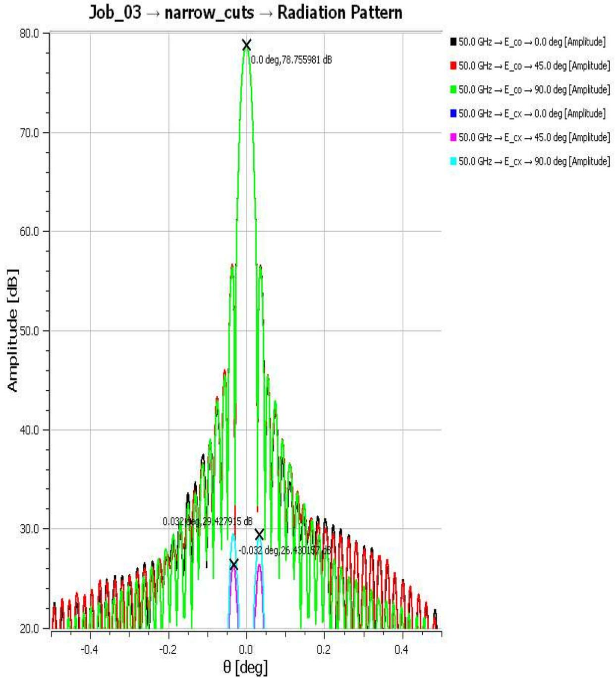
Figure 41 Undistorted Surfaces Beam Pattern 50 GHz
