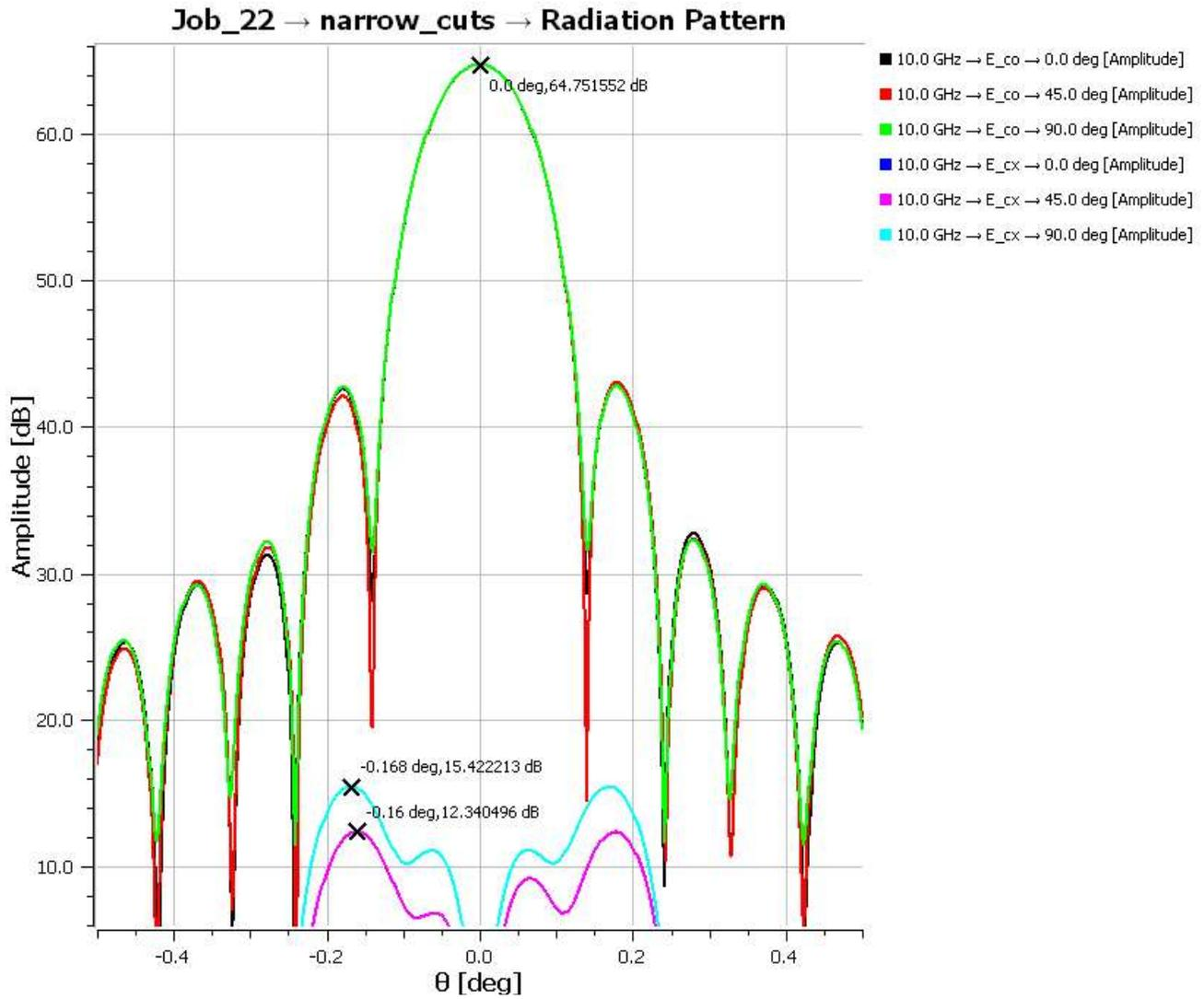
**Figure 42 15° Elevation Angle Gravity Loading Case Beam Pattern 10 GHz**
