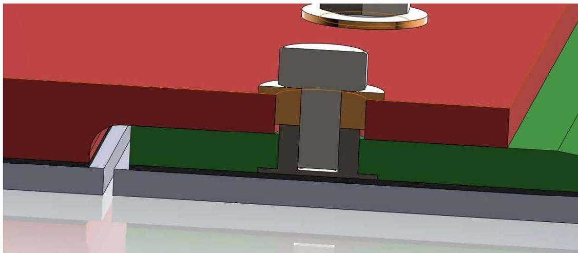
**Figure 20 Cross section through one of the primary surface joining bolts showing the inserts**
