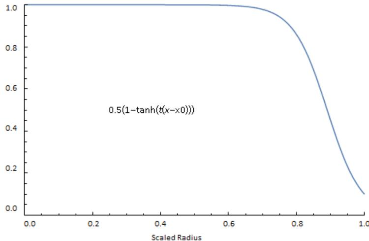
Figure 1 - Aperture illumination relative amplitude.
