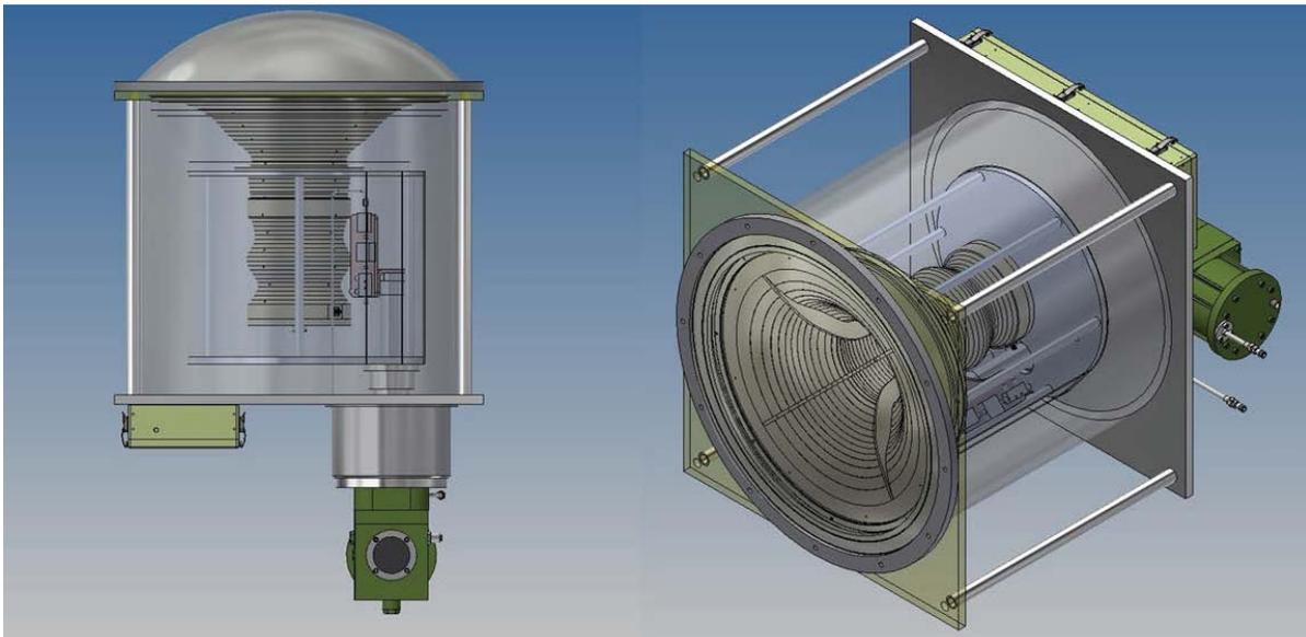
Figure 11 - ngVLA reference receiver Band 1 (cryostat A).
