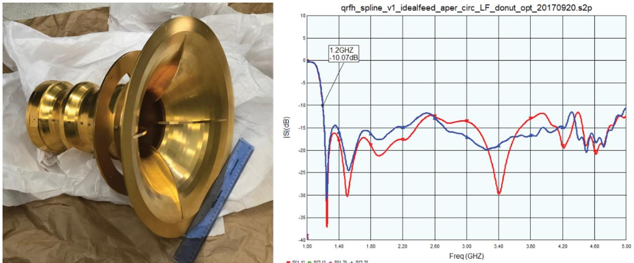
**Figure 4 - Band 1 quad-ridge feed horn prototype (photos courtesy S. Weinreb).**
