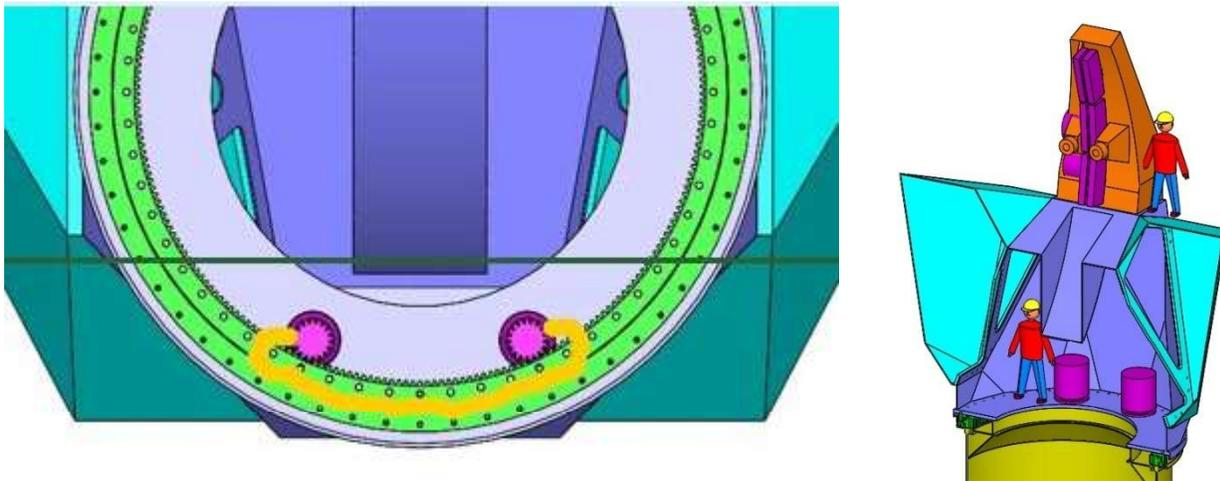
**Figure 32 Azimuth Pinion/Gear Drive**
