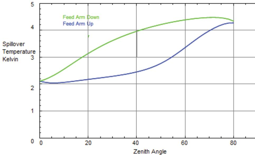
Figure 20 - ngVLA\_6 spillover curve at 5 GHz with corrugated feed horn and SKA noise model.
