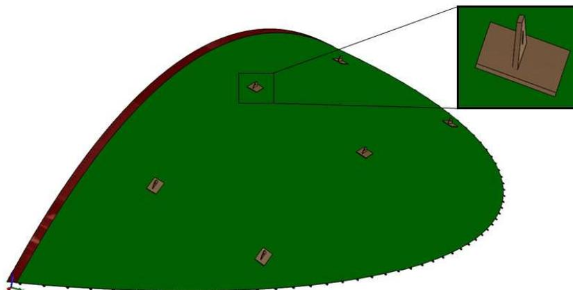
**Figure 21 Lifting points added to one of the 4 primary surface panels**
