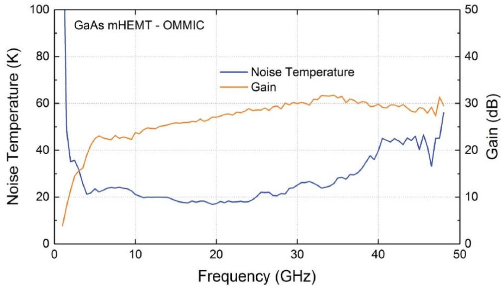
Figure 18 - OMMIC 70 nm GaAs m-HEMT LNA: gain and noise temperature.
