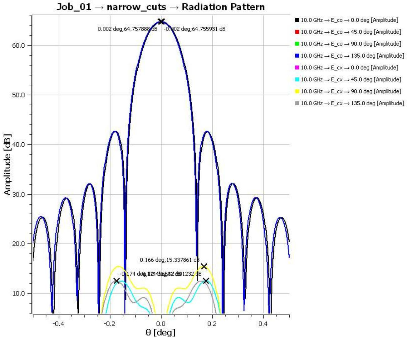
Figure 52 Wind Load Case 2 Beam Pattern 10 GHz
