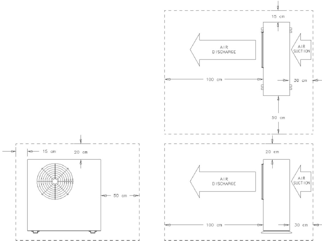
Figure 7 - Compressor space requirements on the antenna platform.
