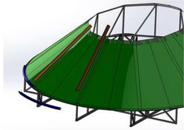
Then the rim beam (shown in blue) and the radial beams (in brown exploded view) are added.
