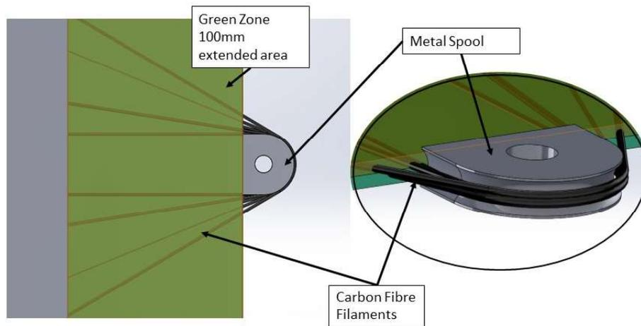
**Figure 7 Primary surface edge adjuster tab concept**
