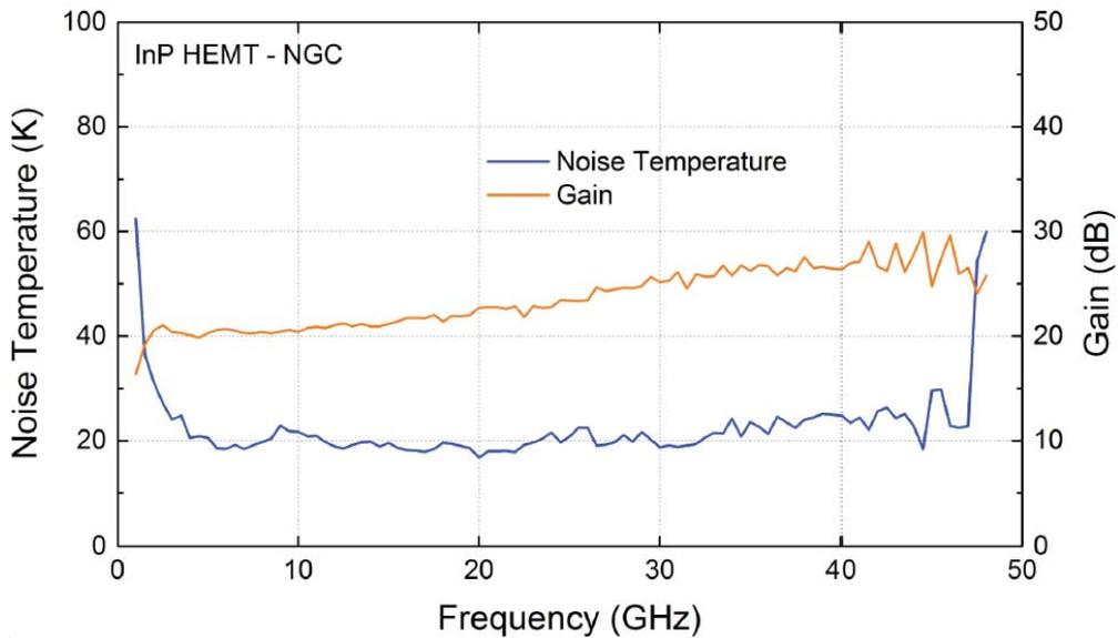
Figure 19 - NGC 35 nm InP HEMT LNA: gain and noise temperature.
