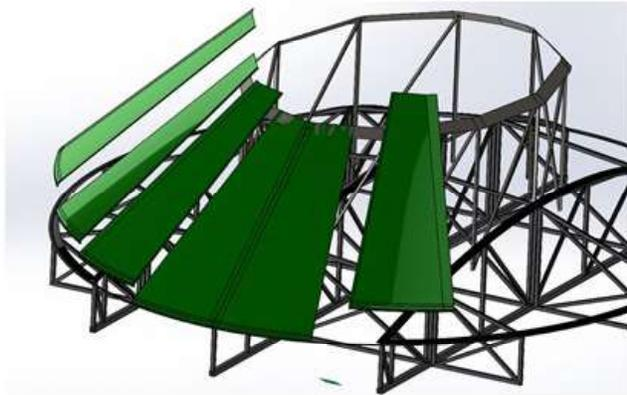
The panels are assembled on the assembly jig. Connecting edges are bonded lap joints.
