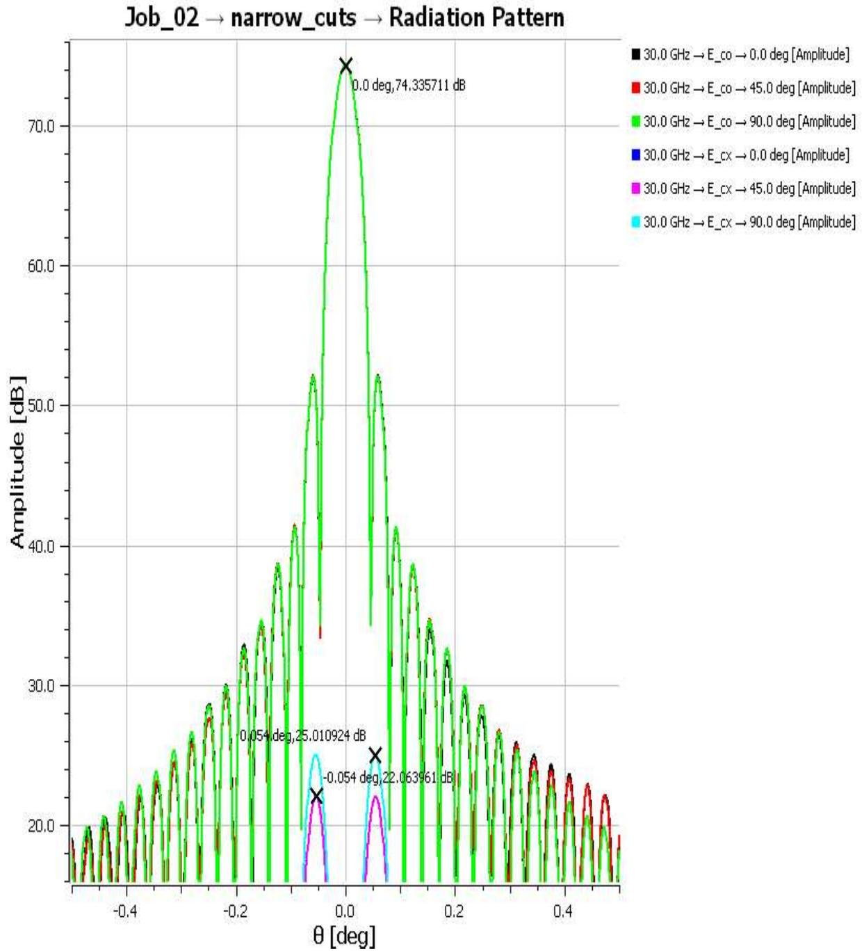
Figure 40 Undistorted Surfaces Beam Pattern 30 GHz
