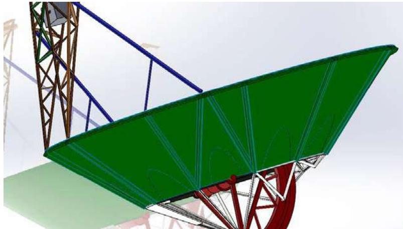
**Figure 16 Stiffening Ribs on Primary Reflector to Support Secondary Support Structure**
