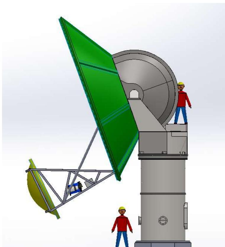
**Figure 11 Complete 6m telescope with mount**
