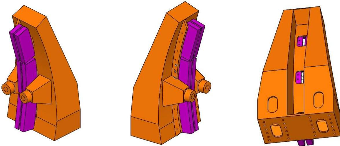
**Figure 26 Elevation Drive Stator Pylon Structure**
