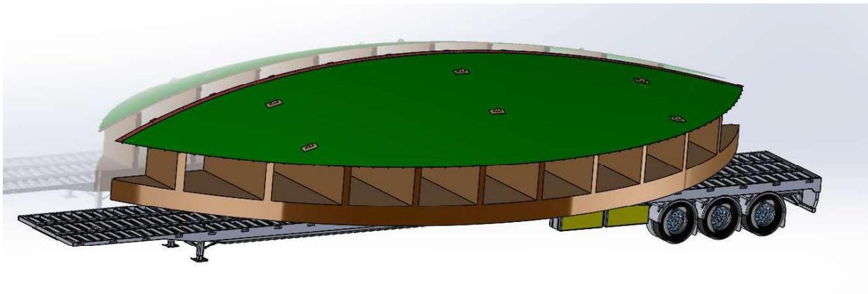
**Figure 23 One of the four primary surface parts on its transport jig and flat deck trailer**
