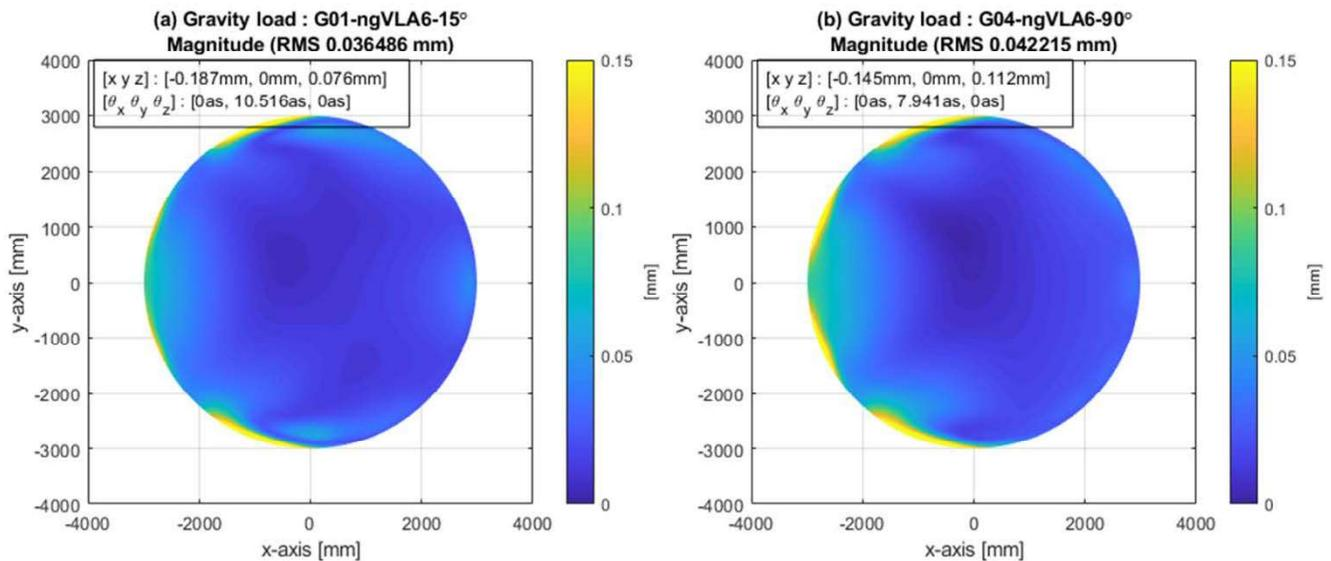
**Figure 20 ngVLA 6m surface RMS error under Gravity load cases (a) 15° and (b) 90° elevation angle.**
