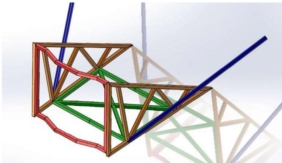
**Figure 10 Secondary and Feed Support Structure for 6m dish**
