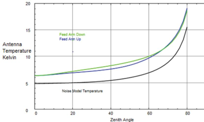
Figure 10 - ngVLA Design #6, tipping curve at 5 GHz with ideal feed and SKA noise model.
