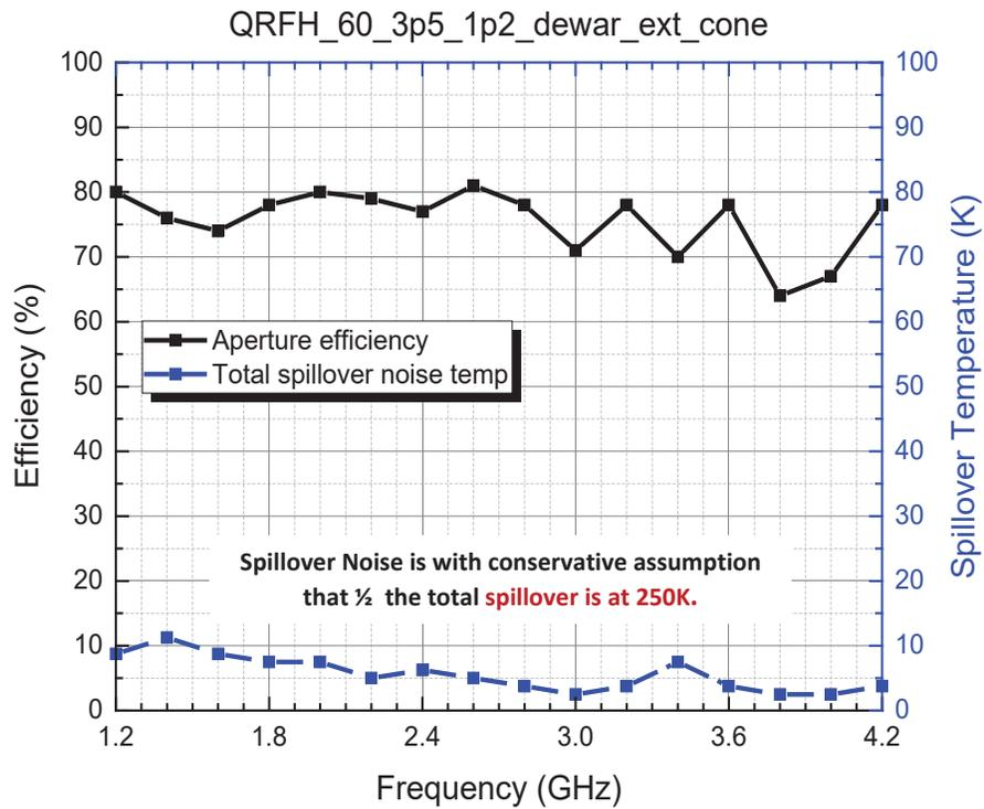
Figure 15 - QRFH cross section and shield cone, with simulated illumination efficiency and spillover noise.
