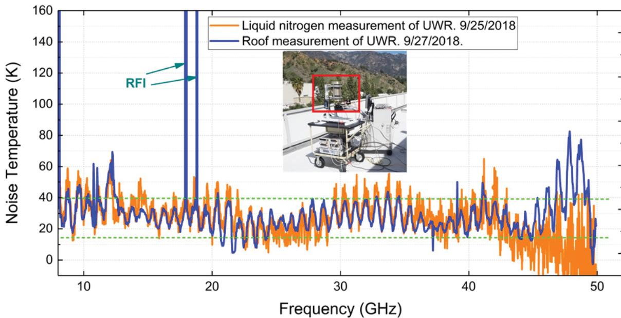
Figure 21 - JPL UWB receiver noise temperature, measured both with an LN2 load and on cold sky.
