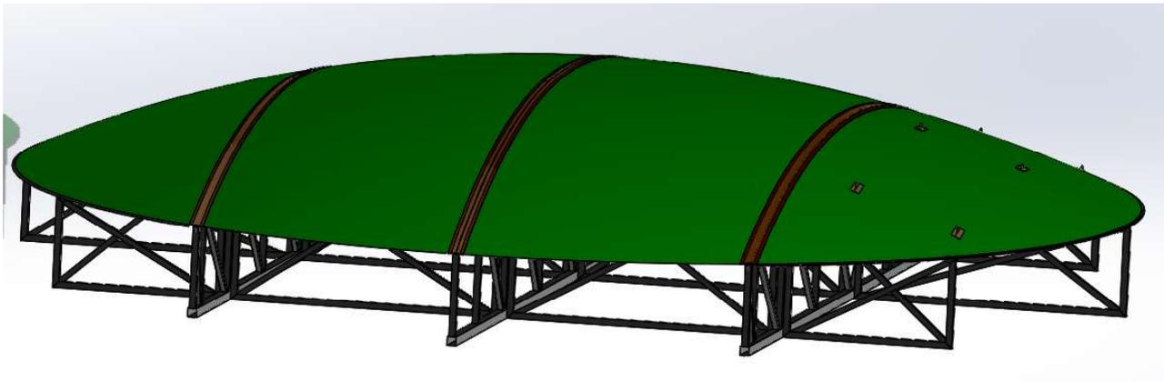
**Figure 22 Assembly jig for the primary surface parts**
