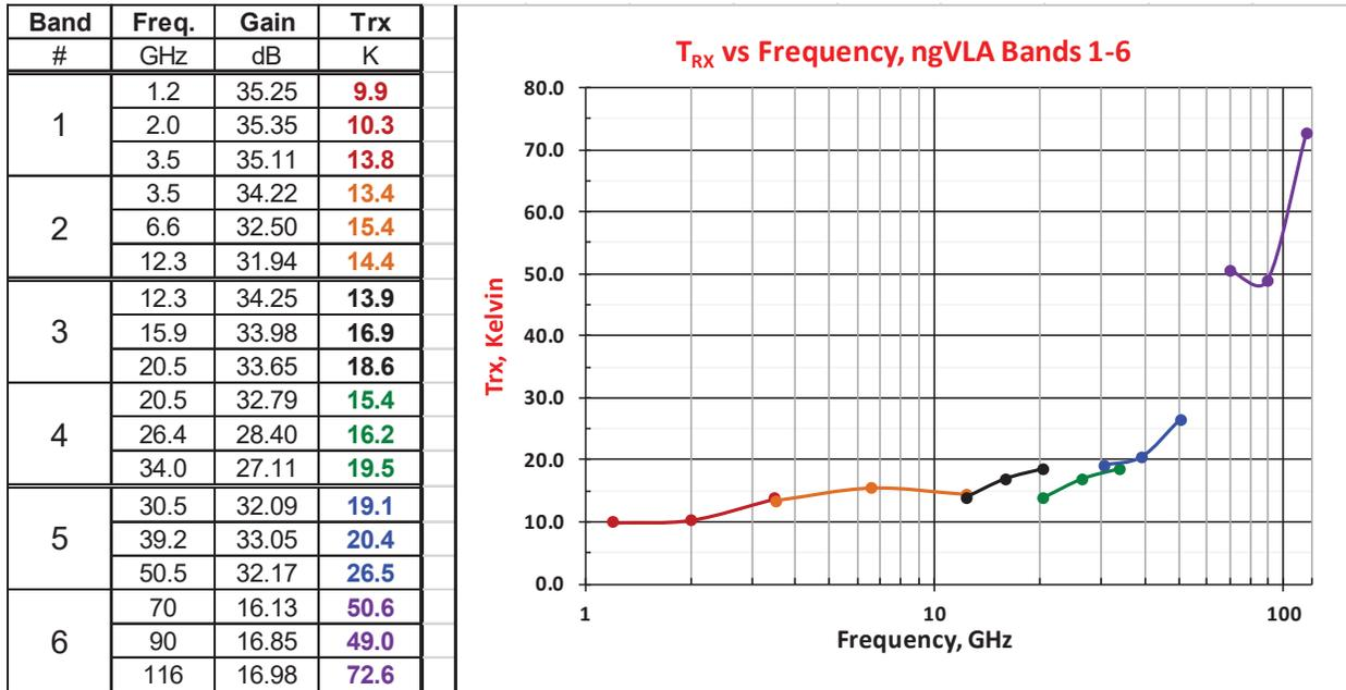
Figure 22 - Plot of receiver noise vs. frequency, Bands 1-6.
