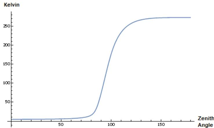
Figure 9 - SKA noise model of brightness temperature at 5 GHz.
