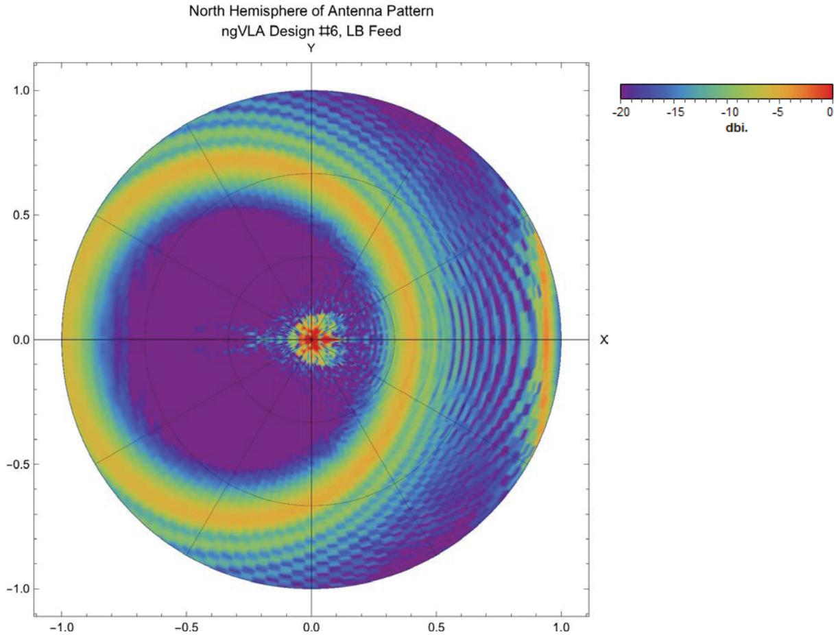
Figure 16 - Unit disk projection of far-field illumination pattern using corrugated feed horn, north hemisphere.
