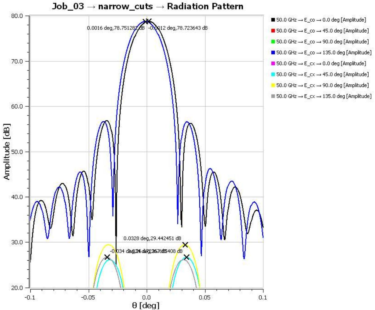
**Figure 51 Wind Load Case 1 Beam Pattern 50 GHz**
