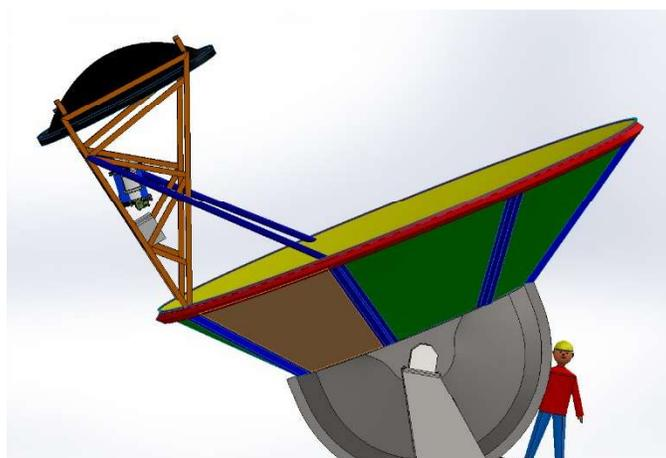
**Figure 9 Stiffening Ribs on Primary Reflector to Support Secondary Support Structure**
