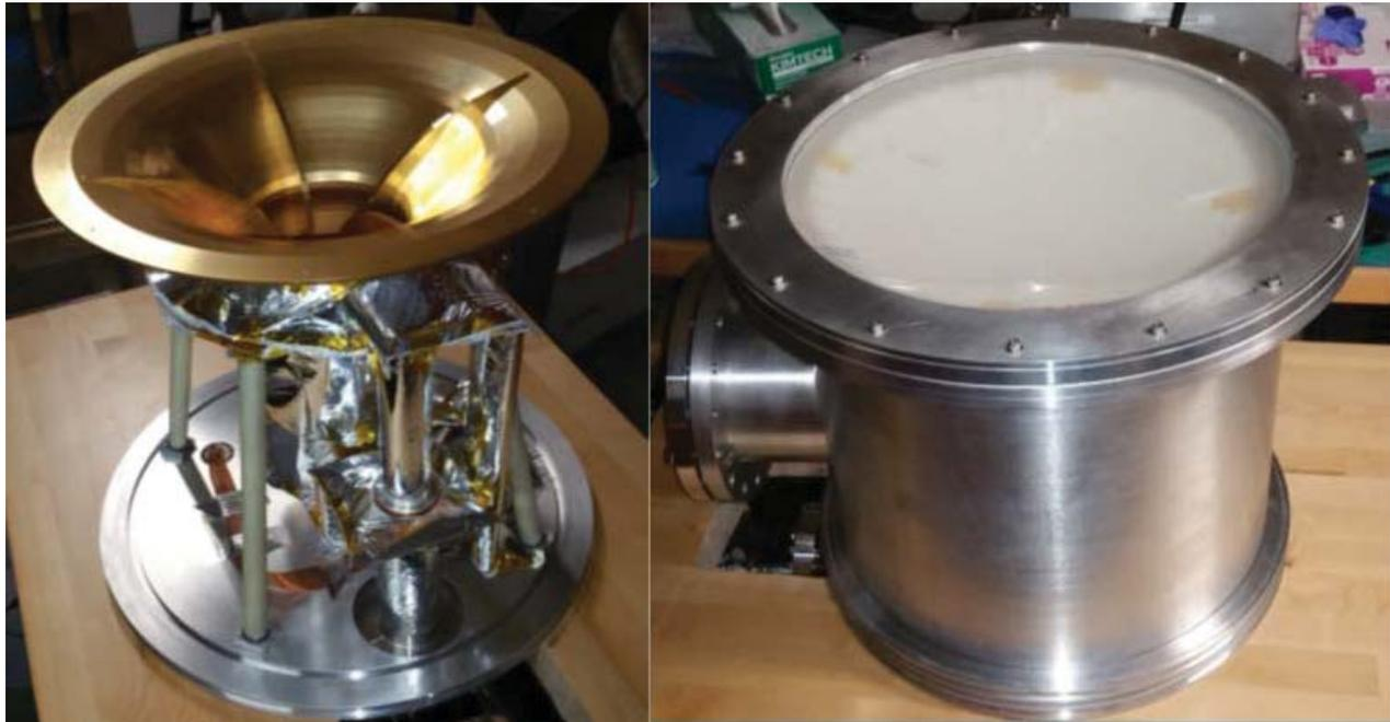
Figure 17 - Caltech/ASU Band I cryostat, open and fully assembled (cryocooler is below tabletop).
