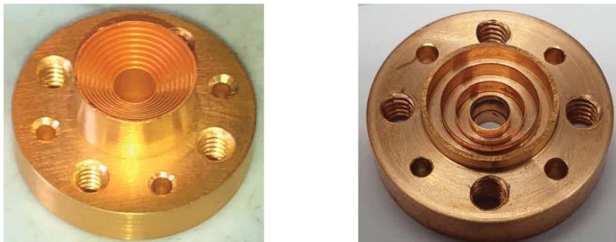
**Figure 6 - Prototype W-band axially corrugated feed horns (left - Baker, right - EMSS).**
