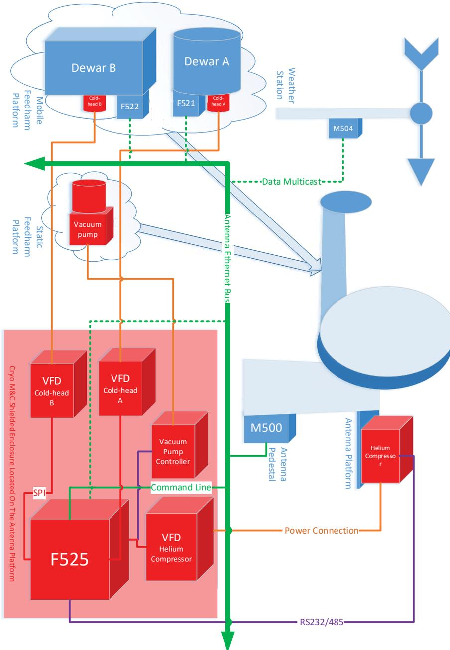
Figure 2 - Cryogenics Monitor and Control subsystem block diagram.
