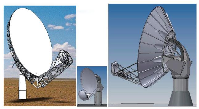
Figure 14 - Left: ngVLA 18-meter antenna design concept prepared by GDMS. Right: 18m antenna concept prepared by NRC. Center: 6m short spacing array antenna concept prepared by NRC.
