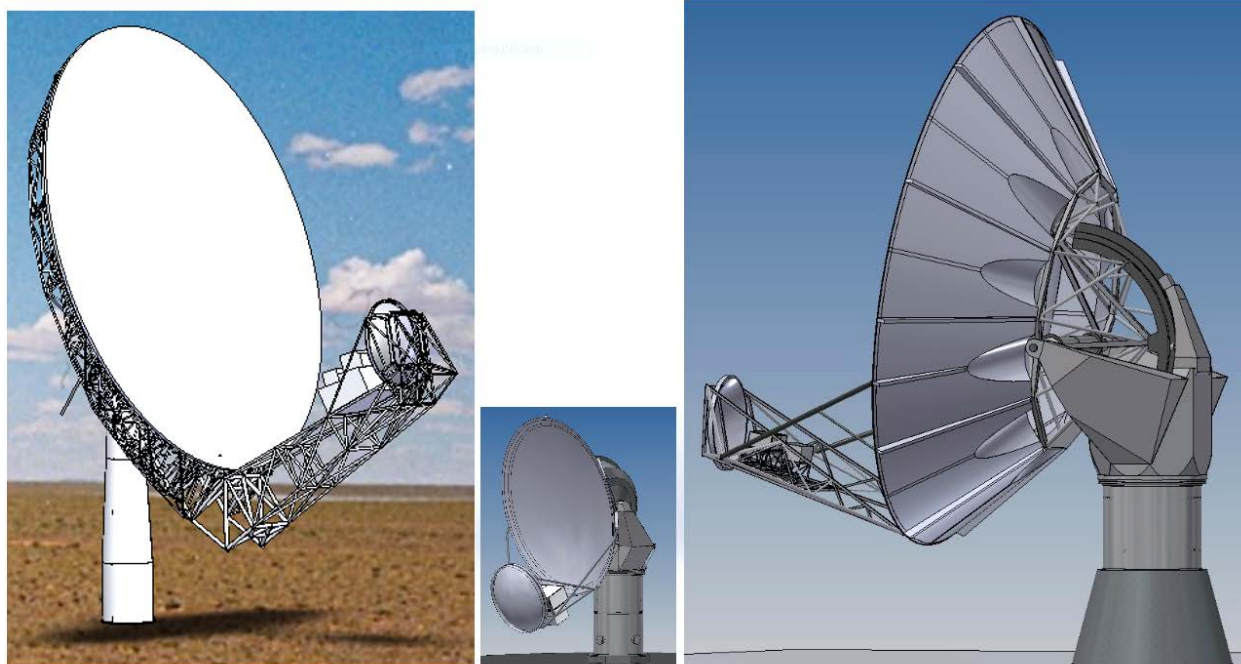
Figure 14 - Left: ngVLA 18-meter antenna design concept prepared by GDMS. Right: 18m antenna concept prepared by NRC. Center: 6m short spacing array antenna concept prepared by NRC.
