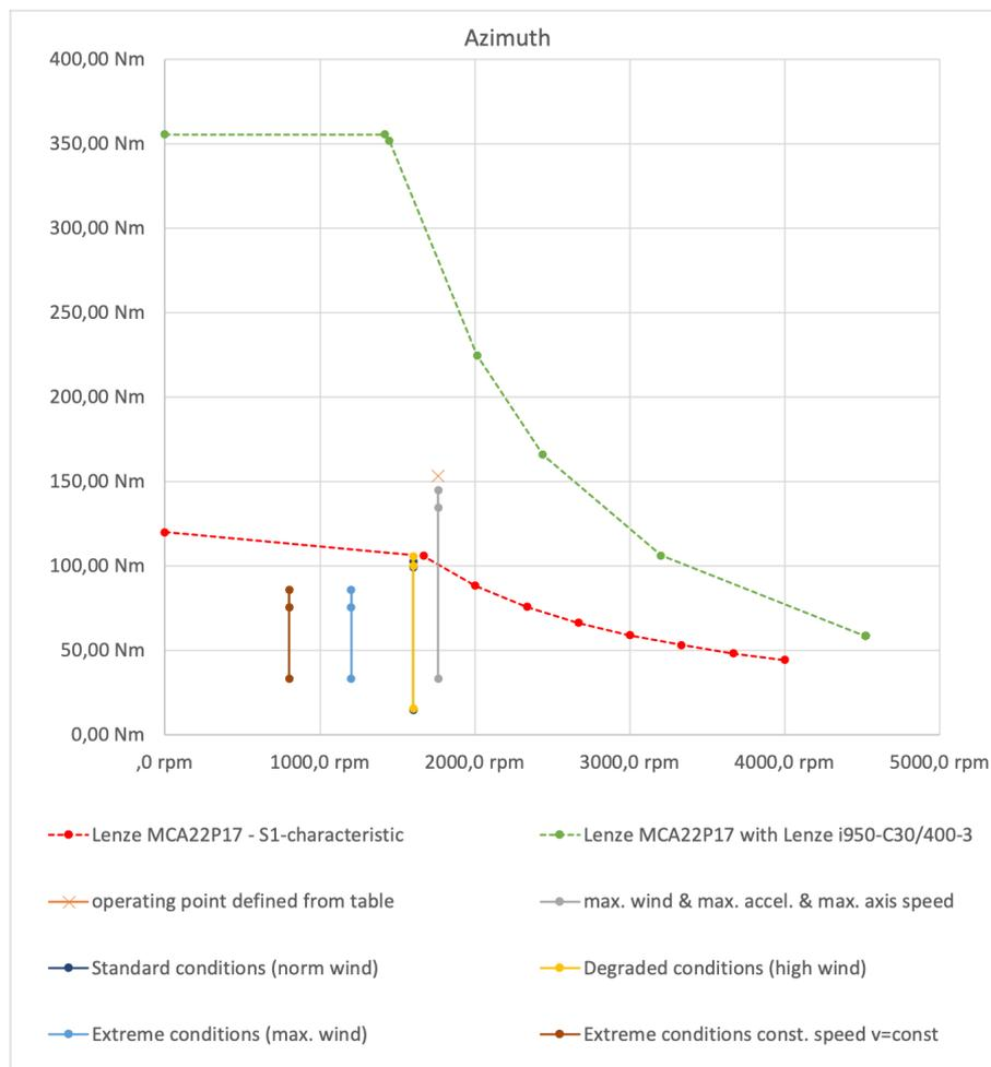
Figure 55 Azimuth torque-over-speed diagram and operating points of drive system by Lenze, the gearbox ratio is changed to 720:1
