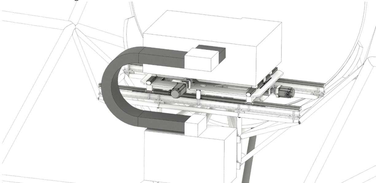
Figure 25 Feed Indexer Actuator Overview
