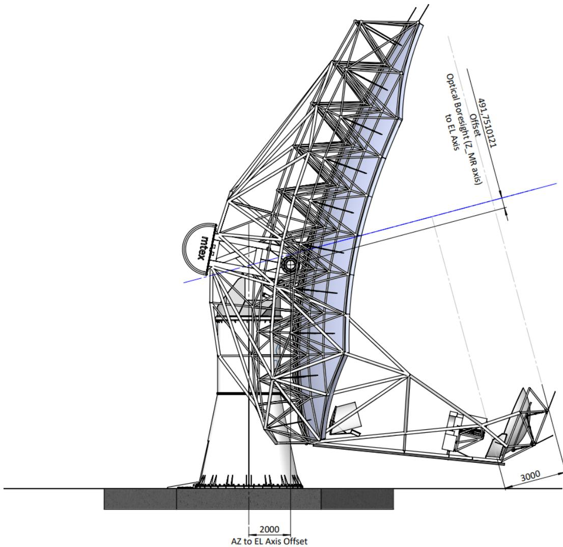
Figure 2 Offset Optical Reflector Axis to parallel EL-Axis
