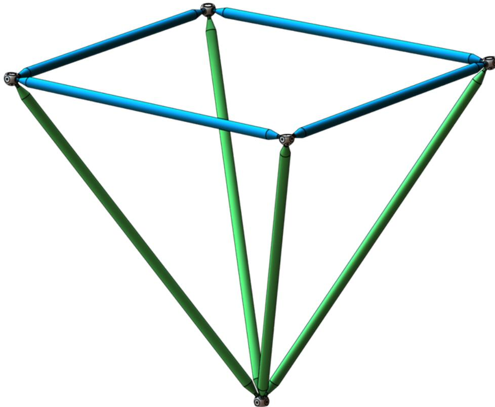
Figure 11 Sample of Octahedron Main Reflector Segment
