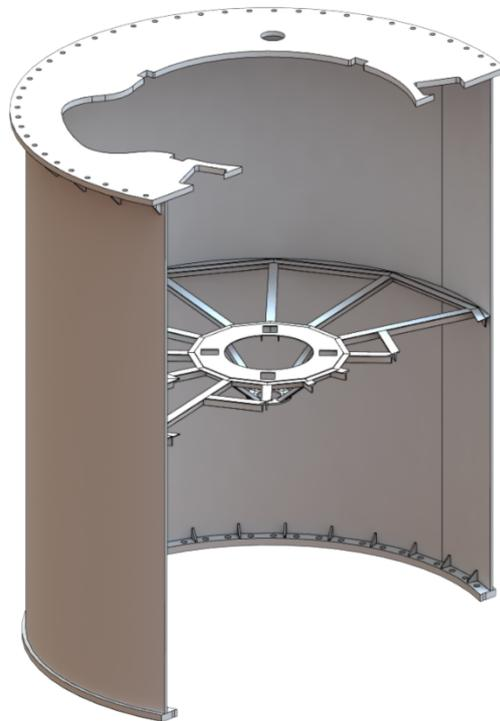
Figure 39 Upper Pedestal Steel Structure (Cross Section)
