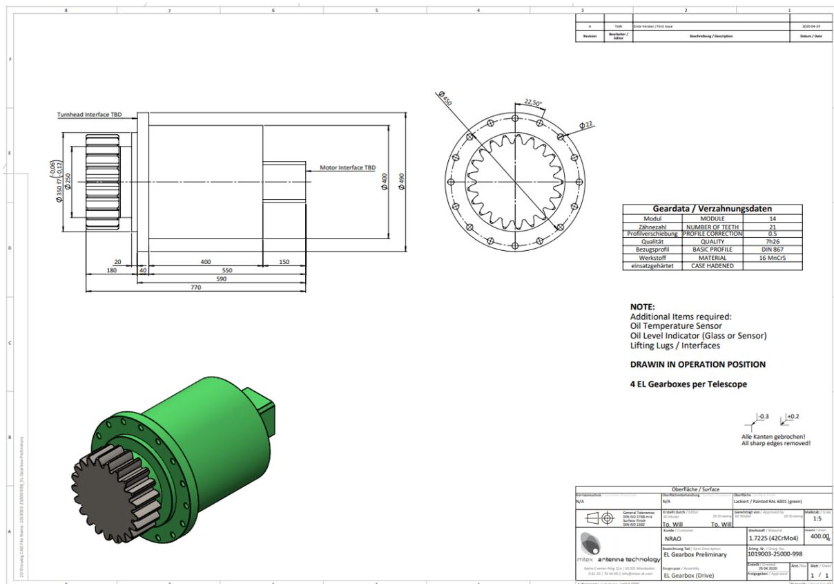
Figure 51 Elevation Gearbox Preliminary Drawing
