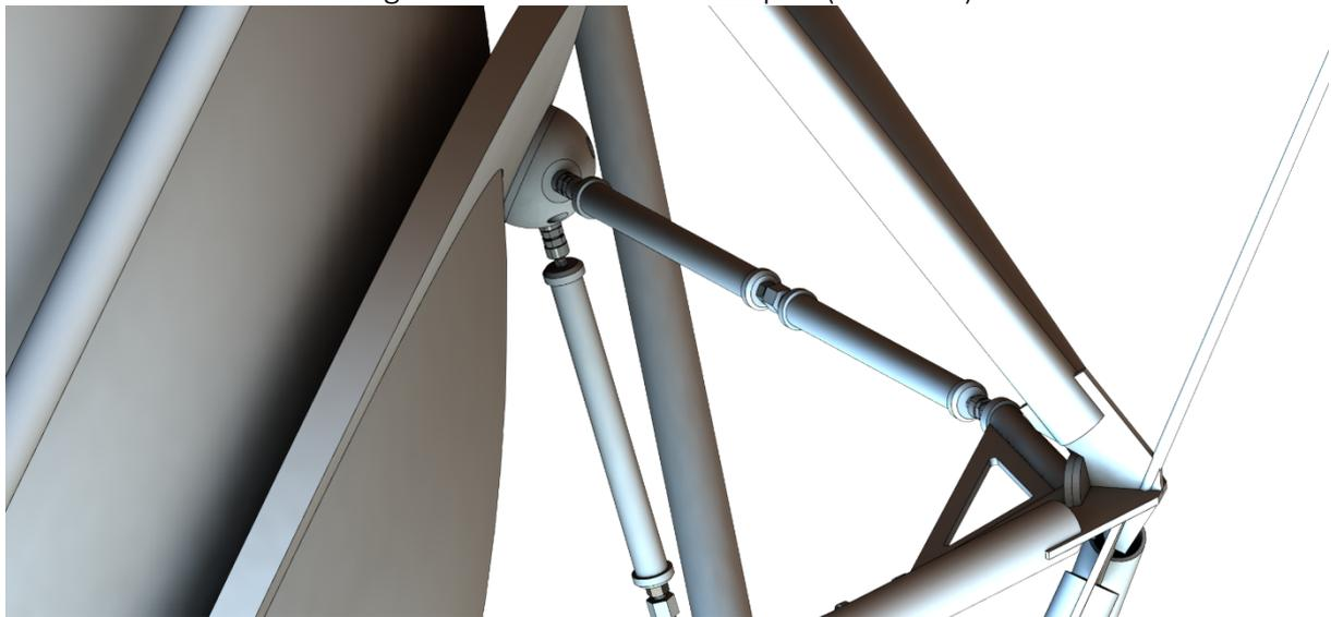
Figure 31 Sub-reflector Hexapod (detail view)
