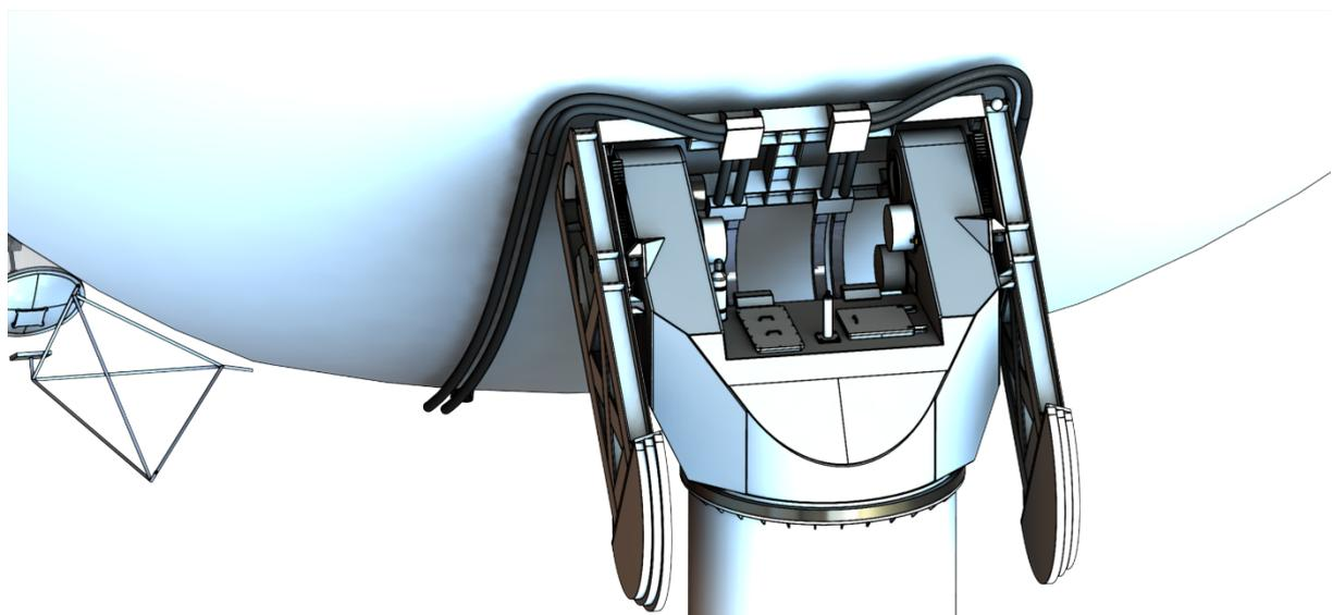
Figure 66 Main Reflector Cable Routing (without BUS)
