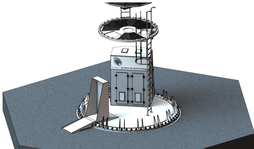
Figure 38 Lower Pedestal without Back-End Rack
