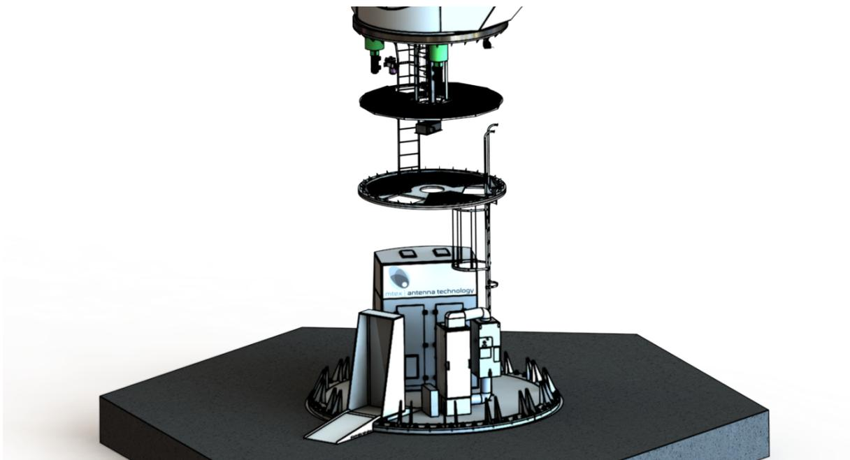
Figure 35 Pedestal without outer steel walls
