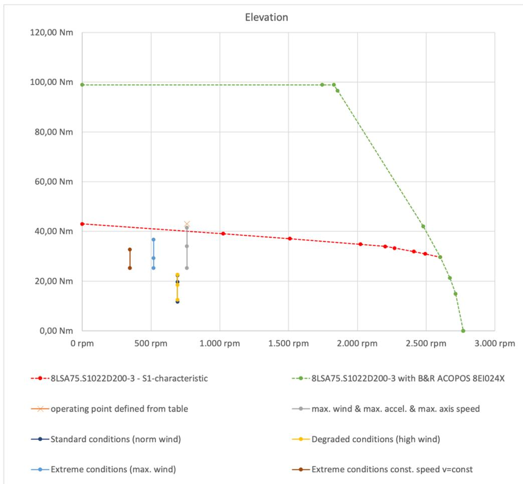
Figure 56 Elevation torque-over-speed diagram and operating points of drive system by B&R
