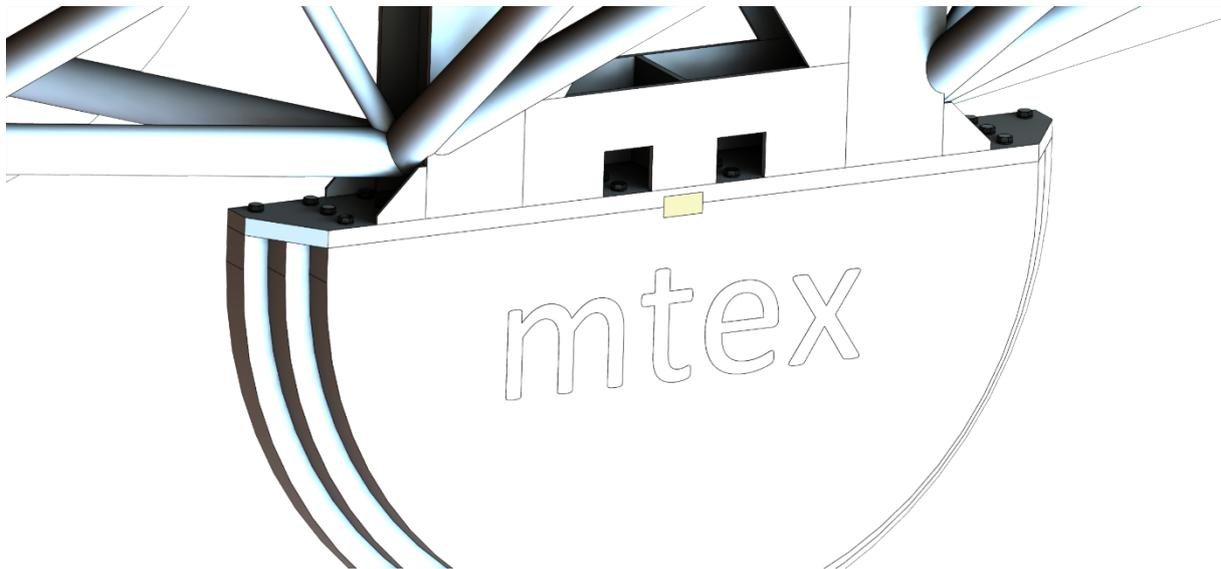
Figure 33 Counterweights mounted to welded structure
