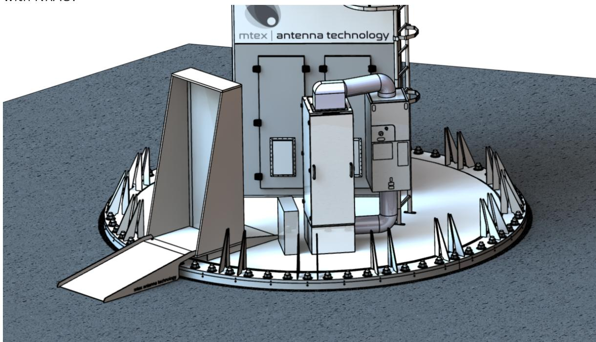
Figure 118 Back-End Equipment inside lower pedestal
