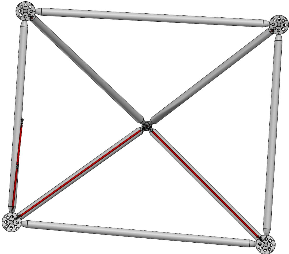
Figure 18 Arrangement of planar and rotation adjusters
