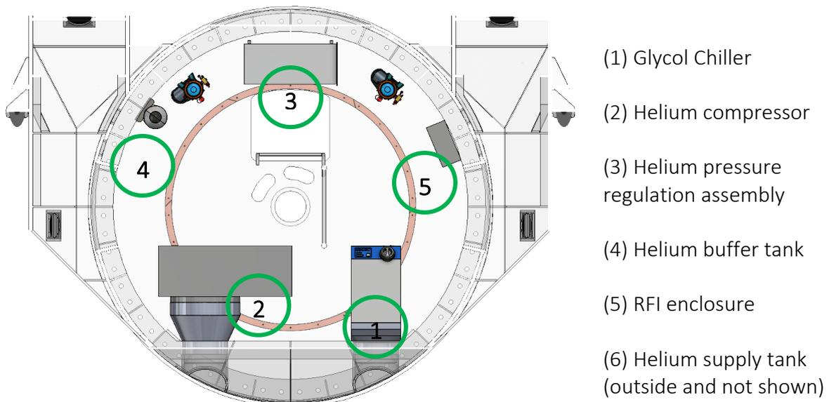
Figure 117 Environmental Control Equipment Locations
