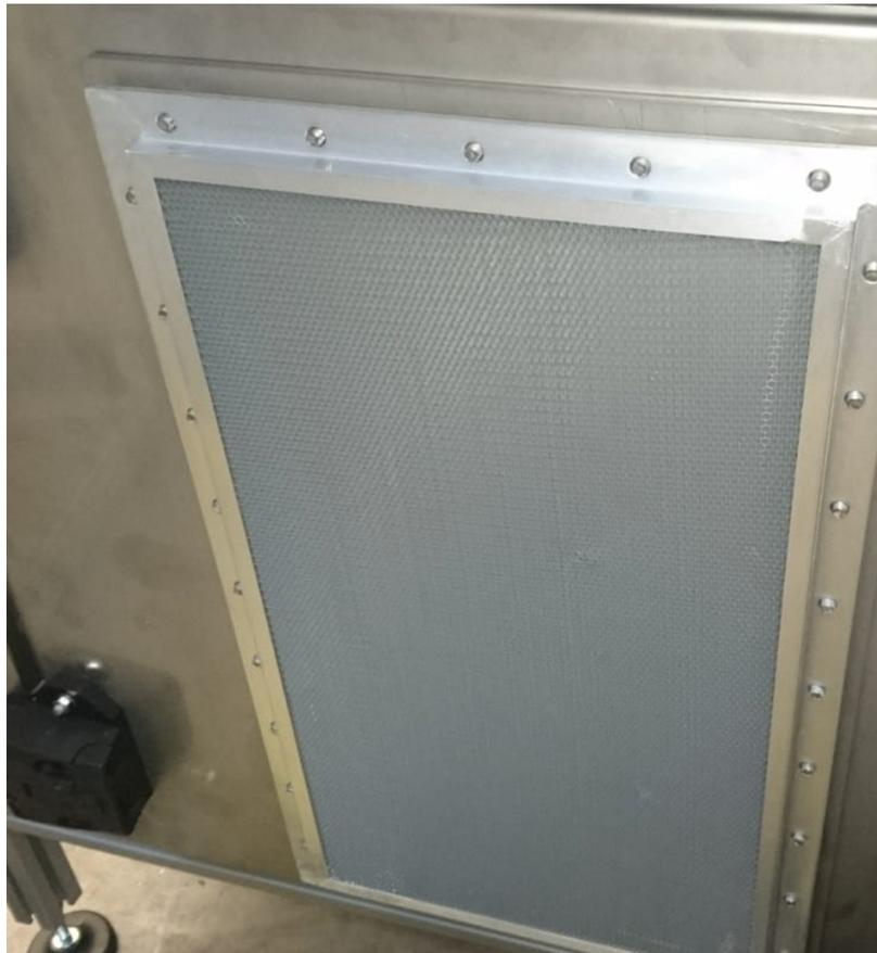
Figure 76 Door/Roof Filter during EMI Tests
