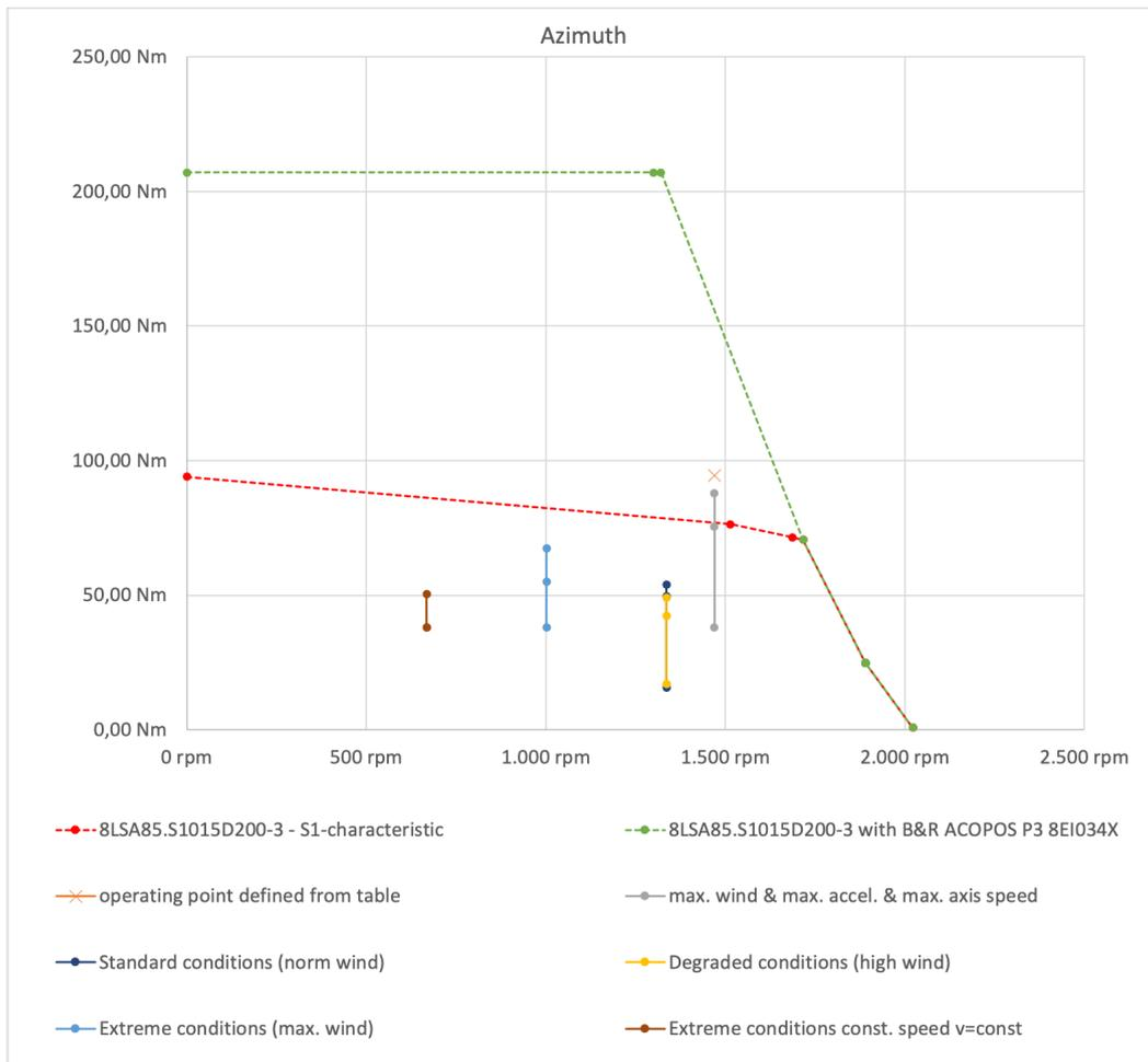
Figure 54 Azimuth torque-over-speed diagram and operating points of drive system by B&R
