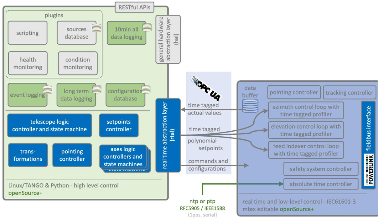
Figure 84 Details of the software structure ACU and real-time PLC
