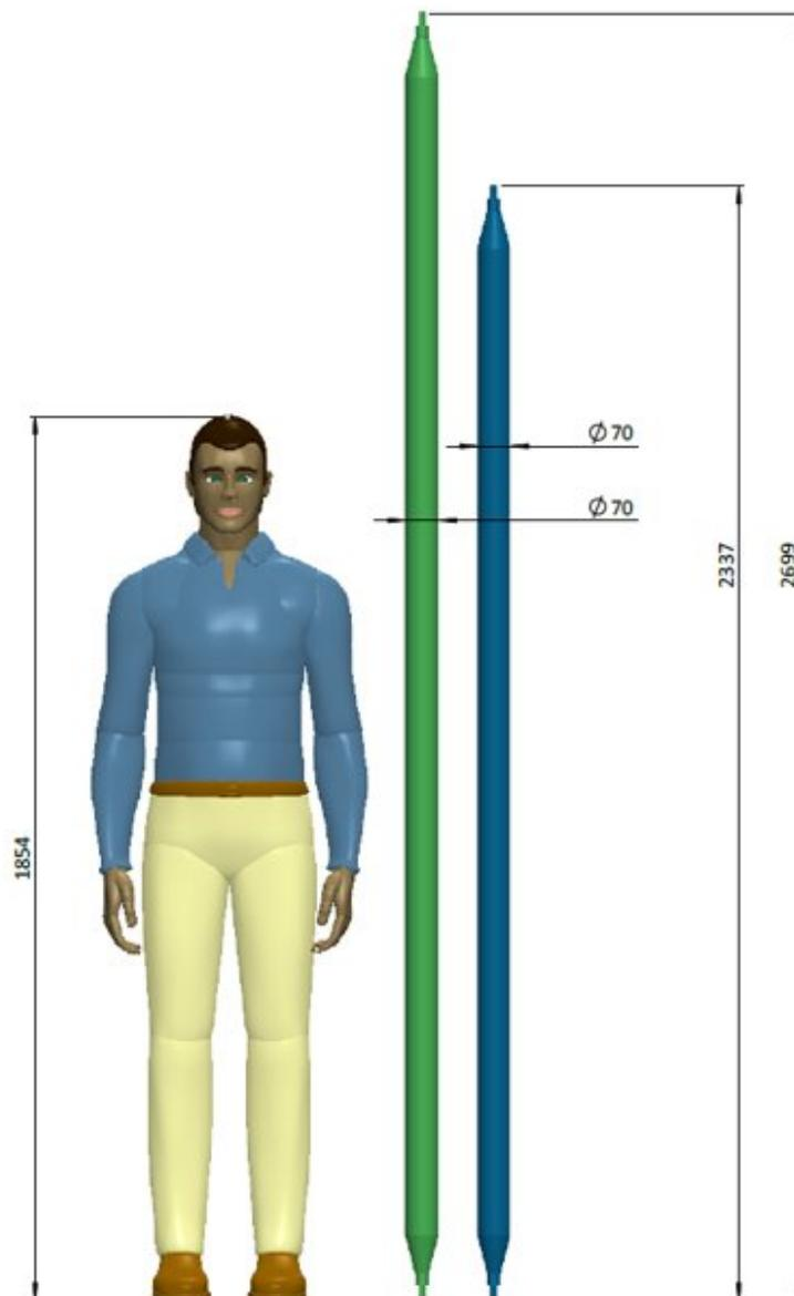
Figure 12 Typical Tube Length (space truss green / upper chord blue)
