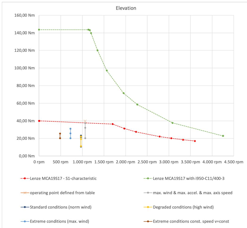
Figure 57 Elevation torque-over-speed diagram and operating points of drive system by Lenze, the gearbox ratio is changed to 1345:1
