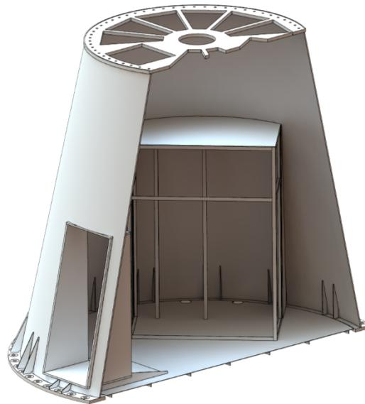
Figure 37 Lower Pedestal Steel Structure (Cross Section)
