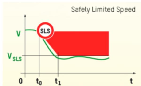
Figure 109: Safe Limited Speed, SLS
