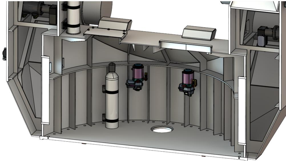
Figure 59 Grease Pump Location of EL ALS (inside Turnhead)
