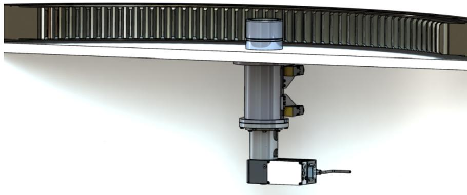
Figure 62 Azimuth Stow Pin
