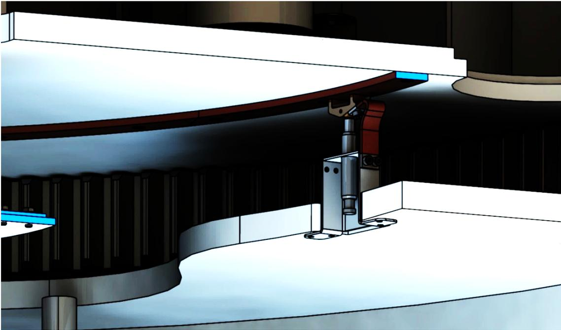
Figure 61 AZ Bearing Lightning Protection
