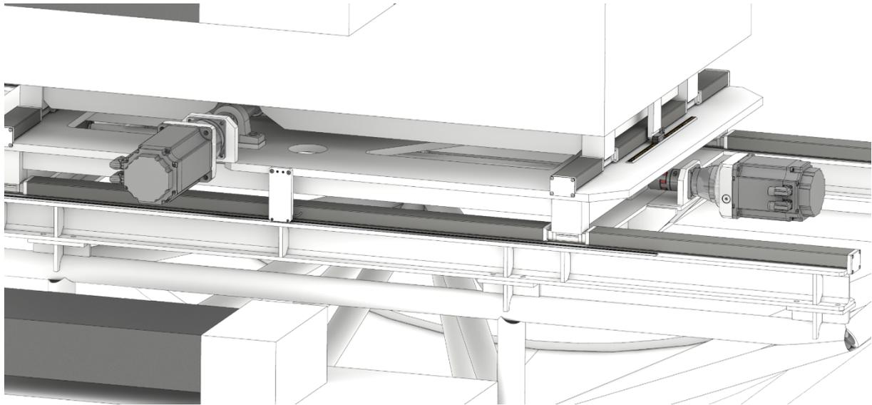
Figure 26 Feed Indexer Actuator (detail view)
