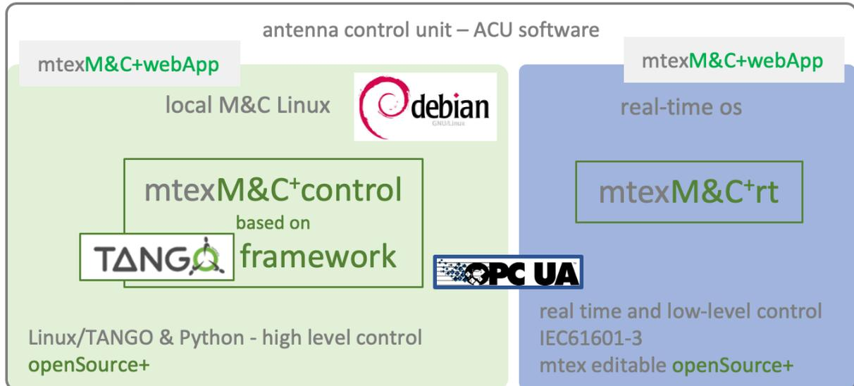
Figure 83 Software ACU and real-time PLC concept
