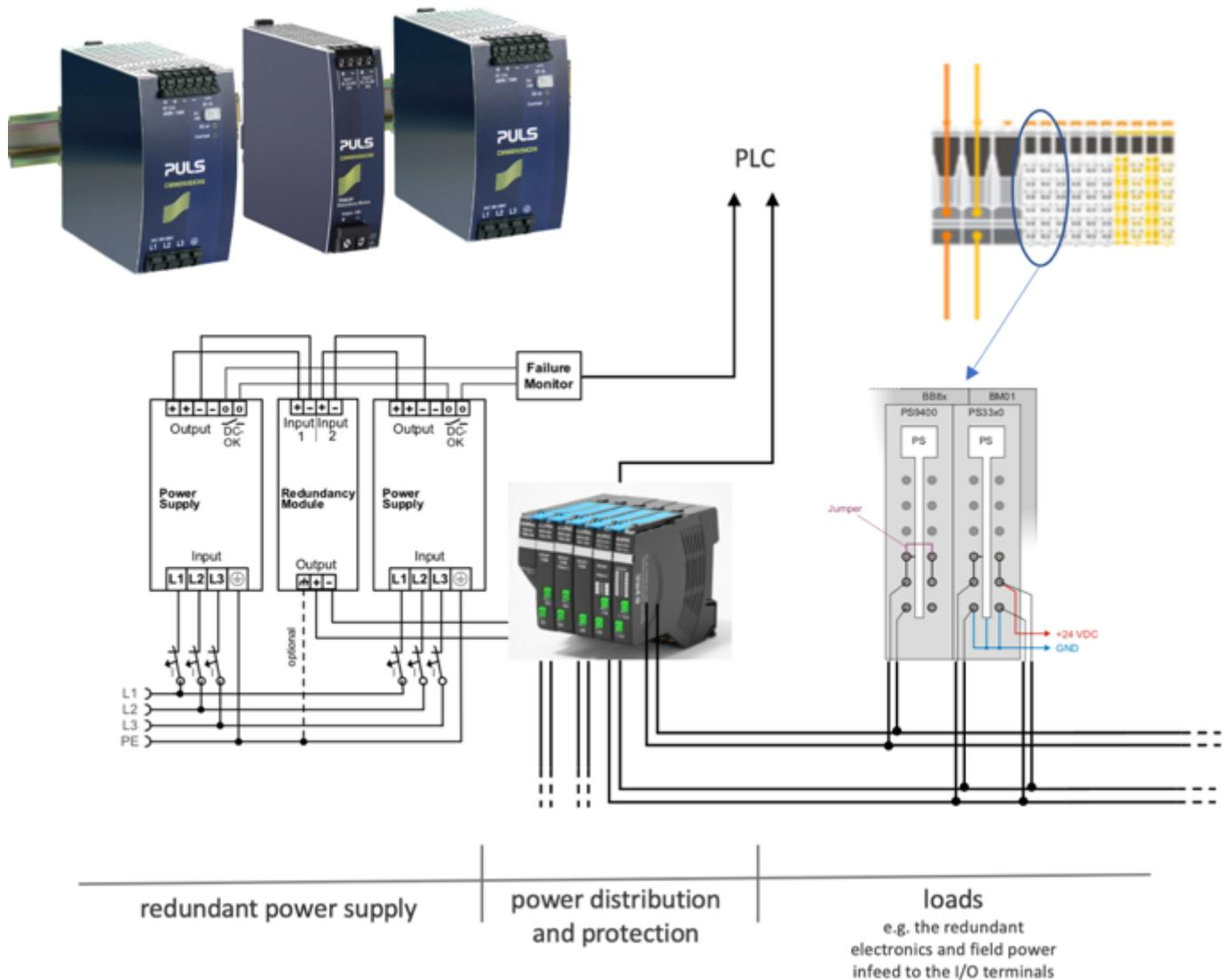
Figure 92 Redundancy concept for 24VDC power supply and distribution to loads
