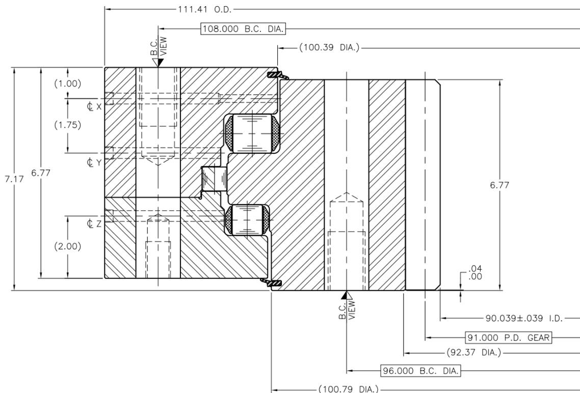
Figure 43 Three-Row-Roller Bearing (Sample, dimensions not applicable to ngVLA)
