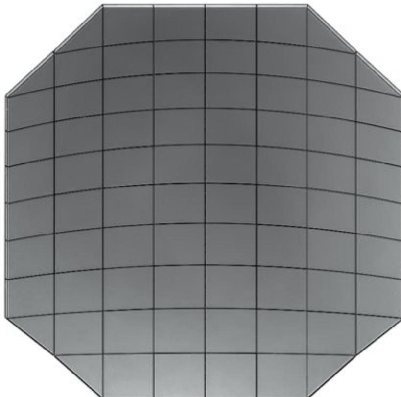
Figure 21 Main Reflector Panel Layout
