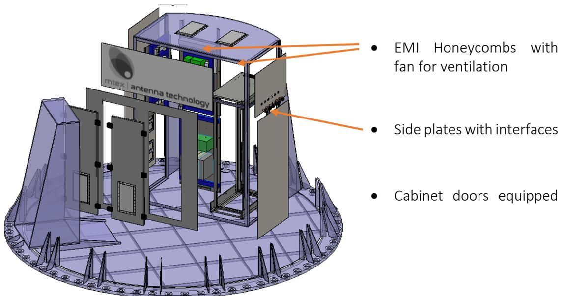
Figure 78 Details of the mtex EMI enclosure
