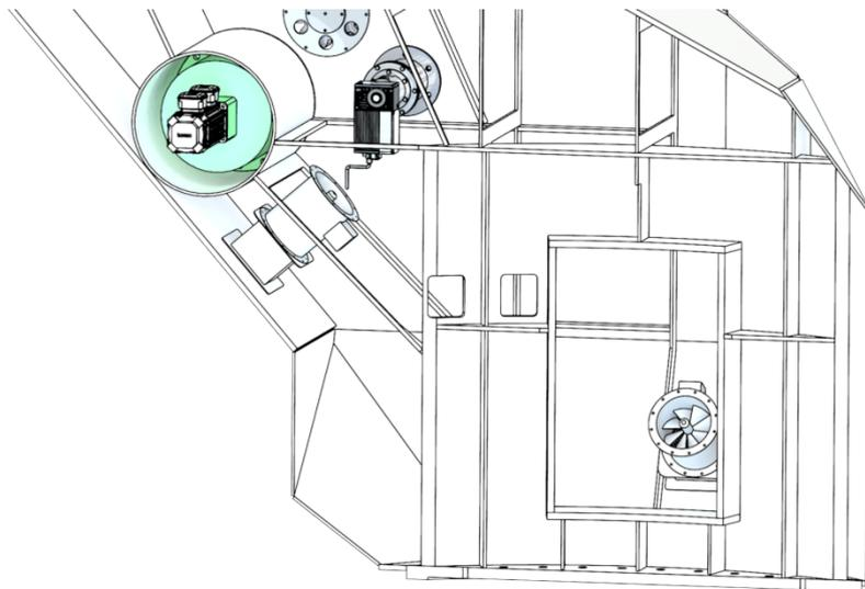
Figure 74 Active Ventilation System (Turnhead, right arm)
