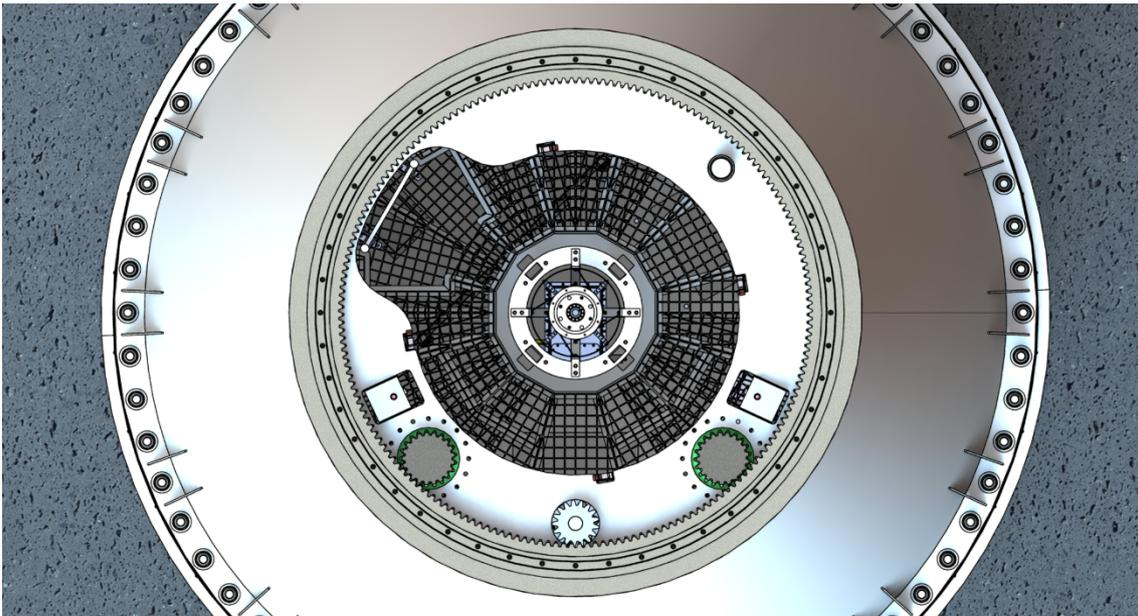
Figure 48 Azimuth Drive Arrangement
