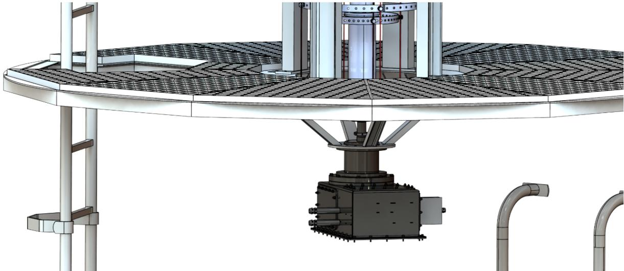
Figure 79 Azimuth I/O Box mounted to Maintenance Platform
