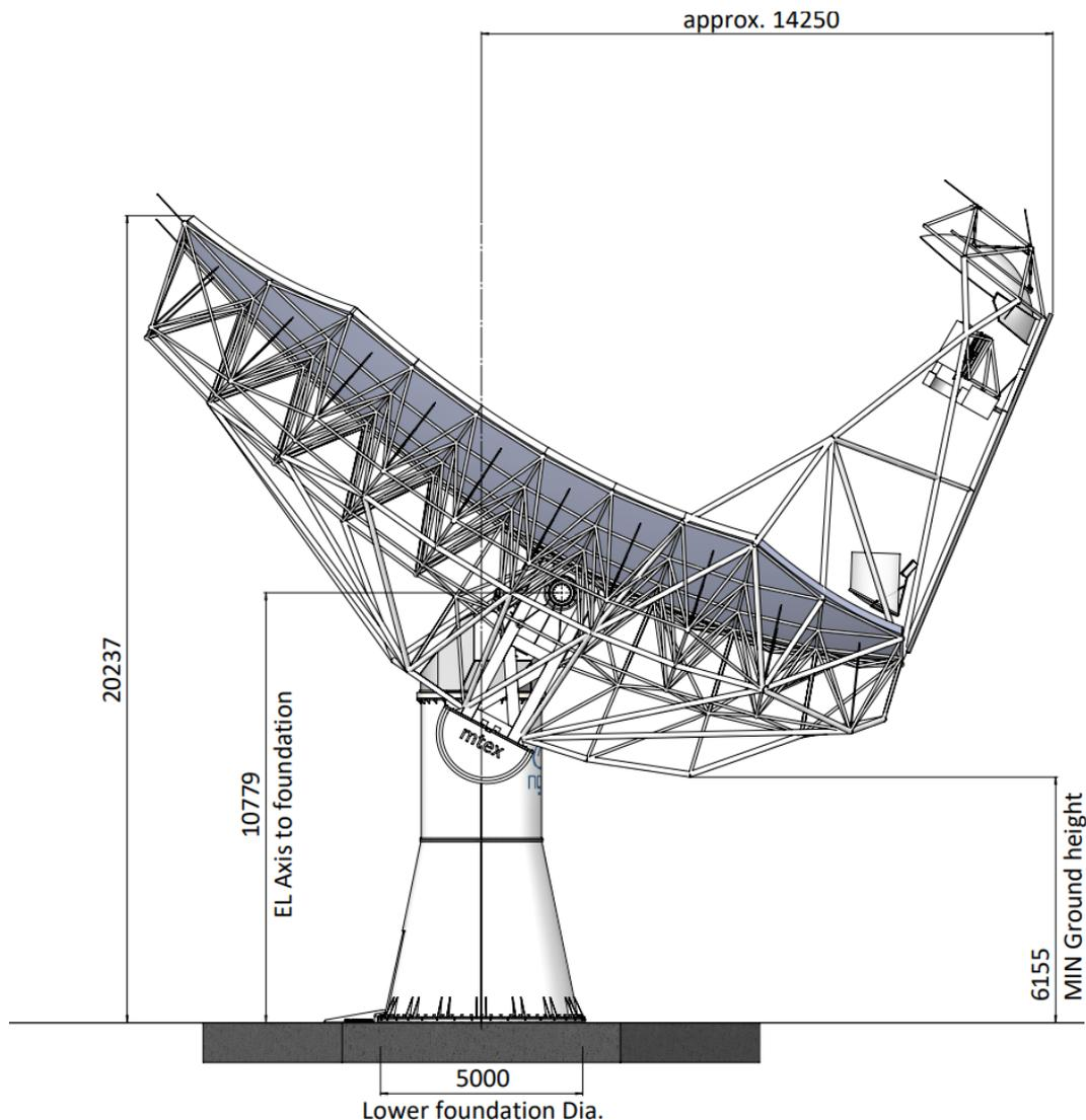
Figure 7 Antenna Main Dimensions (EL 88deg)
