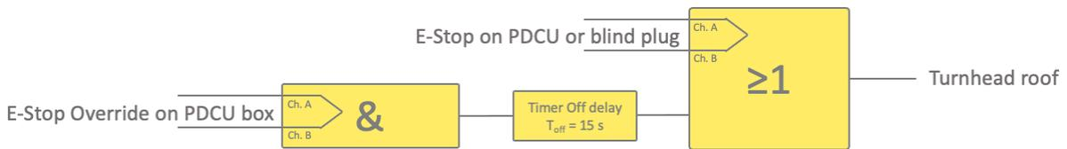
Figure 101: PDCU E-Stop override when connecting/disconnecting PDCU
