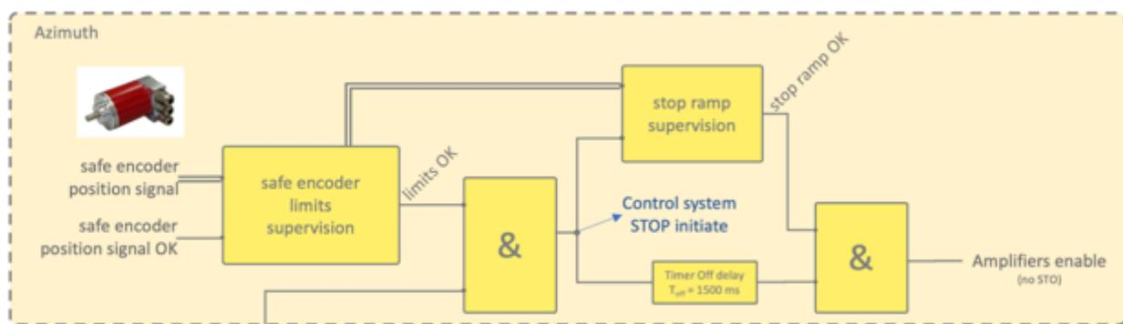
Figure 103: Azimuth motion limits
