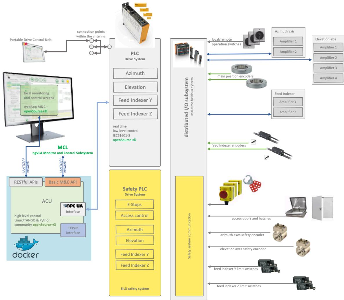
Figure 88: Servo System hardware context
