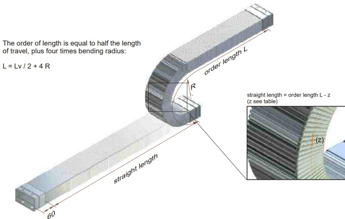
Figure 68 Sample of Steel Tube Cable Loop
