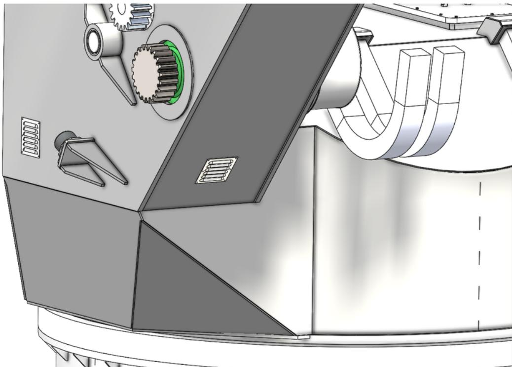
Figure 72 Air Outlet Louvers at Turnhead
