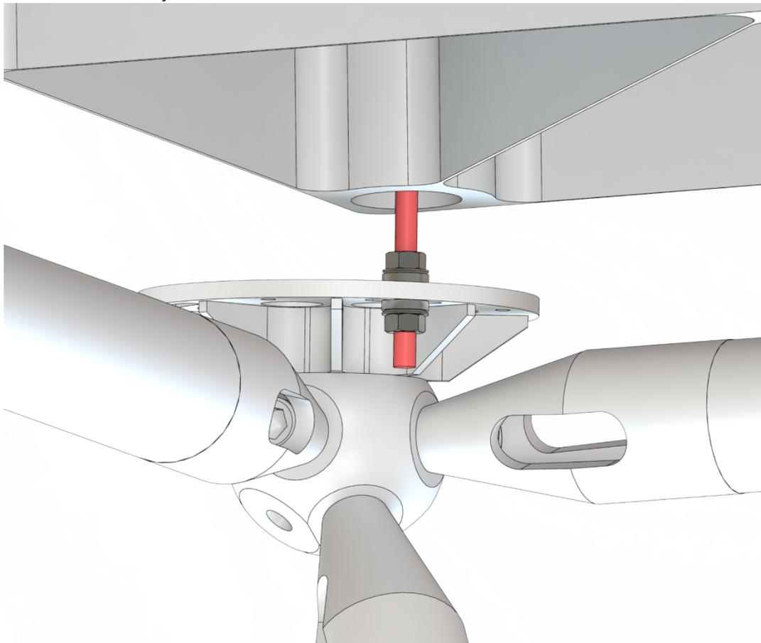
Figure 17 Sample of Panel Adjuster (Corner)
