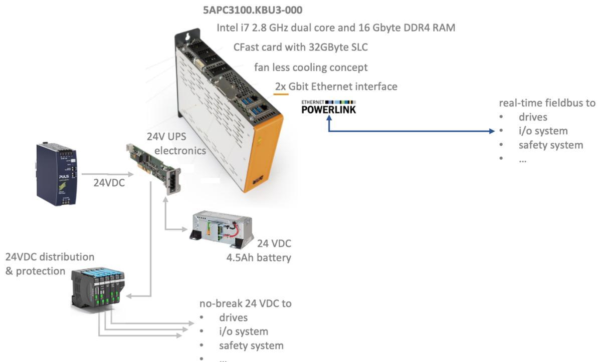
Figure 91: Drive system PLC
