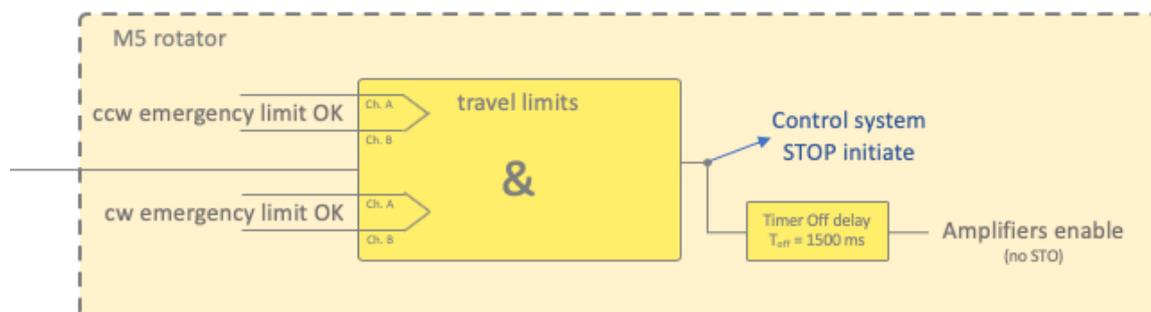
Figure 102: Standard limit switch for travel range
