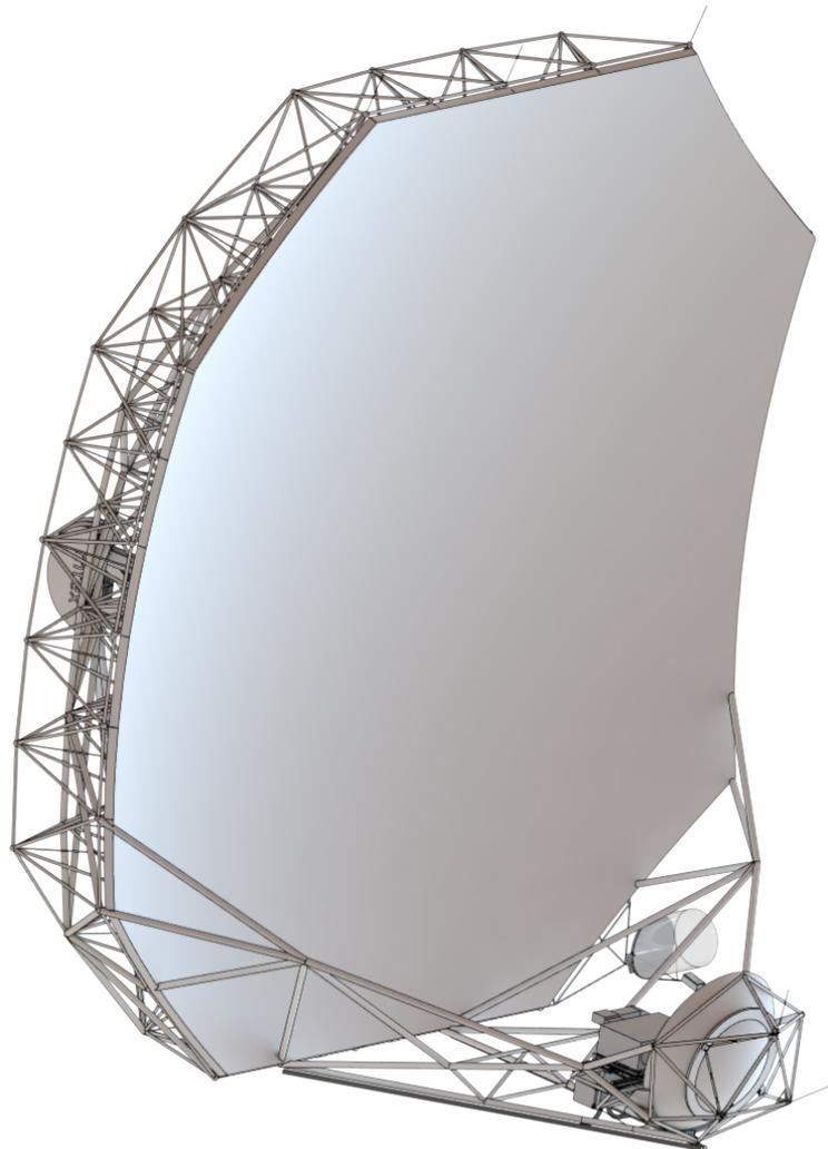
Figure 10 Reflector System (front-iso view)
