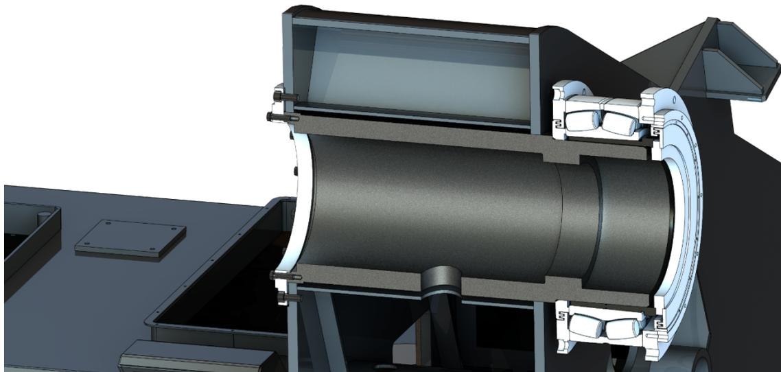
Figure 46 Elevation Bearing Assembly (Cross Section, Left Side)
