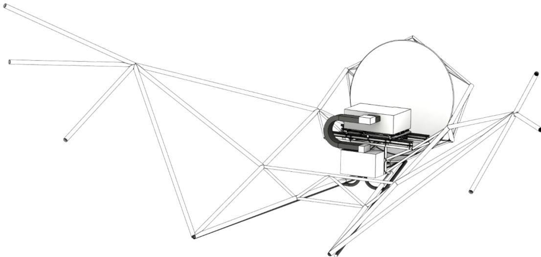
Figure 23 Feed Arm with Equipment
