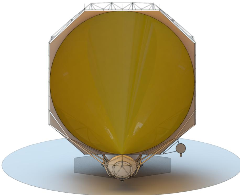
Figure 4 Antenna optics (view along optical axis into reflector)
