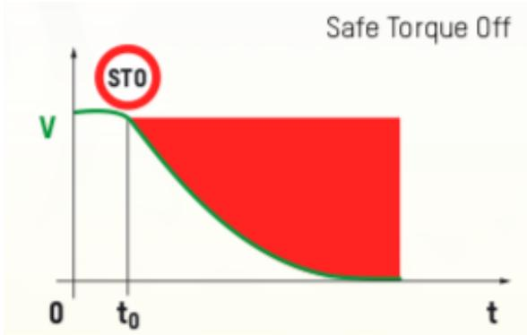
Figure 104: Safe Torque Off, STO
