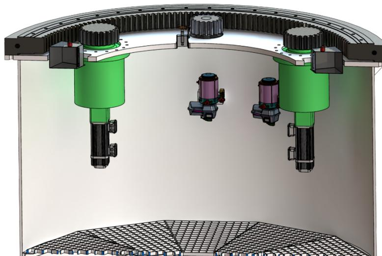
Figure 58 Grease Pump Location of AZ ALS (inside upper pedestal)
