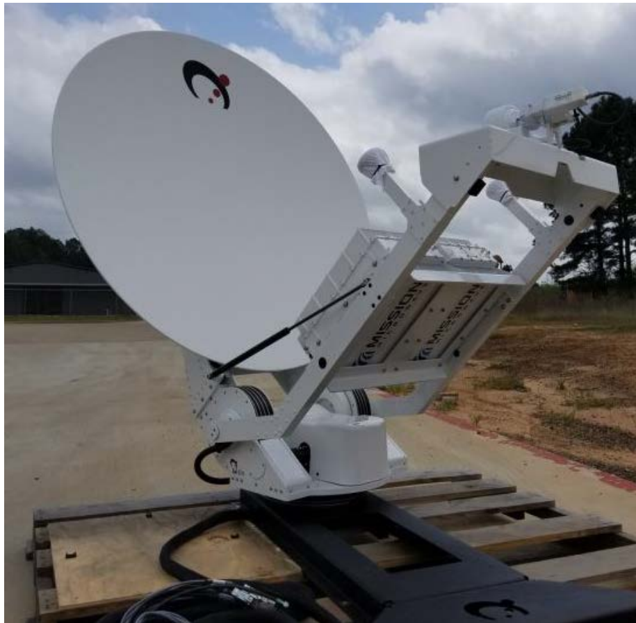
Figure 3: Sat-Lite Technologies Model I41 I Peloris Class motorized 1.45 m vehicle-mount antenna.
