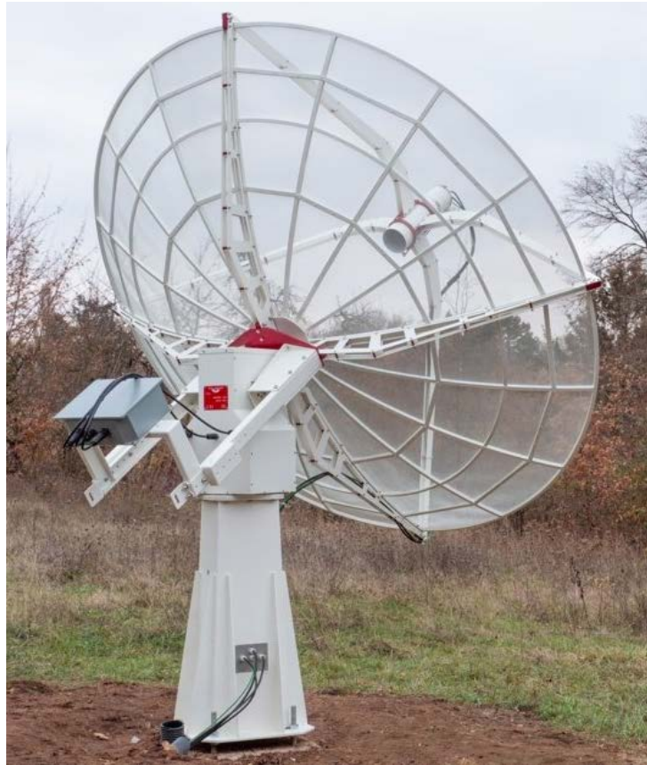
Figure 4: R2S SPIDER 300A 3m telescope with C106-HEAVY pier on concrete base and GS-100 tracker.
