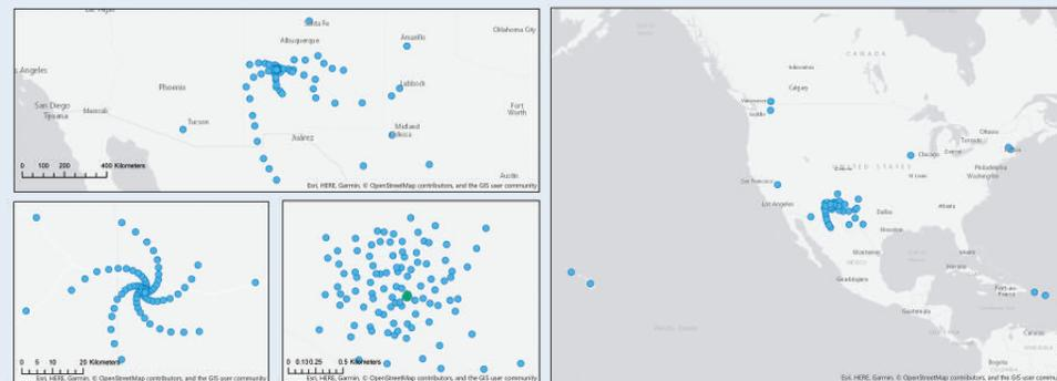
Main interferometric array composed of a compact core (bottom right; short baseline array antennas are shown in green), a five arm spiral spanning the Plains of San Agustin (bottom left) and a nearly 3-armed spiral that extends into TX, northern Mexico and AZ (top).
