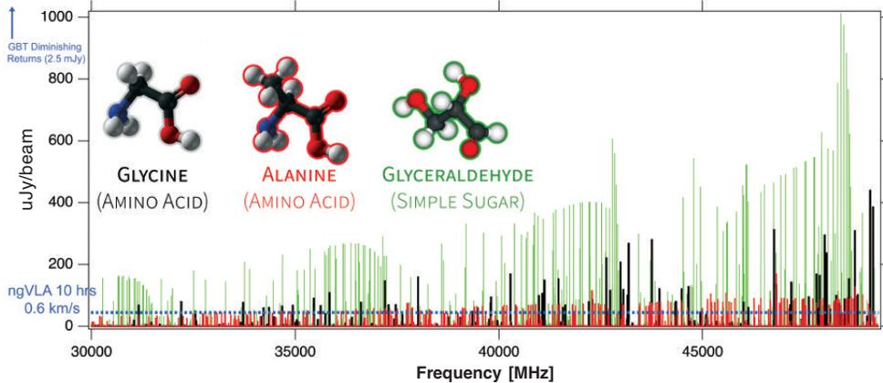
Simulations of three biogenic molecules in a typical hot core source, based on existing upper limits, assuming  $T = 80$  K,  $dV = 3$  km/s, and a 5" source. The ngVLA's sensitivity to detect these lines for the first time in a 10 hr integration is shown as a dashed blue line. For comparison, diminishing returns with GBT integrations start around 2.5 mJy; to detect any new molecules below that limit would require 100s to 1000s of hours.
