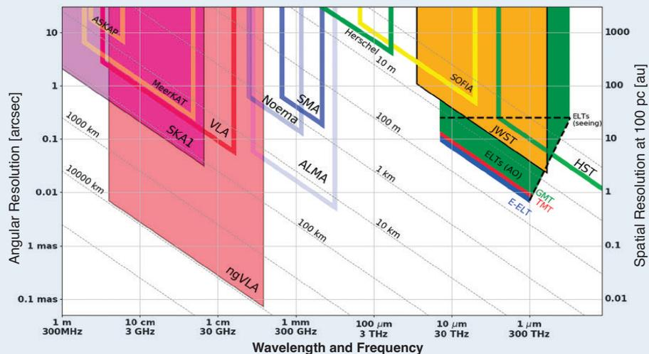
A comparison of achievable angular resolutions for a number of existing and expected facilities spanning the electromagnetic spectrum.
