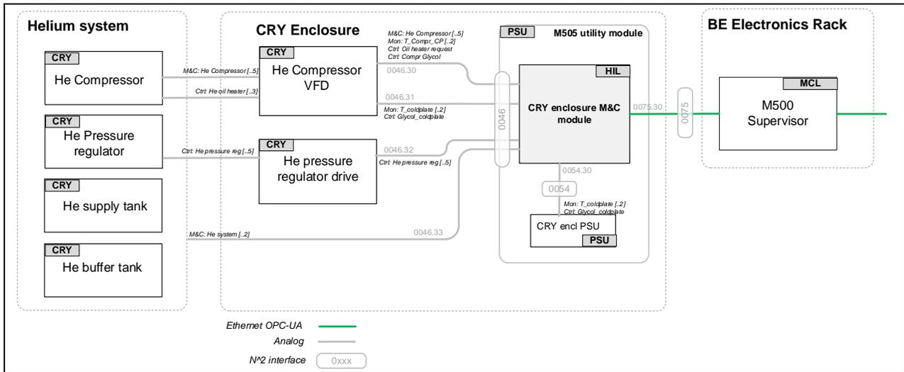
Figure 8: Cryogenics enclosure control and monitoring interfaces
