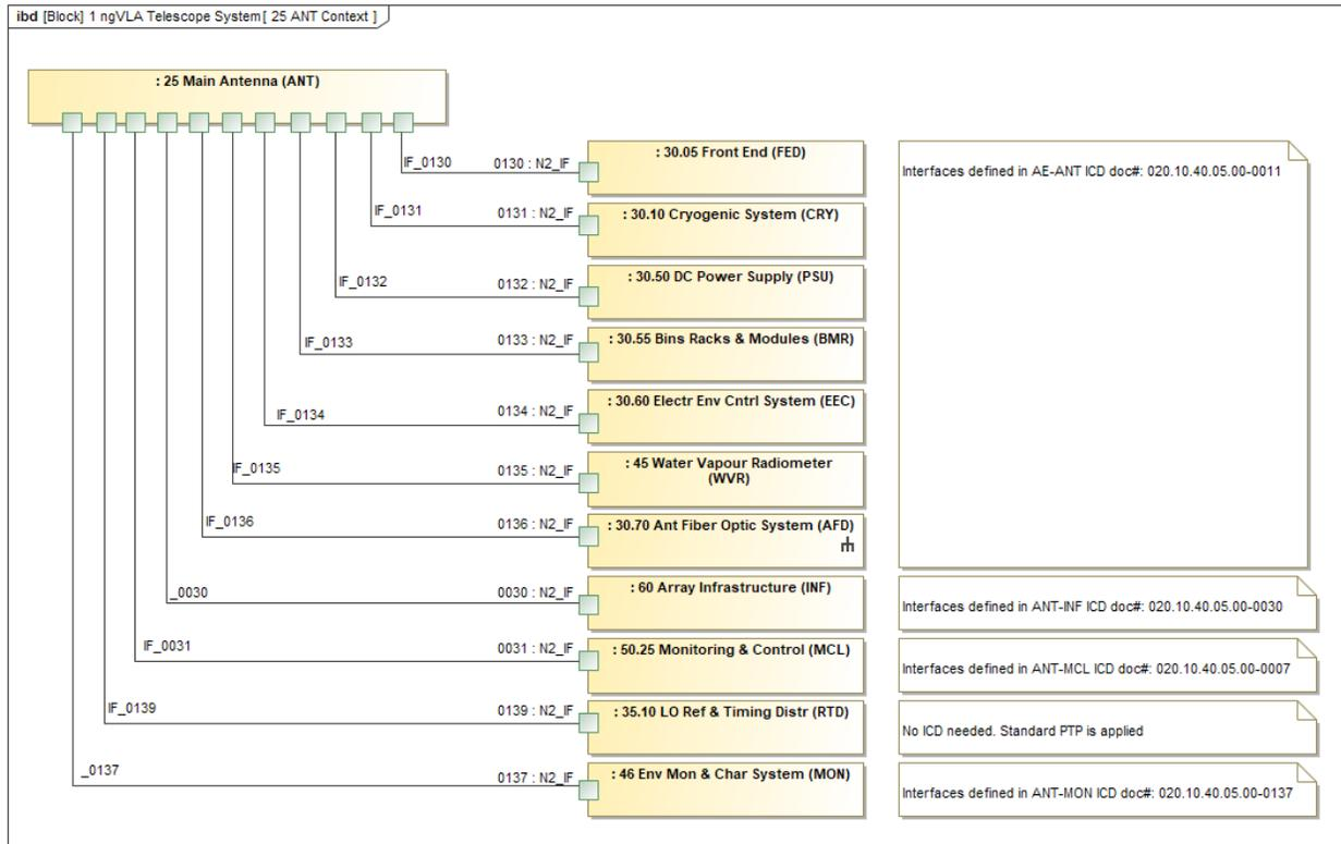
Figure 12: Main Antenna external interfaces
