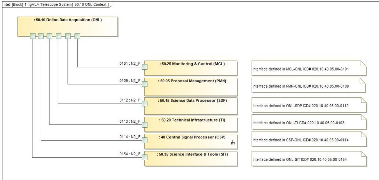
**Figure 49: Context diagram for the ONL sub-element, showing the interfaces between this sub-element and other system elements.**
