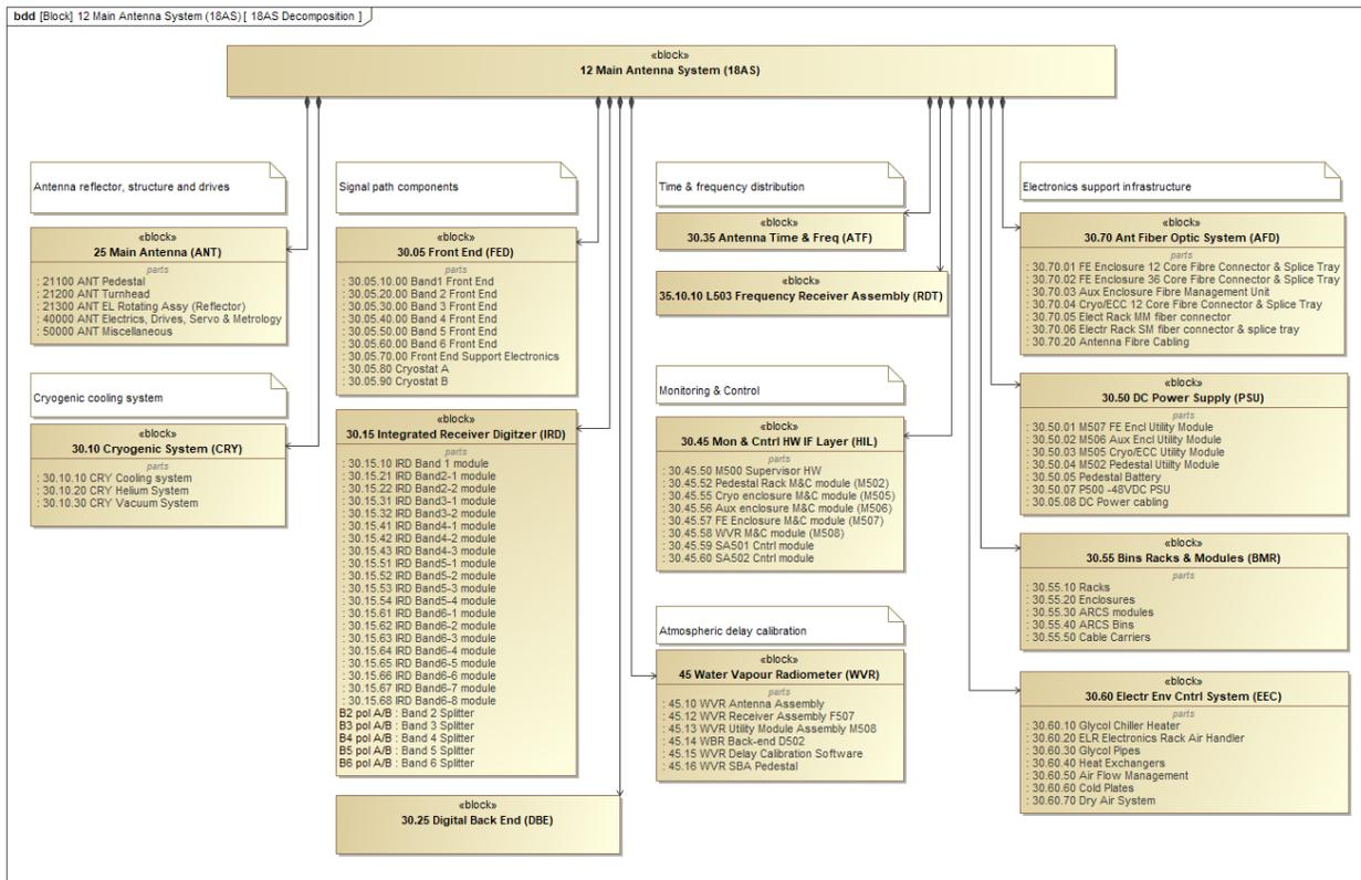
Figure 4: Product Breakdown Structure of Main Antenna System
