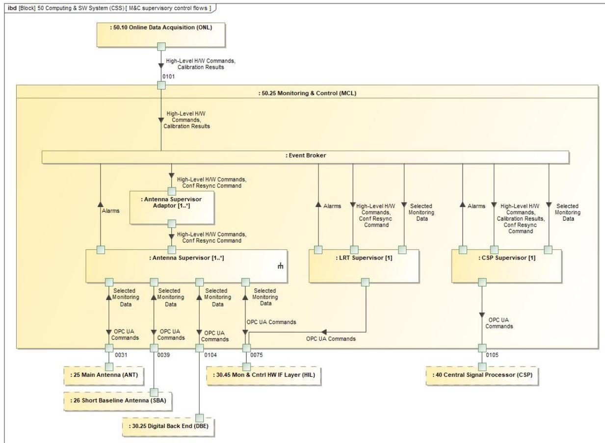
Figure 53: Monitoring and control supervisory flows.
