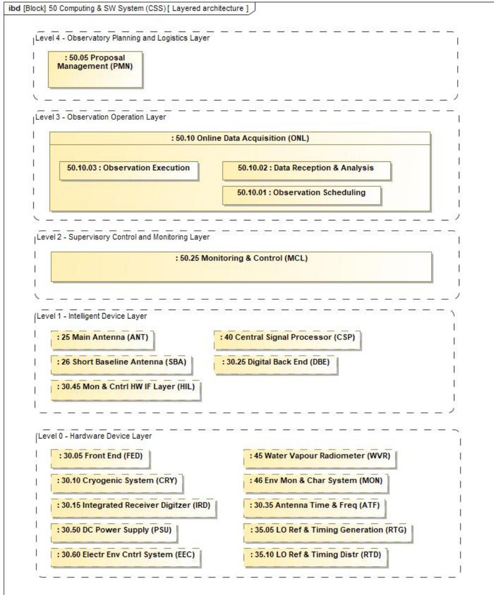
Figure 42: Monitoring and control conceptual layered architecture.
