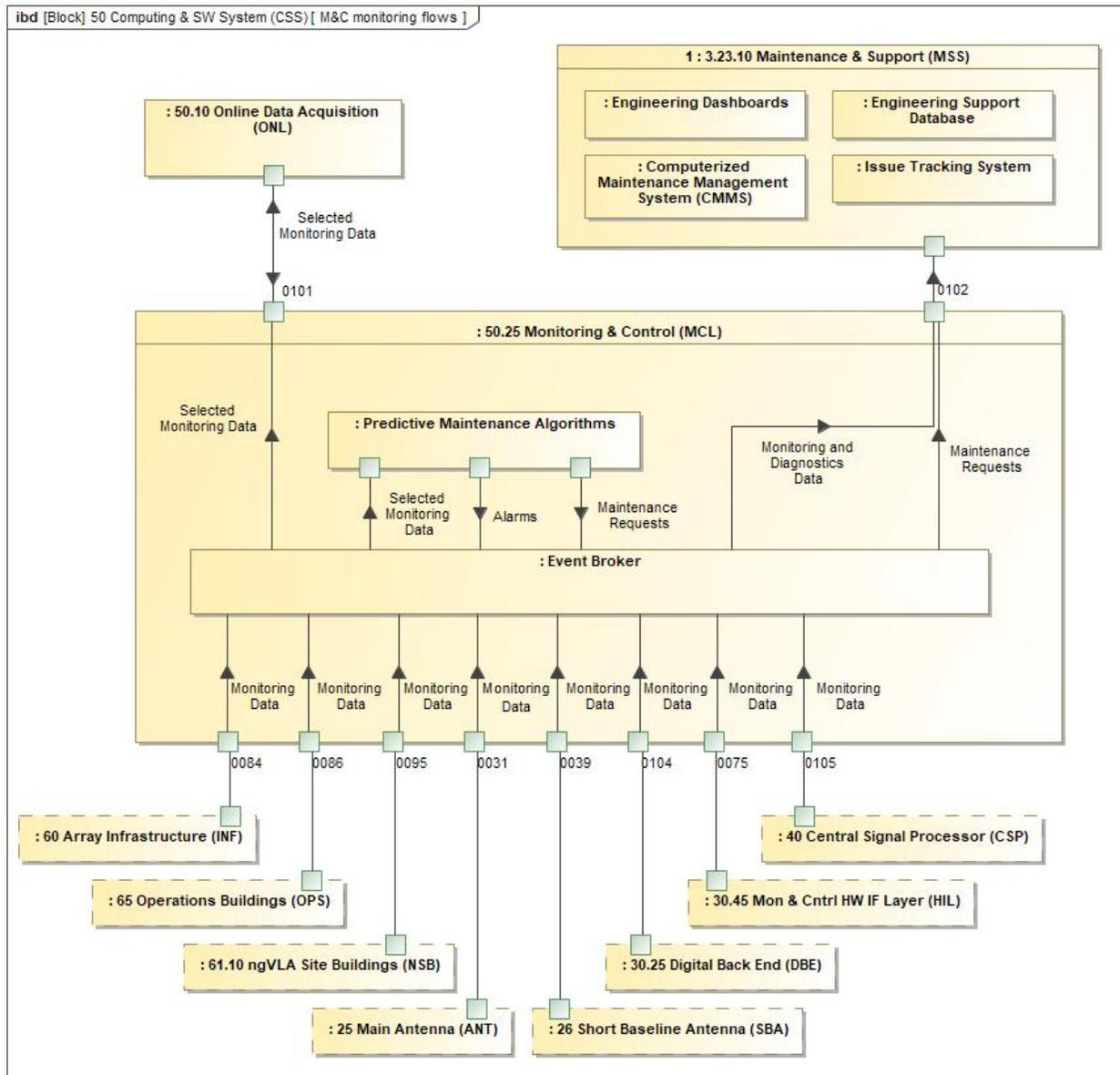
Figure 54: Main monitoring data flows in the MCL system.
