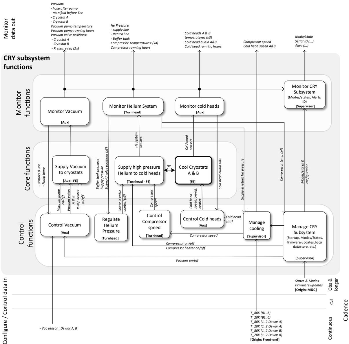
Figure 92: Cryogenic cooling function
