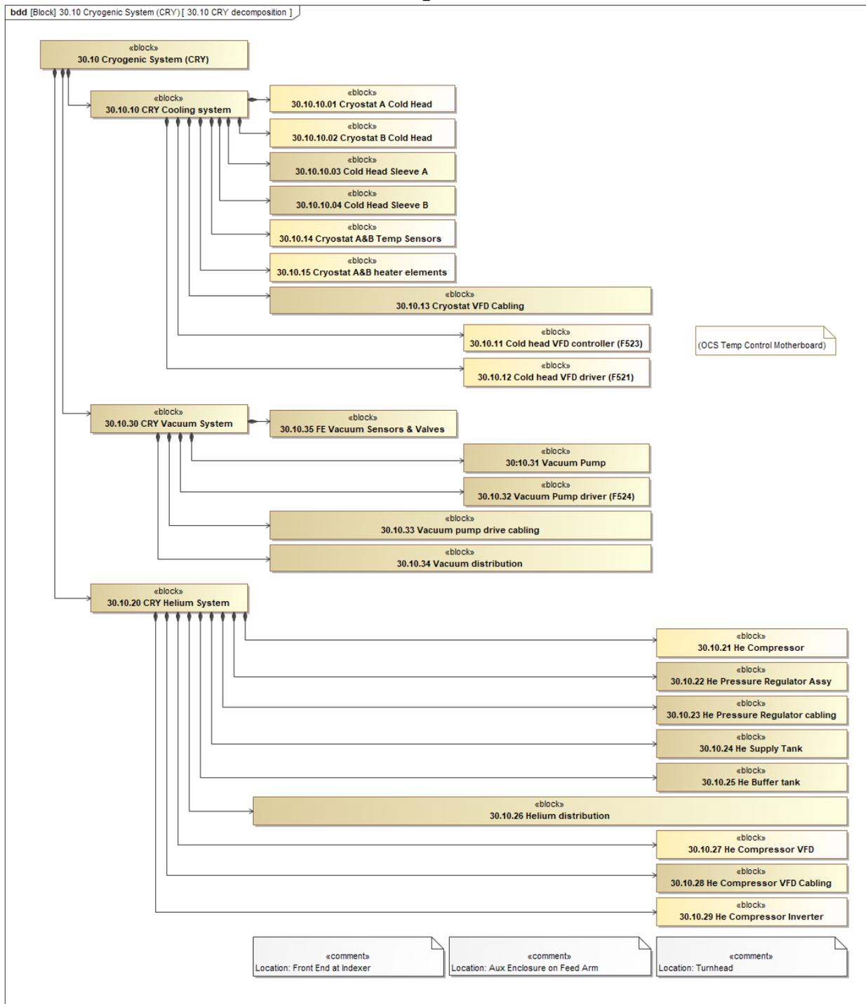
Figure 16: Cryogenic Subsystem decomposition and location
