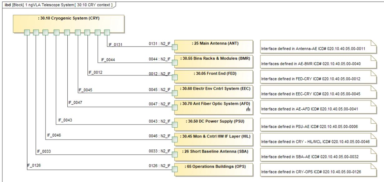
Figure 17: Cryogenic Subsystem external interfaces
