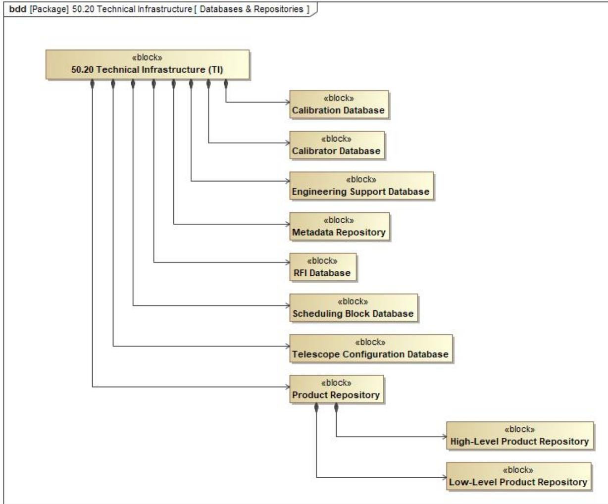
Figure 65: TI decomposition for databases and file repositories.
