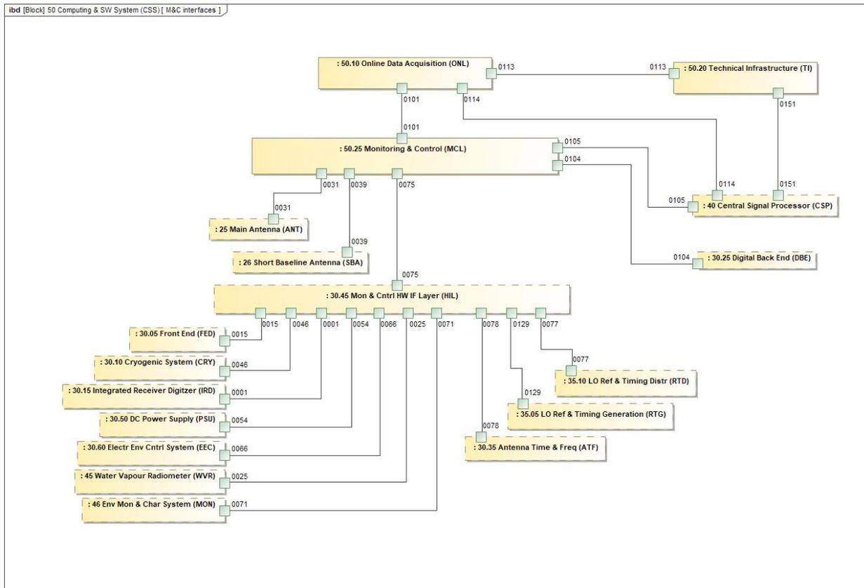
Figure 44: CSS monitoring & control interfaces.
