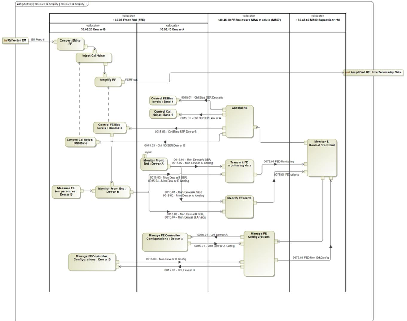
Figure I 12: Functional model for Front End M&C
