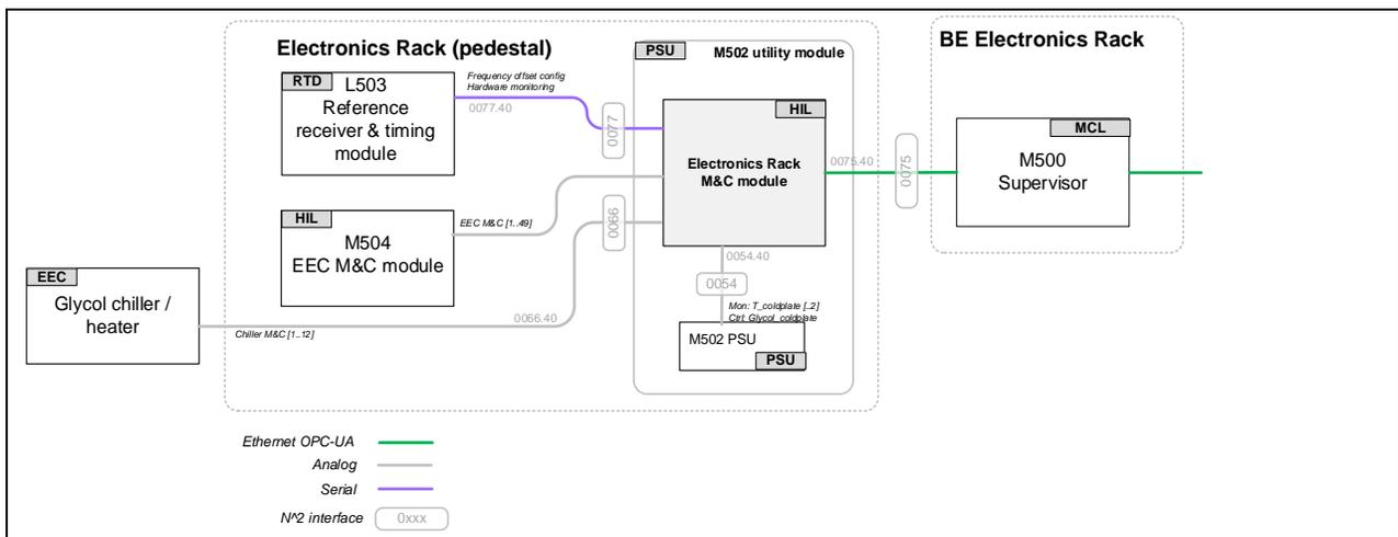
Figure 10: Electronics Rack control and monitoring interfaces
