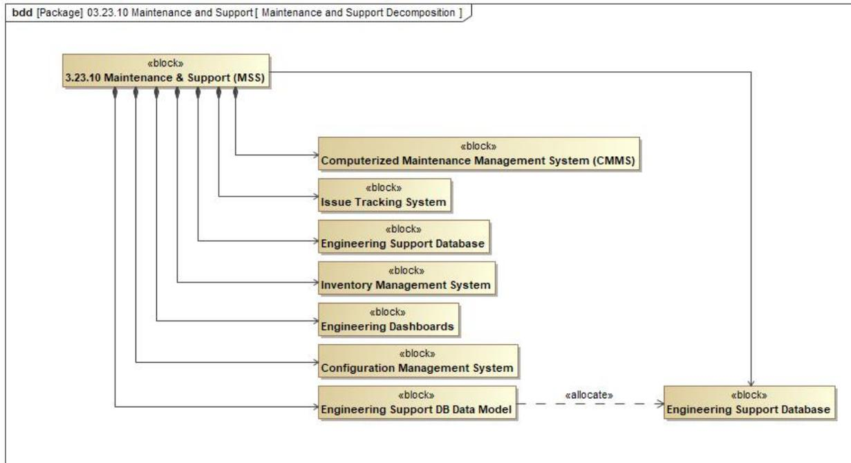
Figure 56: High-level decomposition of the Maintenance and Support Subsystem.
