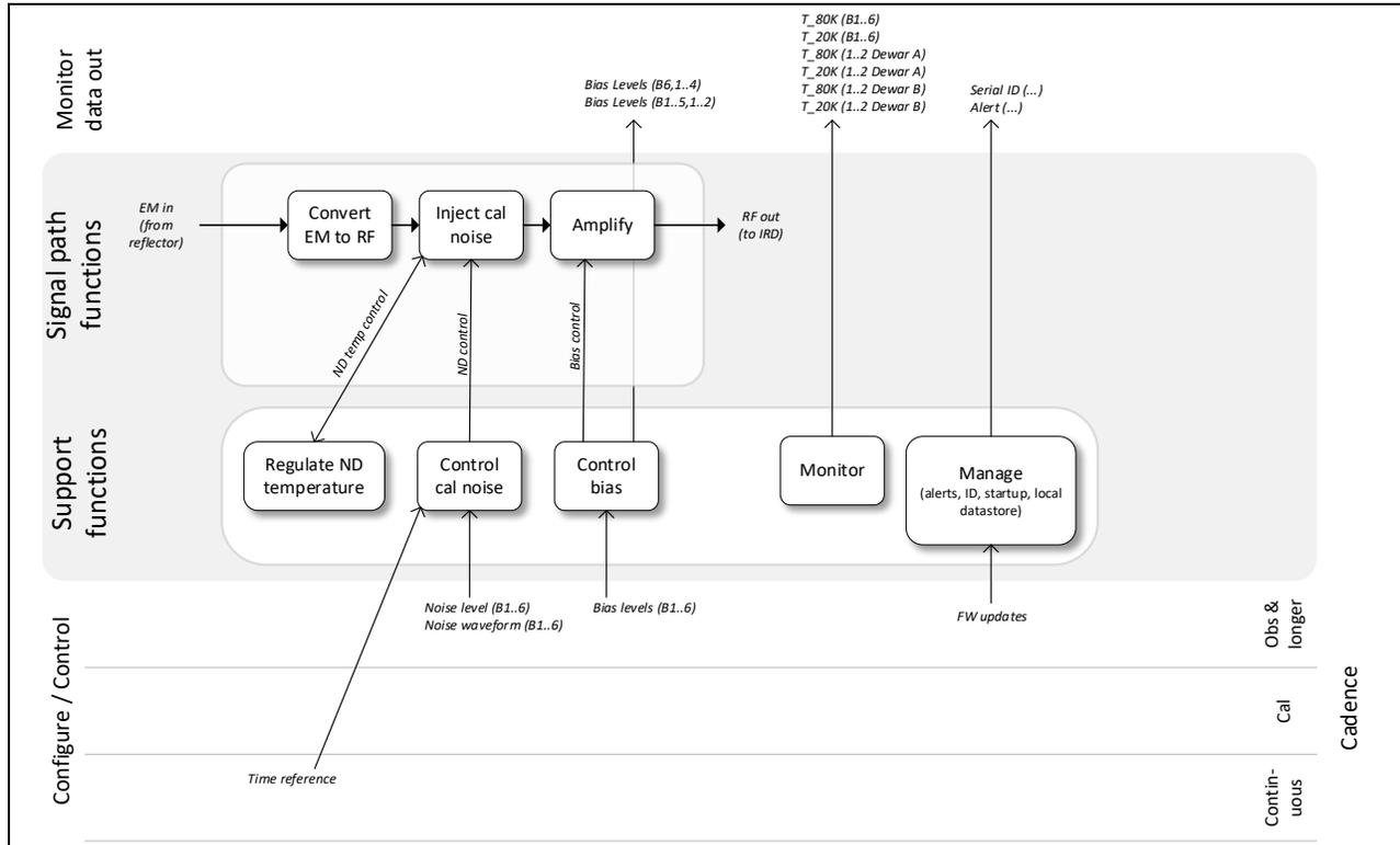
**Figure 86: Receive and amplify functions**
