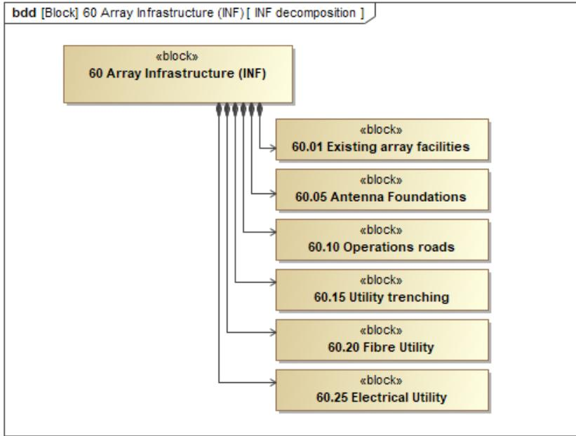
Figure 35. Array Infrastructure Subsystem Decomposition
