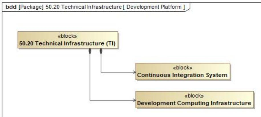
Figure 66: TI decomposition for the development platform elements.
