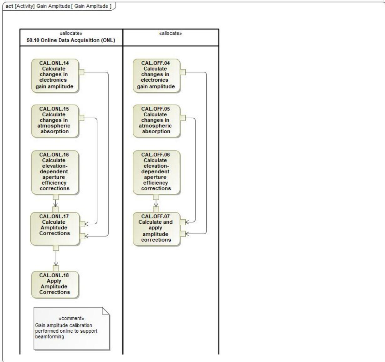
Figure I04: Gain amplitude calibration activities.
