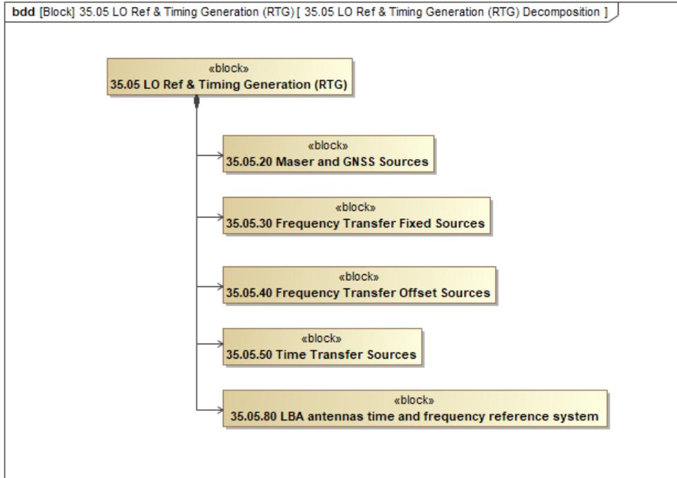
Figure 77: RTG decomposition
