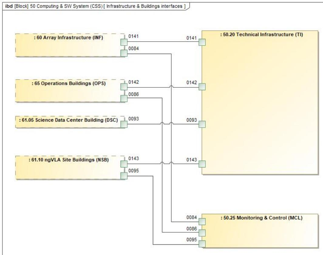
**Figure 45: Interfaces between Infrastructure and Buildings and CSS elements.**
