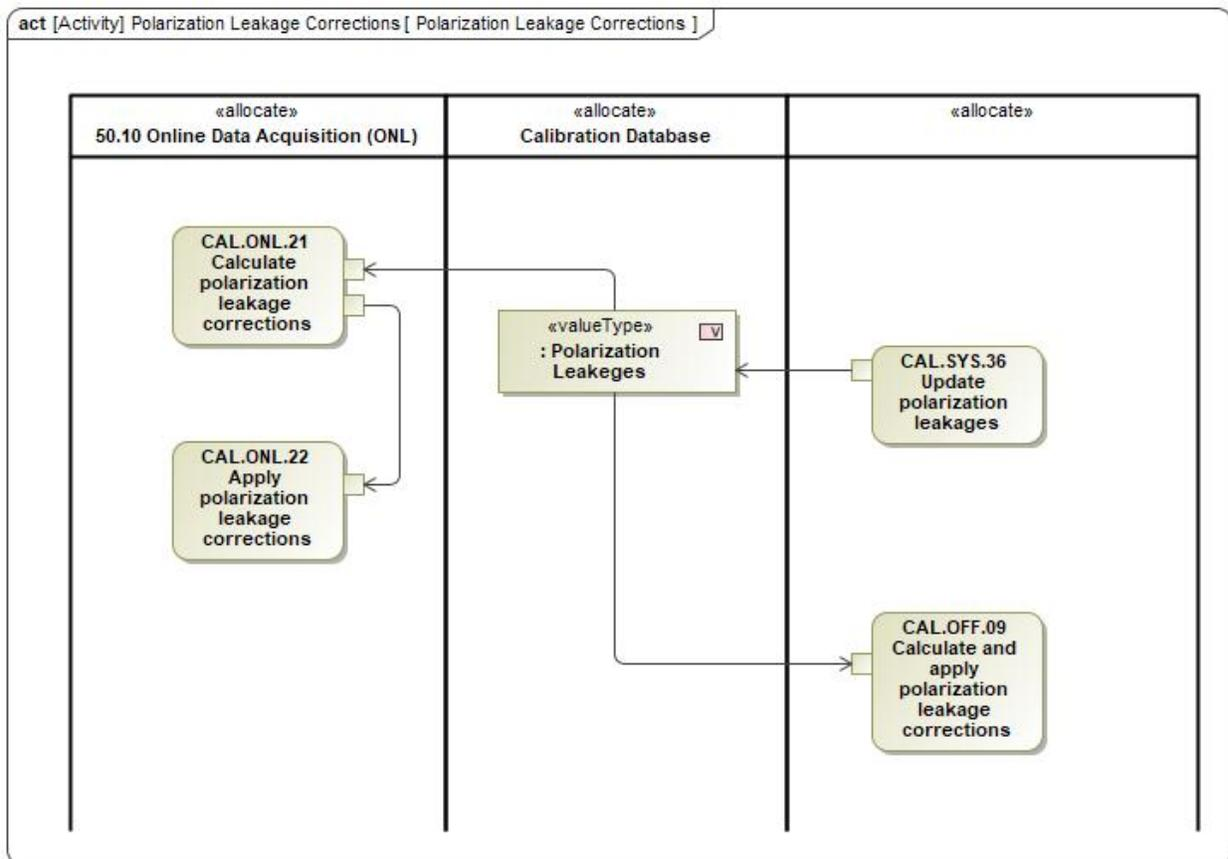
Figure 107: Polarization leakage calibration activities.
