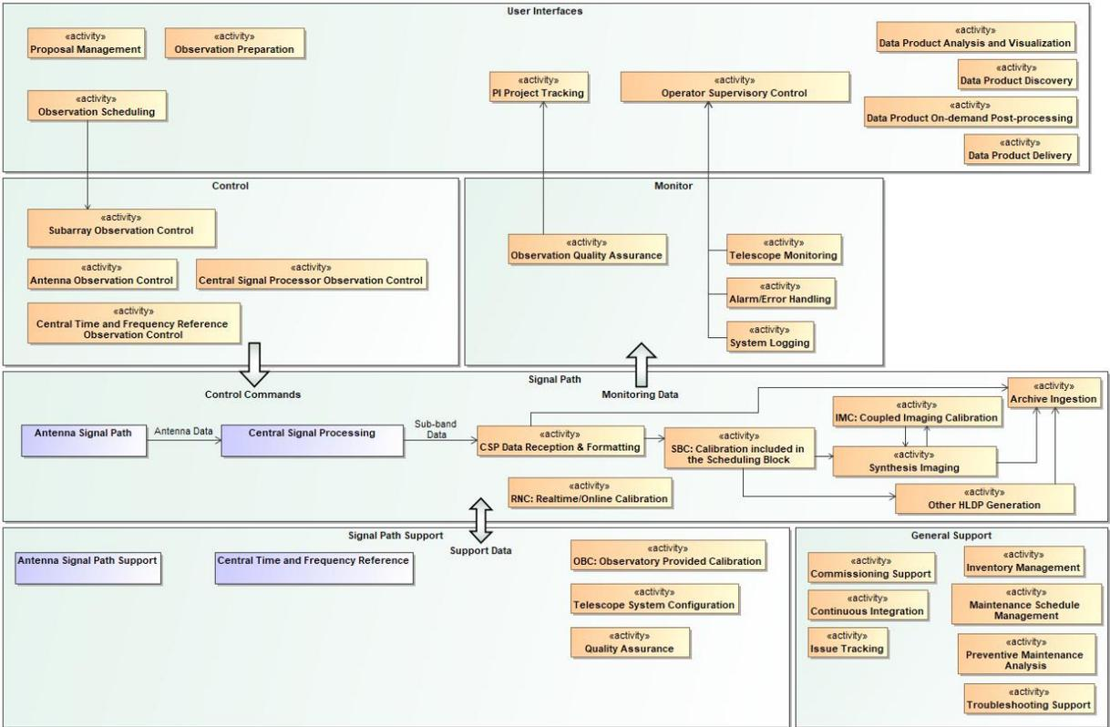
**Figure 83: System Functions**
