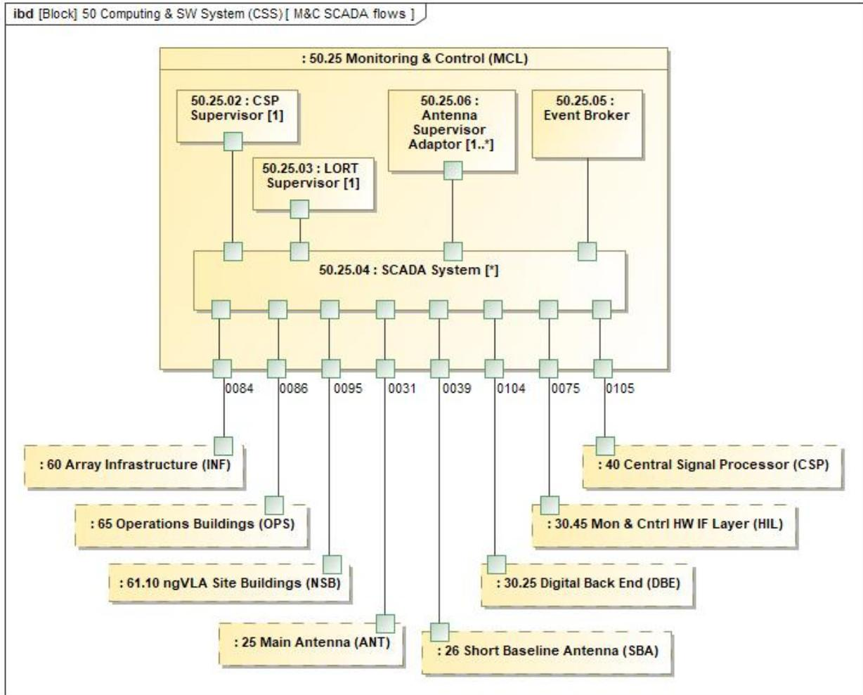
**Figure 55: SCADA-related connections and data-flows.**
