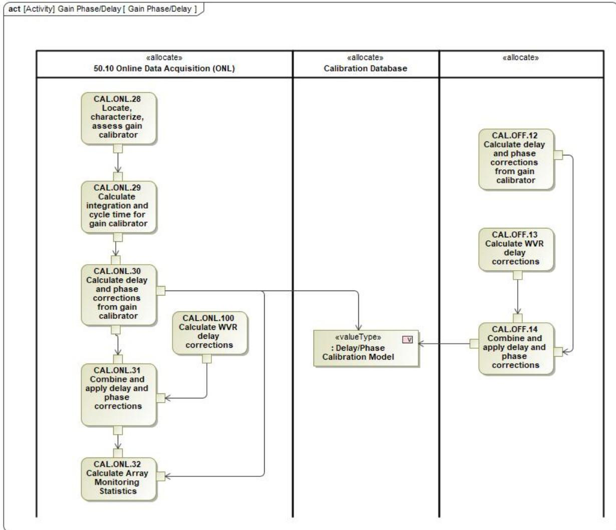
Figure 105: Gain phase and delay calibration activities.
