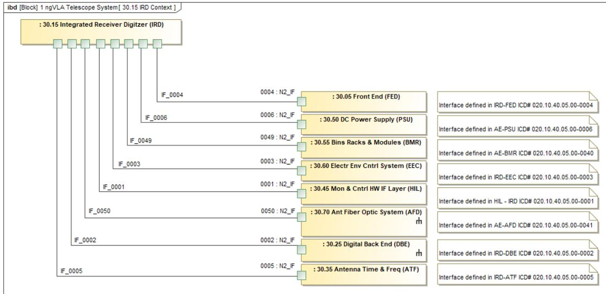
Figure I9: IRD external interfaces
