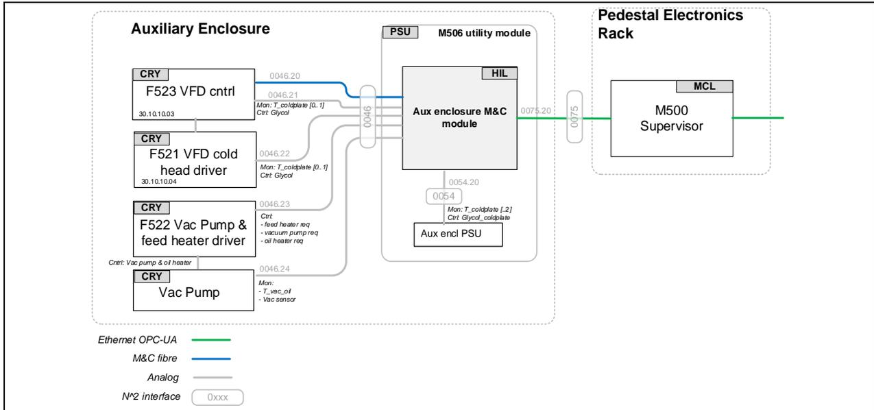
Figure 7: Auxiliary enclosure control and monitoring interfaces
