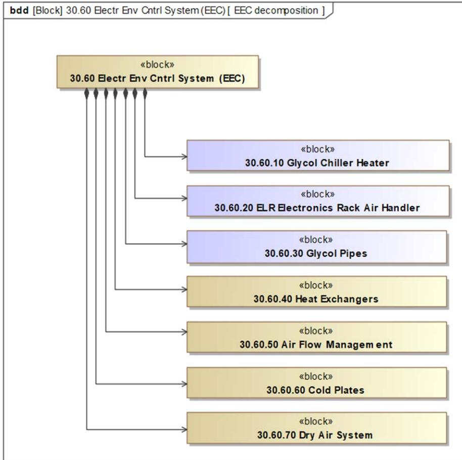
**Figure 29: EEC product breakdown structure**
