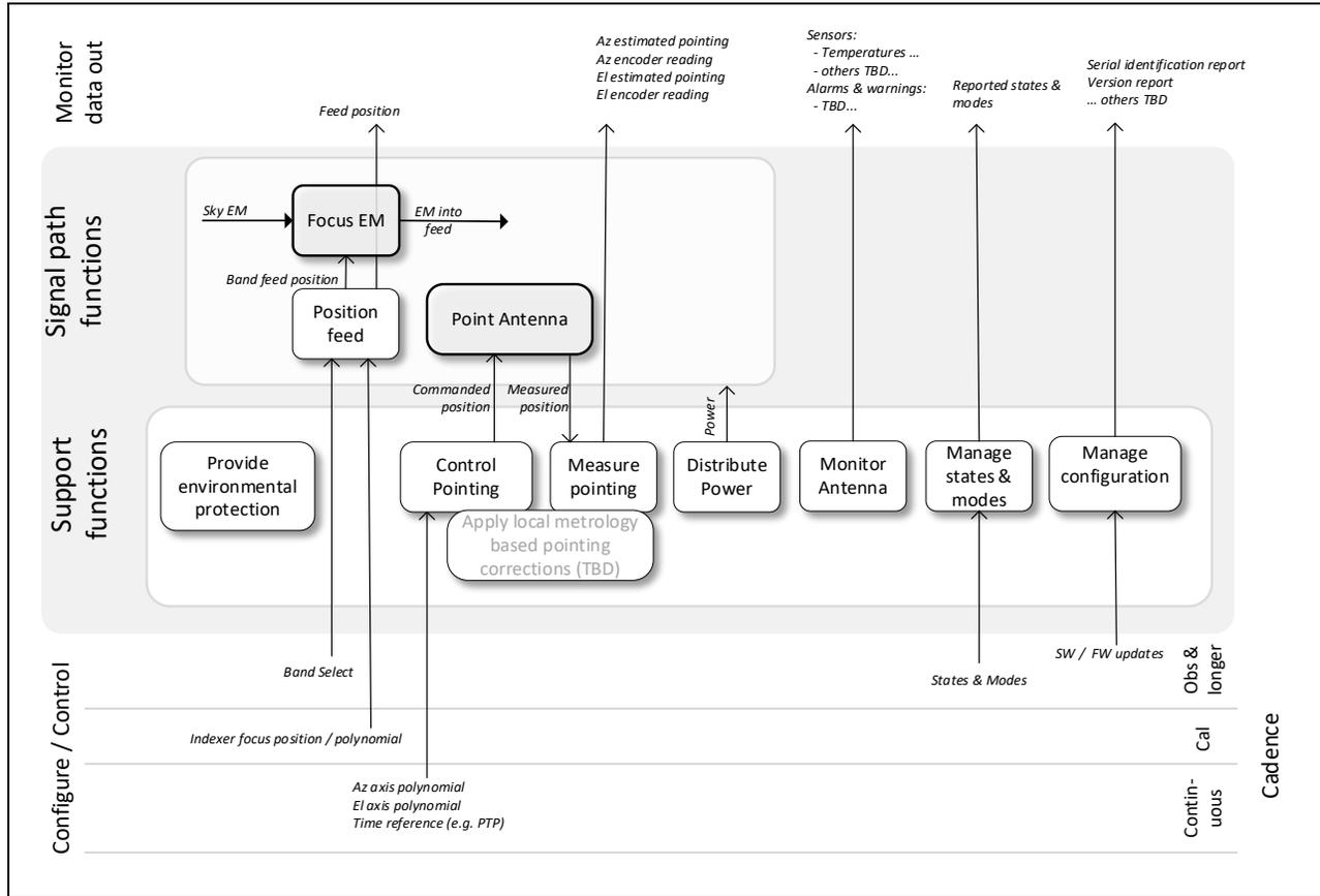
Figure 85: Focus and point functions
