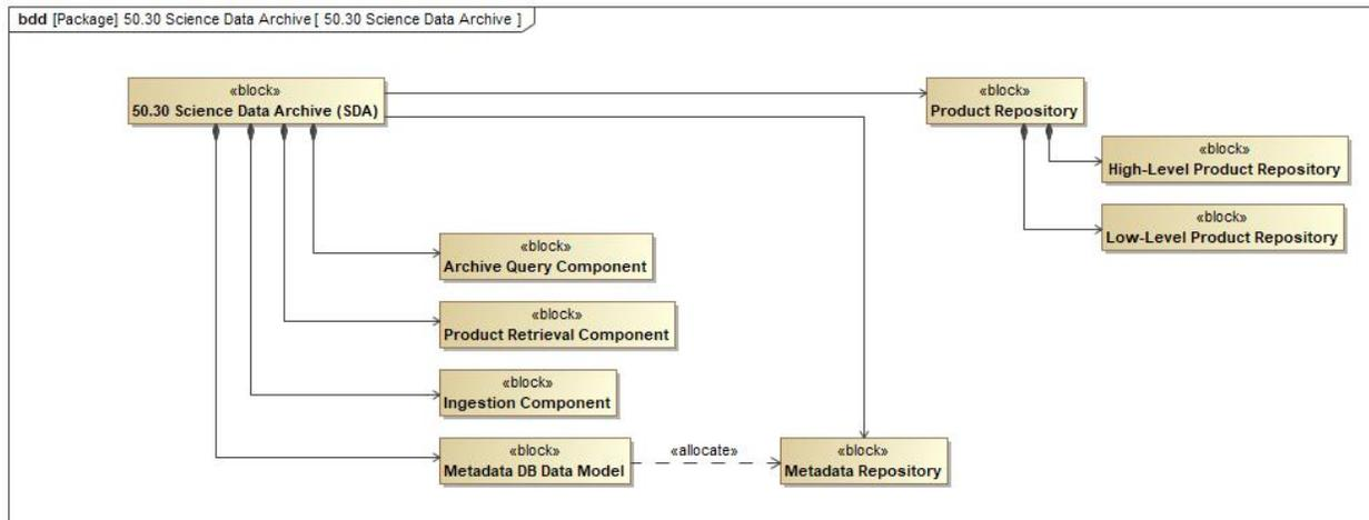
Figure 60: SDA decomposition diagram.
