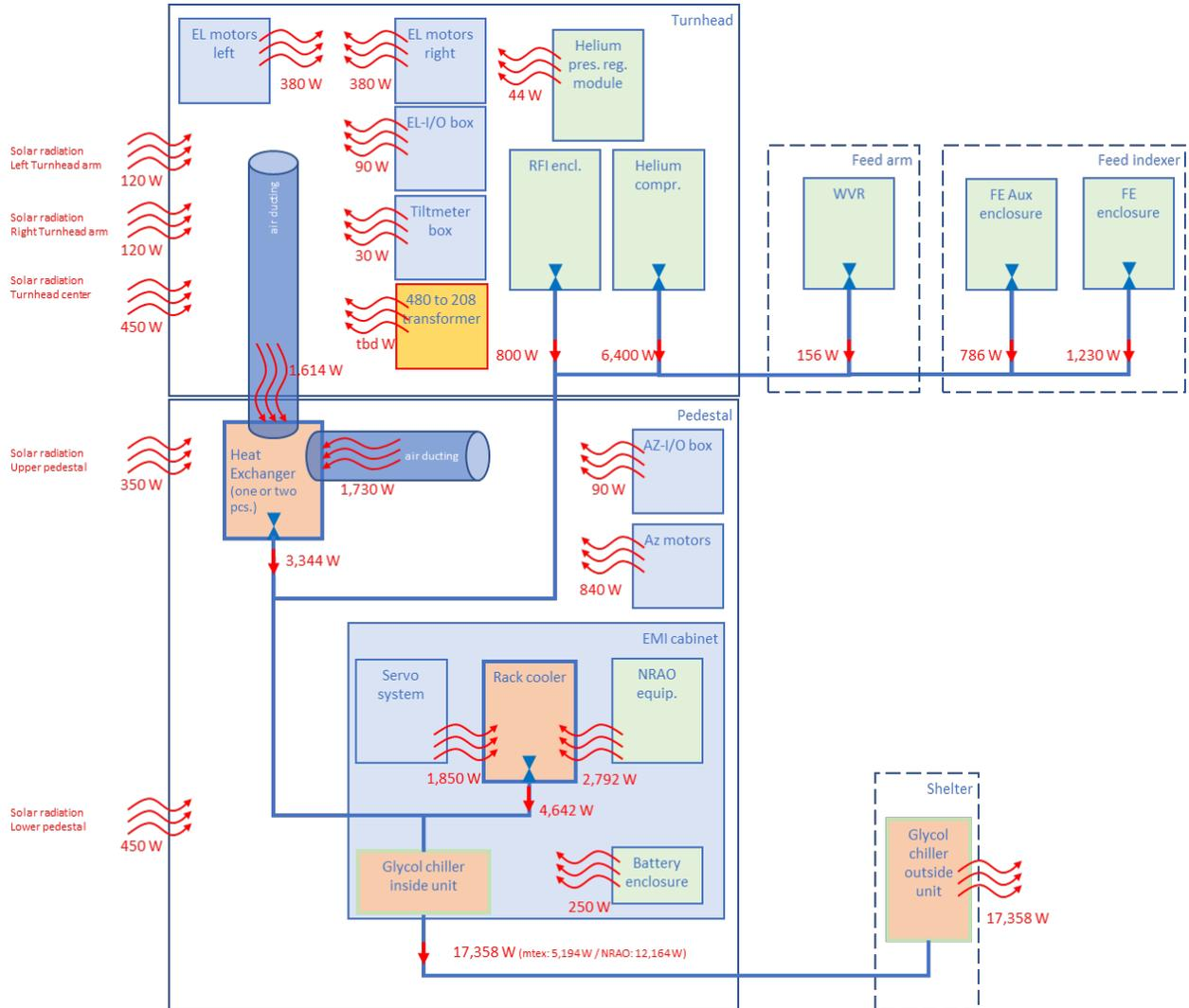
**Figure 28: Overview of the Antenna Environmental Control System**
