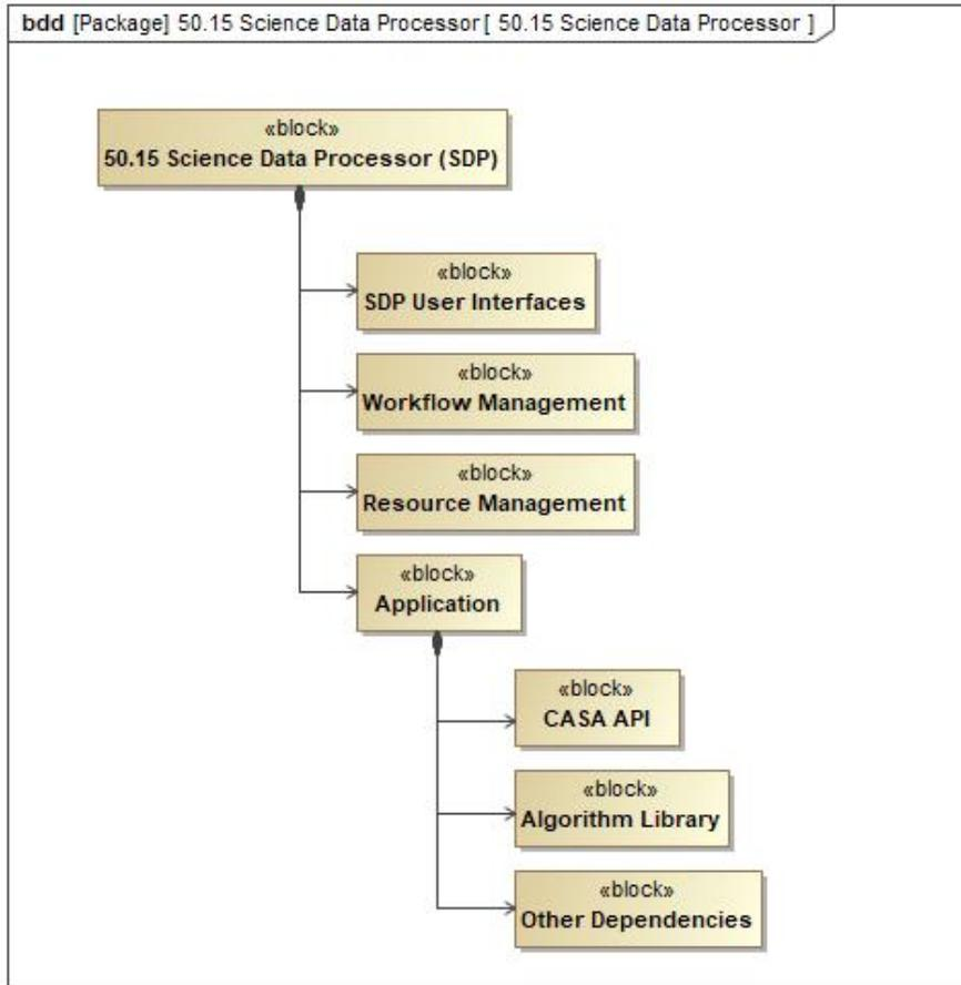
**Figure 58: SDP system decomposition.**
