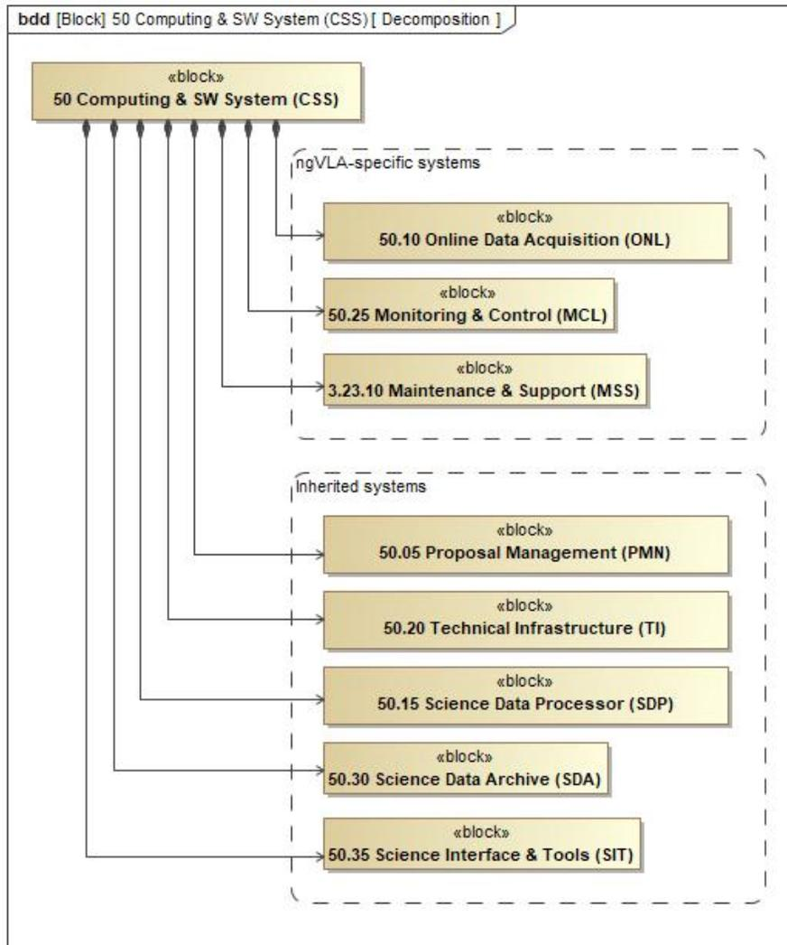
**Figure 4I: Decomposition diagram for the Computing and Software (SW) Subsystem.**
