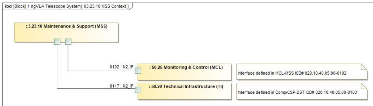
**Figure 57: Context diagram of the Maintenance and Support Subsystem, showing the interfaces between this subsystem and other system sub-elements.**
