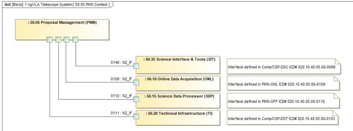
**Figure 47: Context diagram for the Proposal Management System, showing the interfaces between this system and other system elements.**
