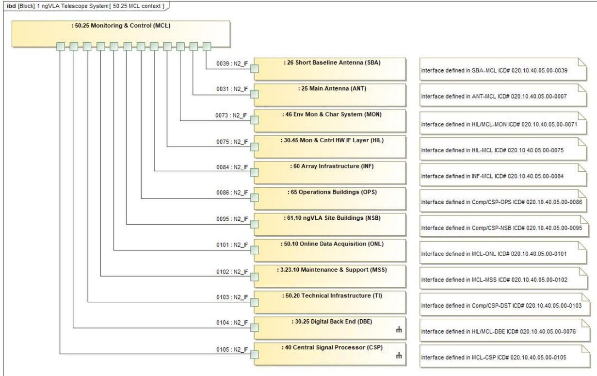
**Figure 52: Context diagram for the MCL system, showing the external interfaces between this system and other system elements.**
