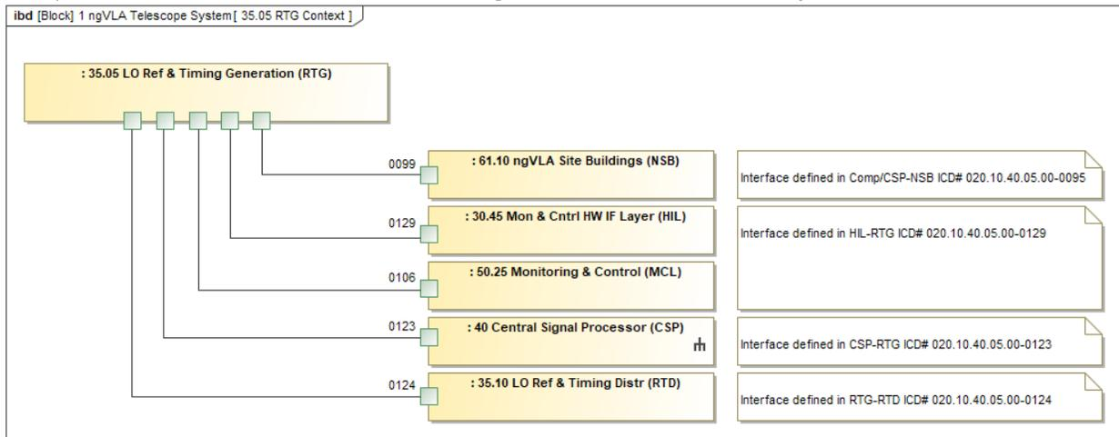
Figure 78: RTG external interfaces
