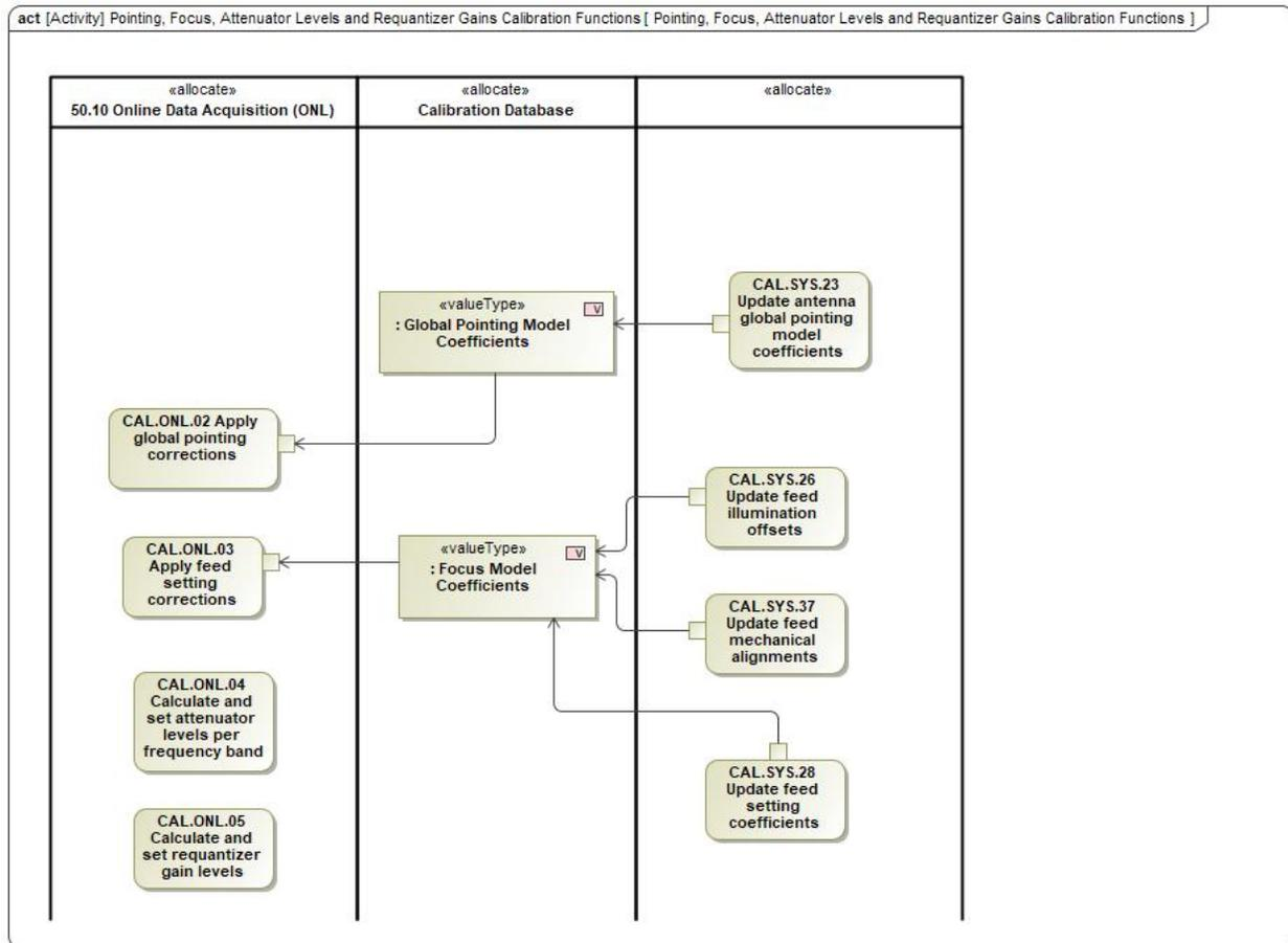
Figure I01: Pointing, focus and attenuator level and requantizer gains calibration activities.
