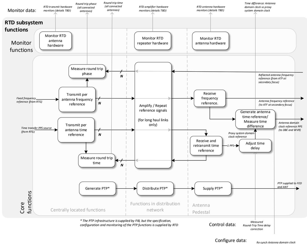
**Figure 97: Reference signal distribution functions**
