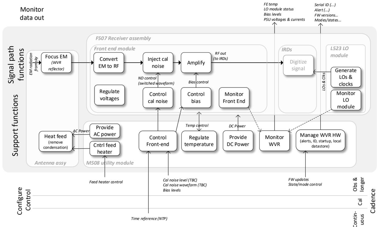
Figure 94: Receive and amplify WVR signal functions
